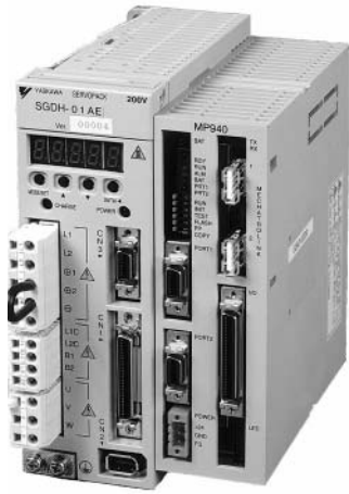
Integrated Sigma II servo amp with MP940 controller
