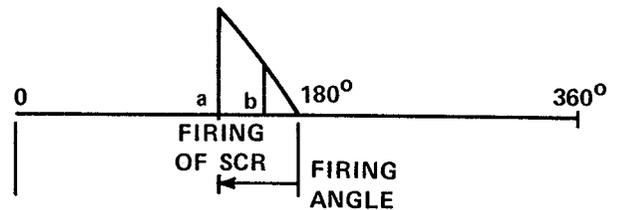
Figure 3-2. Resultant Armature Voltage, Phase A Positive with Respect to Phase C
