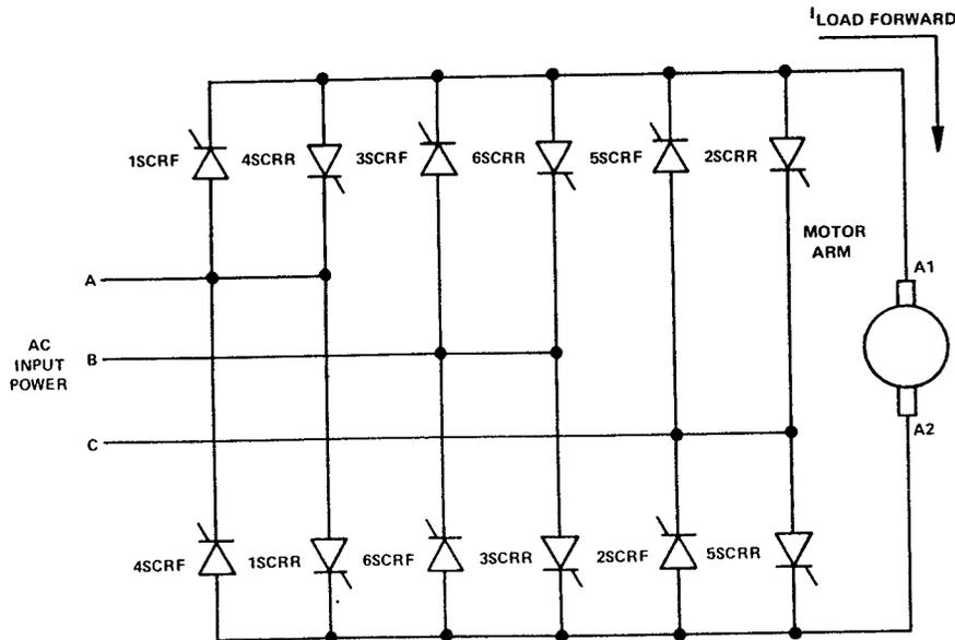
Figure 3-5. Simplified 12SCR Power Circuit
