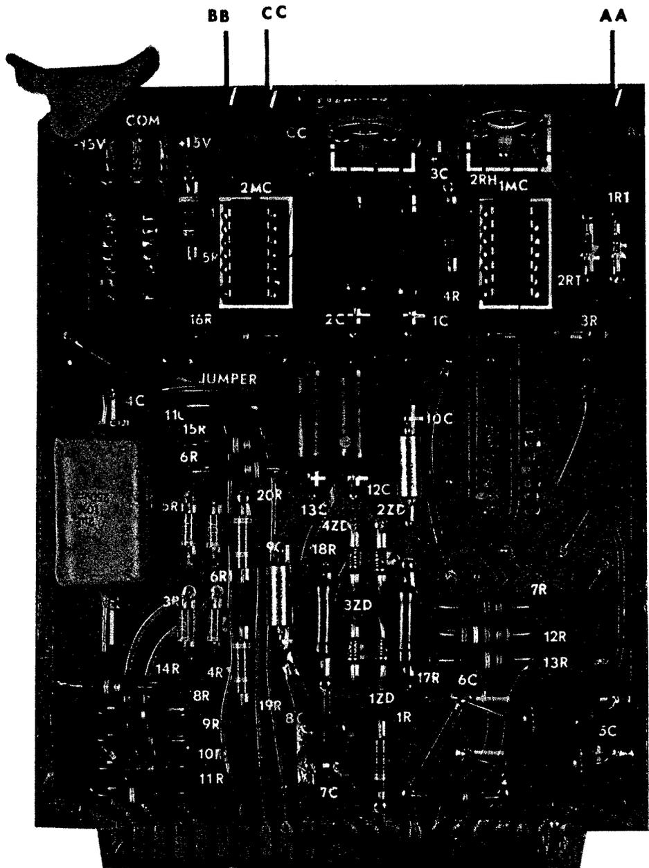
Figure 6-5. Reference and Actuator PCB Test Point Location
