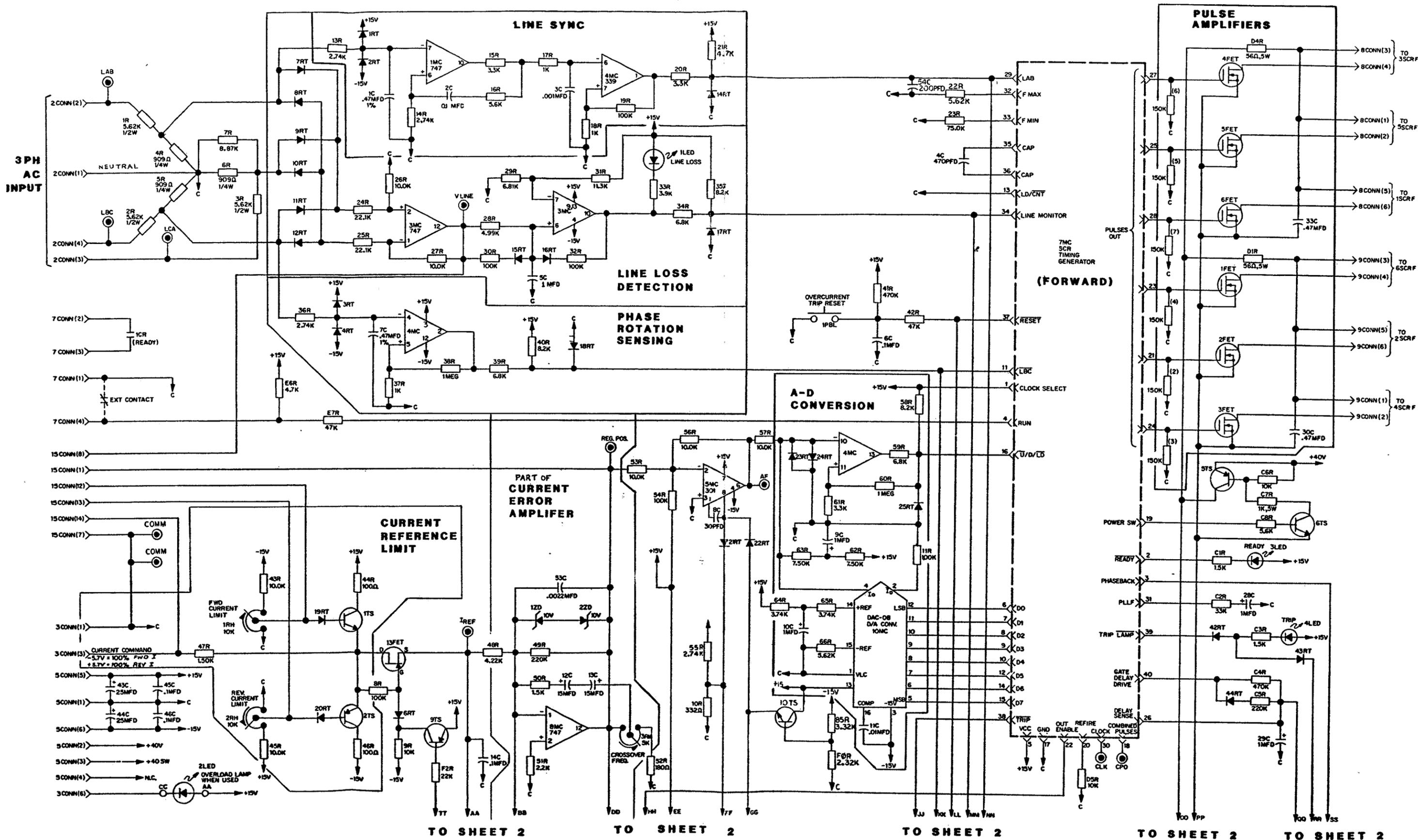
Figure 6-2. Main PCB Schematic Diagram Sheet 1
