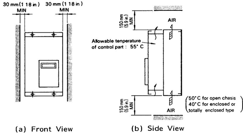
Fig. 2 Clearance Requirements for Proper Cooling and Maintenance
