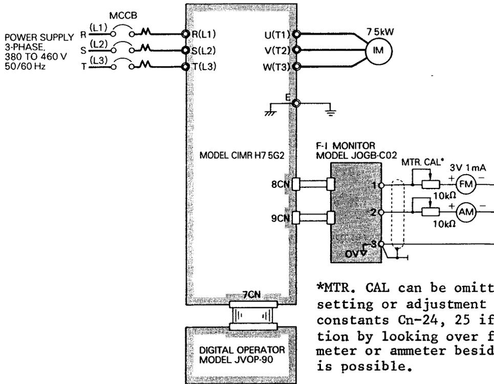
\*MTR. CAL can be omitted by setting or adjustment of control constants Cn-24, 25 if calibration by looking over frequency meter or ammeter beside unit is possible.
