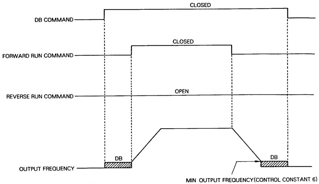
Fig. 15 Time Chart of DC Dynamic Braking
