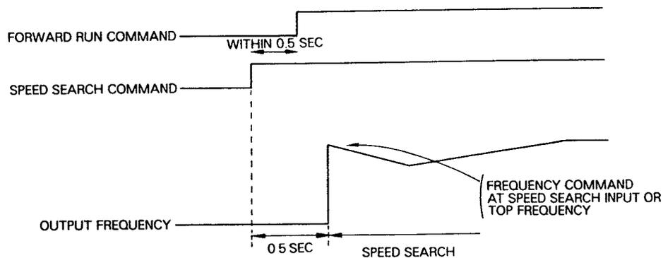
Fig. 13 Time chart at Speed search command Input
