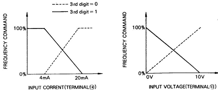
Fig. 10 Input method of Master Frequency Command
