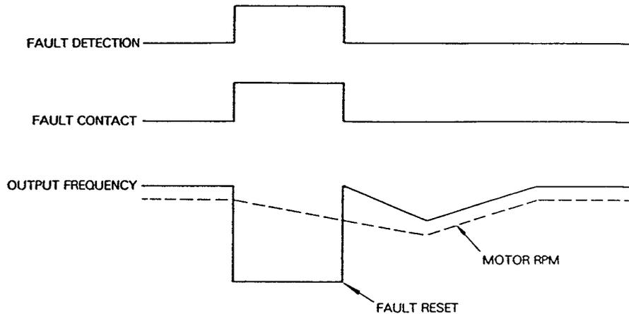
Fig. 21 Time Chart of Retry Operation at fault
