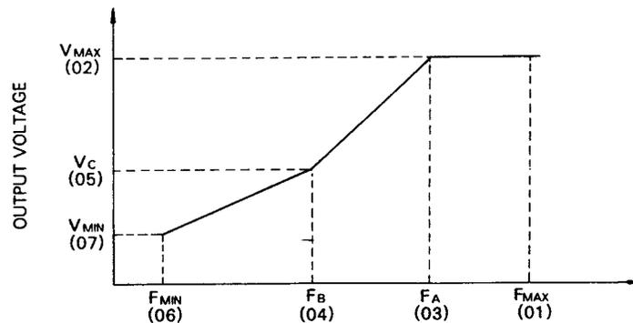
Fig. 16 V/f Characteristics by Control Constants 1 to 7
