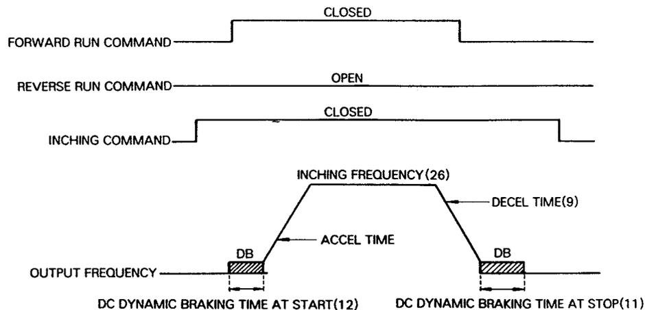
Fig. 12 Time chart at Forward and Inching Operations
