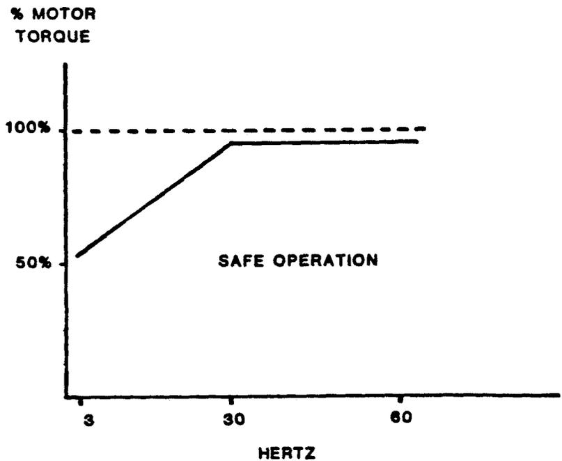
Fixed speed machinery may not run properly at available speed ranges. Operation above 60 HZ may damage bearings or rotating parts. Slow speeds may provide insufficient lubrication on oil filled gear boxes or speed reducers. Manufacturer specifications may need to be consulted.
