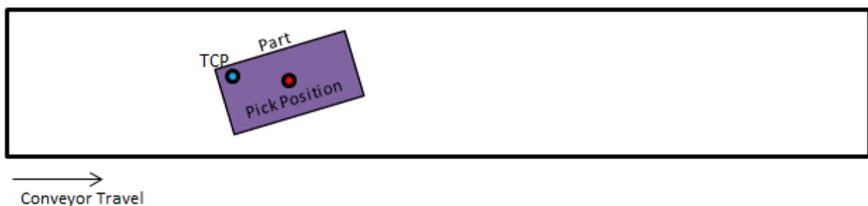
FIGURE 4 TCP IS COMMANDED TO HOVER POSITION OVER PART WHILE SYCNING INTO CONVEYOR
