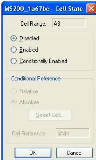
Figure 8: Enable/Disable a Spreadsheet Cell with the Cell State Dialog.
