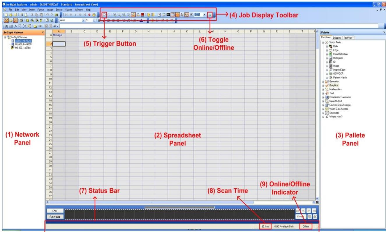
Figure 4: New Job in Spreadsheet Mode of In-Sight Explorer.
