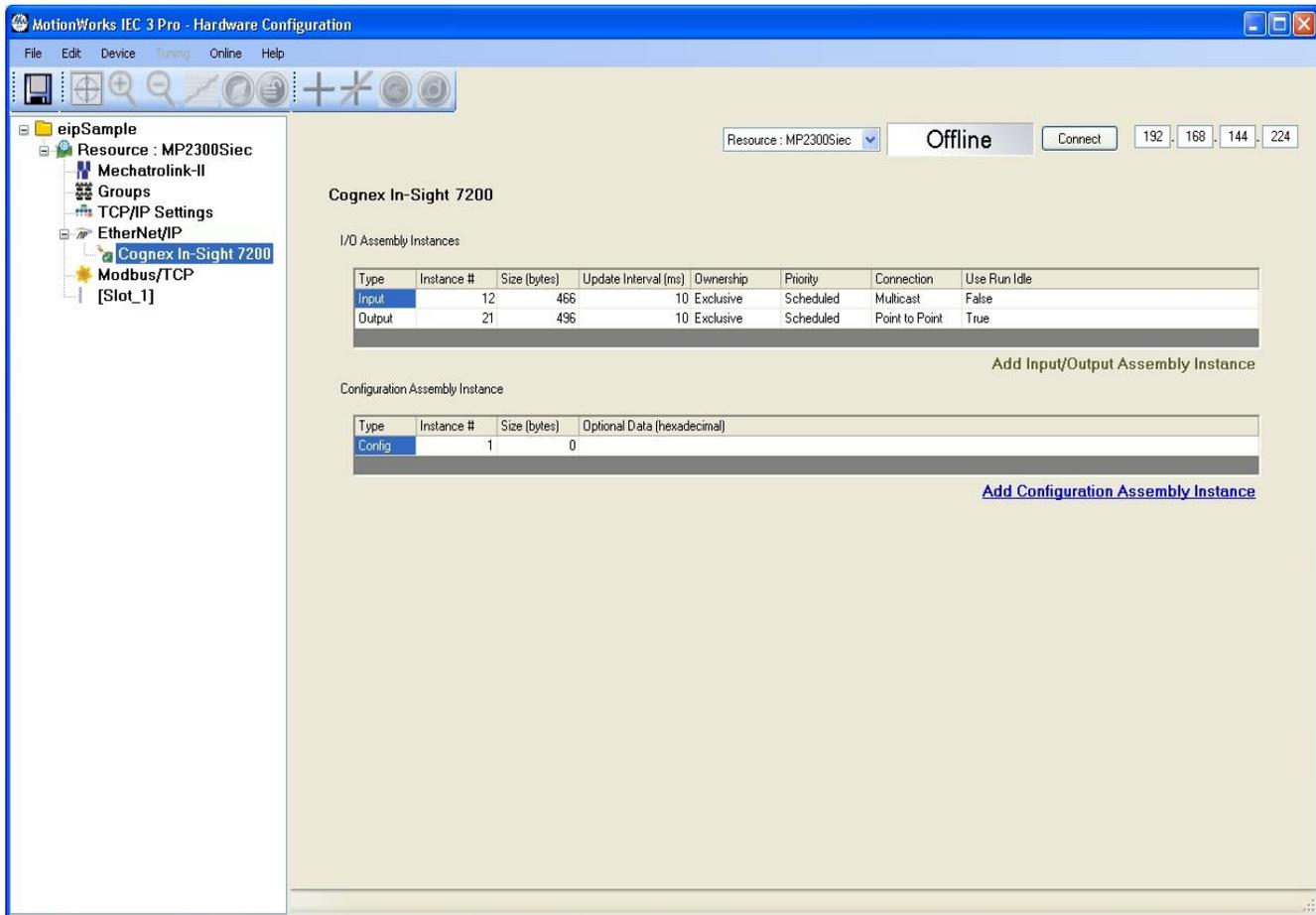
Figure 12: Specify I/O and Configuration Assembly Instances for Cognex System in MotionWorks IEC Hardware Configuration Tool.
