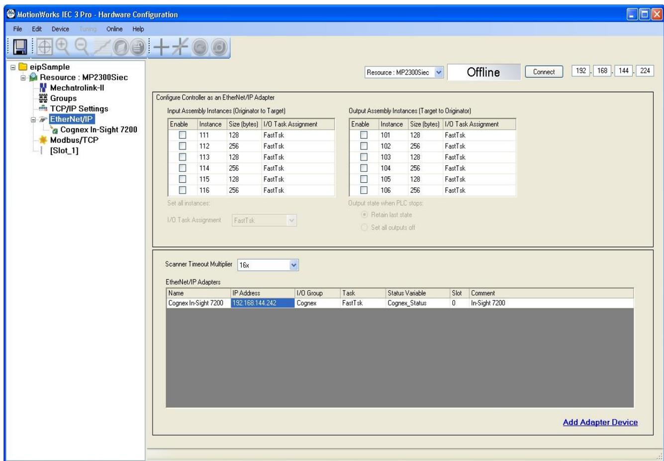
Figure 11: Add Ethernet/IP Adapter Device for Cognex System in MotionWorks IEC Hardware Configuration Tool.
