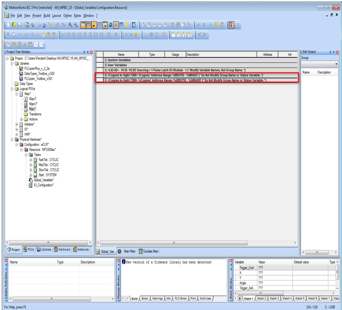
Figure 13: Input and Output Ethernet I/P Groups in Global Variable Table (See AN\_MPIEC\_15.zwt in AN.MPIEC.15.zip).
