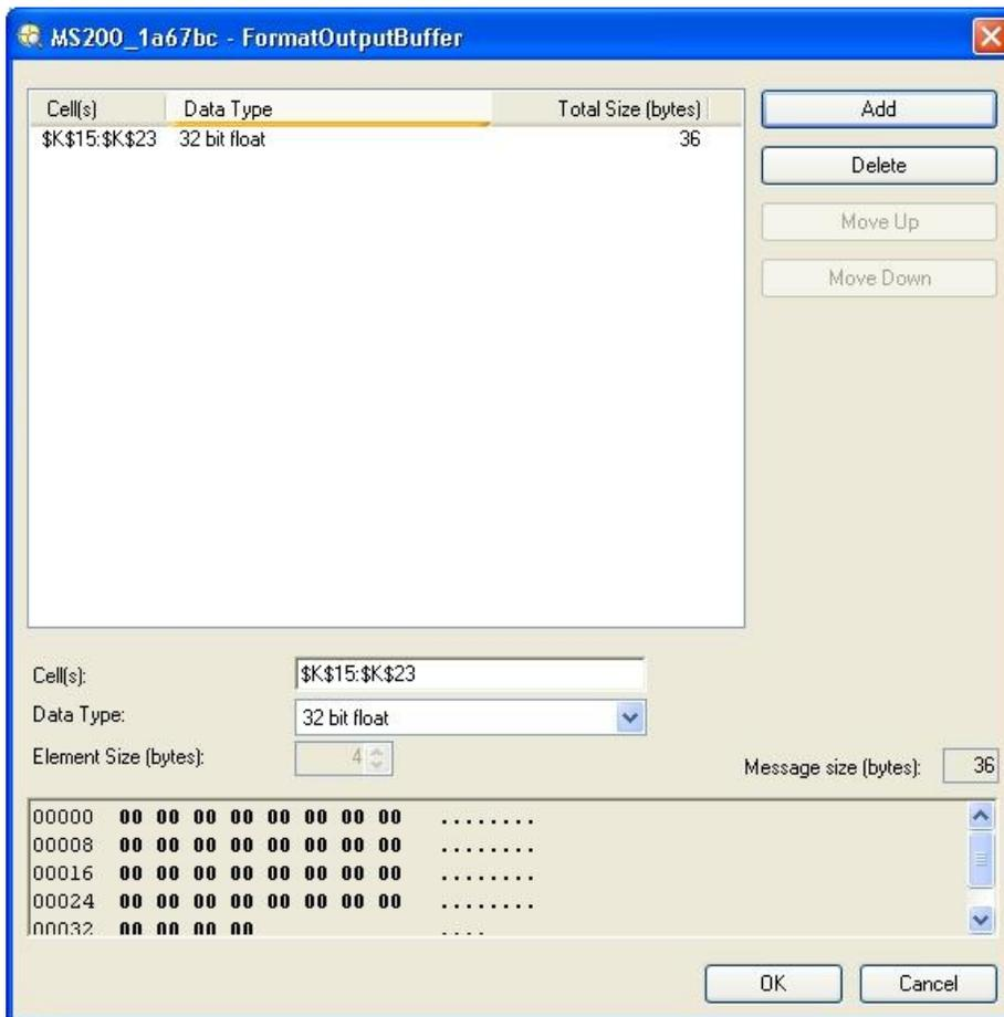
Figure 10: Add the value of the X coordinates, cells K15:K23 in Figure 6, to this Output Buffer
