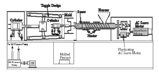
The injection molding is a cyclical process. Cycle times may range from 10 to 100 seconds and are controlled by the cooling time of the melted plastic. The melted plastic comes from hard plastic pellets that are fed into the hopper of the injection-molding machine. The pellets or plastic powder is melted inside the machine and then forced into the mold thru a nozzle (like a syringe) by a long screw within a heated cylinder.
