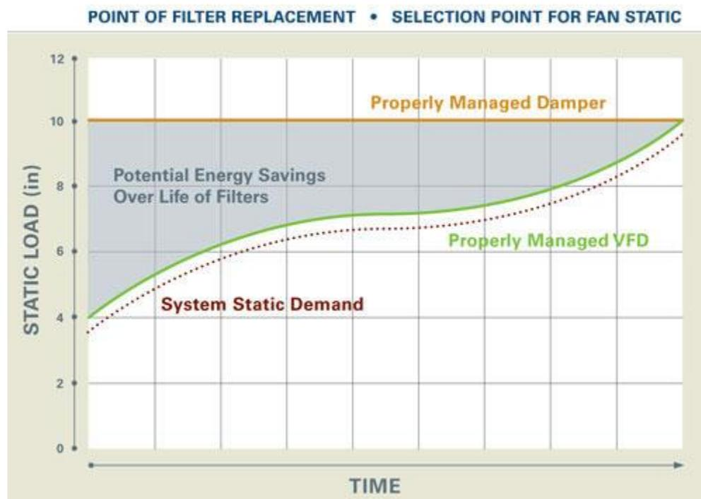
Figure 1 Design System Static <sup>2</sup>
