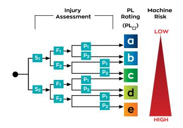
Yaskawa's FSoE servo amplifiers are capable of achieving PLe (equivalent to SIL3) which is suited for machines where serious injuries are possible, the frequency to exposure is long and/or frequent, and the possibility of avoiding injury is scarcely possible
