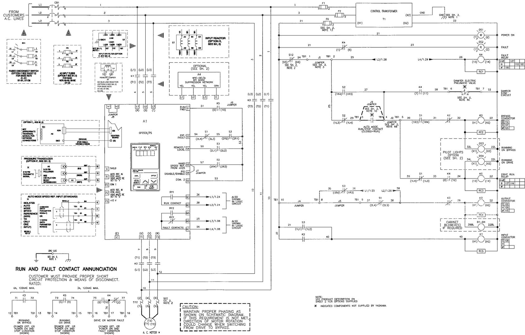
**RUN AND FAULT CONTACT ANNUNCIATION**
