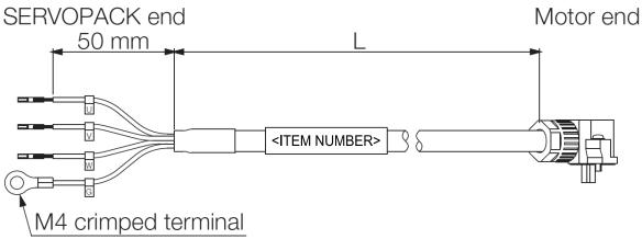
The recommended bend radius is 90mm or larger for moving parts of machines, such as robots.
