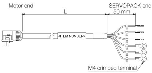
The recommended bend radius is 90mm or larger for moving parts of machines, such as robots.
