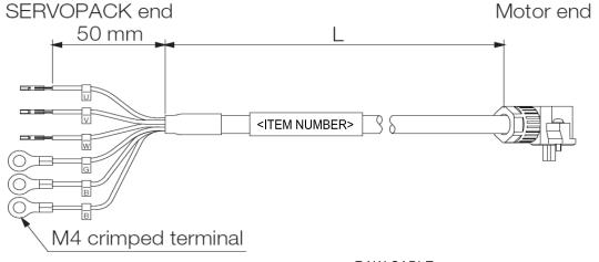
The recommended bend radius is 90mm or larger for moving parts of machines, such as robots.
