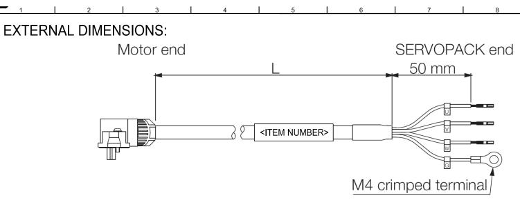
The recommended bend radius is 90mm or larger for moving parts of machines, such as robots.
