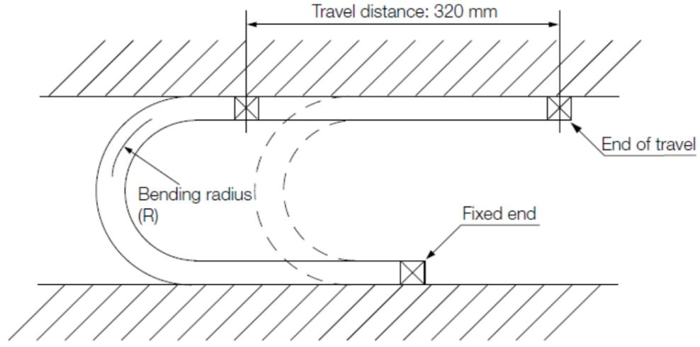
Note: The service life of a Flexible Cable indicates the number of bends while the lead wires are electrically charged for which no cracks or damage that affects the performance of the cable sheathing occurs. Breaking of the shield wire is not considered.
