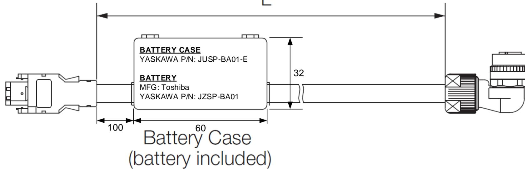
The recommended bend radius is **46mm** or larger for **moving** parts of machines, such as robots. See [Page 2](#) for Precautions for Flexible Cables.
