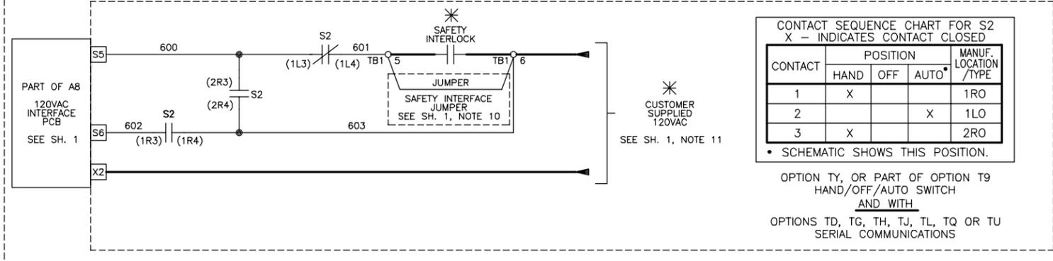
FOR ALL WIRE CONNECTION TO 120VAC INTERFACE PCB A8:
