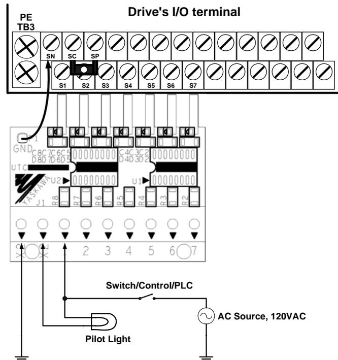
One channel shown as example, remaining channels are identical.
