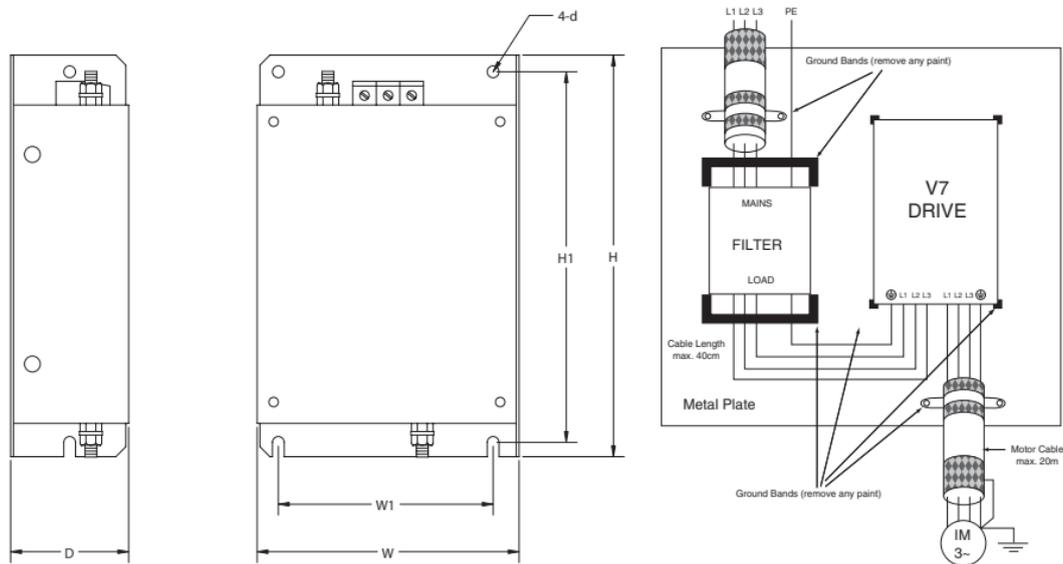
**Figure 1-4. Installation of Line Filter and V7N Drive**
