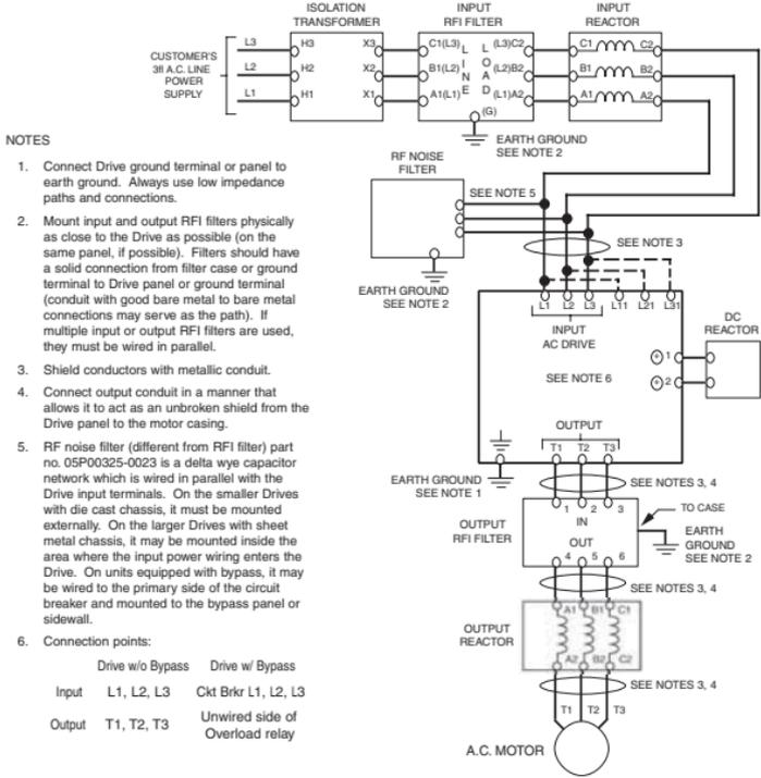
**Figure 1-3. Customer Connection Diagram For Isolation Transformers, Input Reactors, Input RFI Filters, DC Reactors, Output Reactors and Output RFI Filters**
