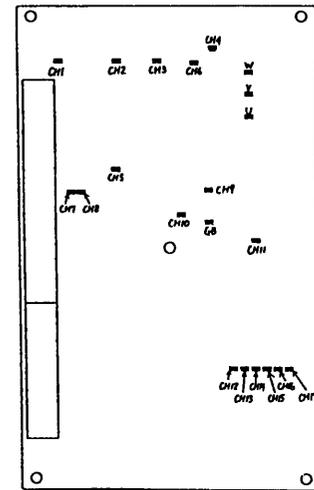
Fig. 9 Control Circuit Board Check Terminals
