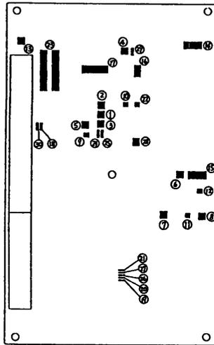
Fig. 8 Adjuster Locations on Control Circuit Board
