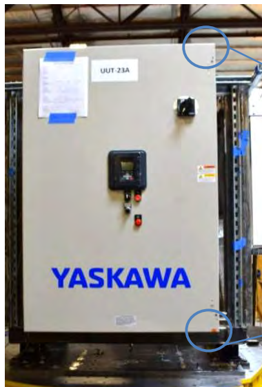
All units were filled with contents and maintained structural integrity and functionality after AC-156 test.
