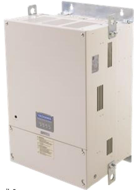
The Single Phase Converter's active power regulator insures minimal stress on the power grid, boasting less than 10% current distortion and 0.99 power factor at rated load. Combining a low harmonic solution with a soft starting variable frequency drive typically allows the opportunity to downsize transformers and decrease installation costs. The SPC utilizes the same components found in a variable frequency drive, which significantly reduces maintenance time and expenses.
