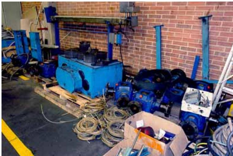
Figure 1: Old mechanical adjustable speed and power transmission components removed from a machine currently being retrofitted at Lafayette Textiles in Bogota, Colombia. These components will be replaced with 9 Yaskawa inverters in a common bus configuration with Electronic LineShaft (ELS) software. Instant gain in uptime, performance and energy savings.
