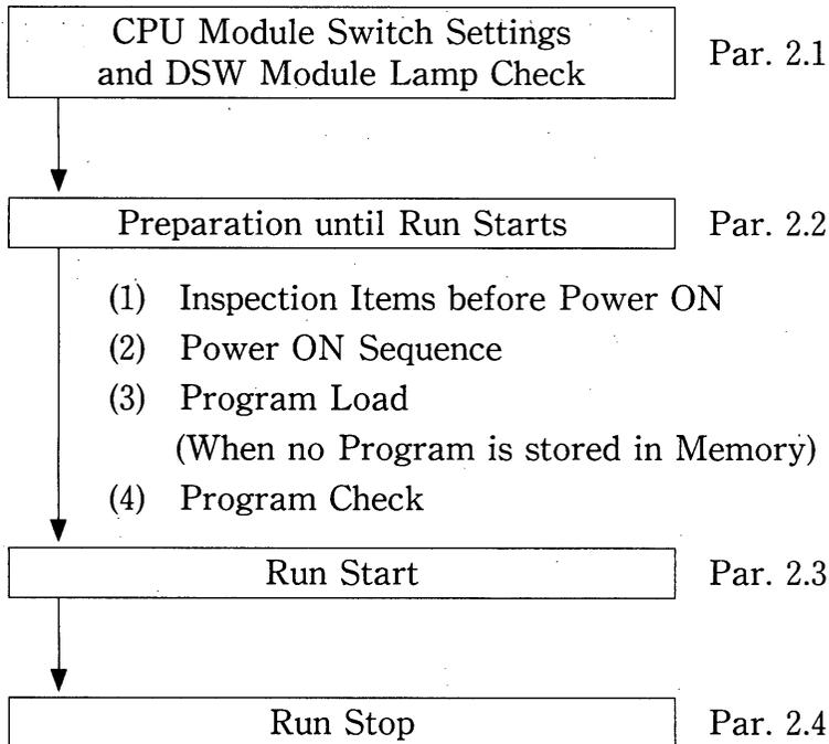
Fig. 2.1 Run Operation Procedure of CP-3300
