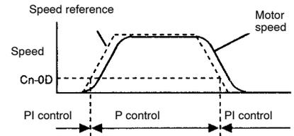
The mode switch is used to reduce settling time.
