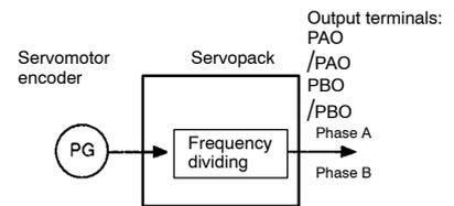
The number of output pulses per revolution is set in this parameter. Set this value according to the reference unit of the machine or controller to be used.
