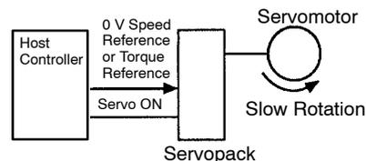
Turn ON the servo ON (/S-ON) signal.
