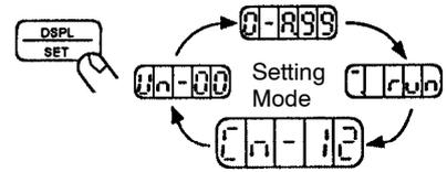
3) Select the parameter number Cn-00. (Parameter Cn-00 is selected when the power is turned ON.)
