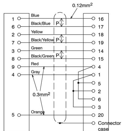
**Connectors and Terminals for Standard Motor**
