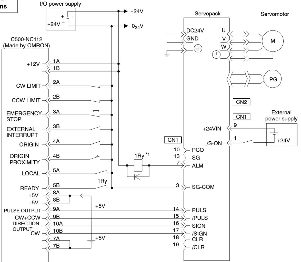
\*1 The ALM signal is output for approximately two seconds when the power is turned ON. Consider this when designing the power ON sequence. Use the ALM signal to operate the alarm detection relay (Relay 1Ry) and turn OFF the power supply to the Servopack.
