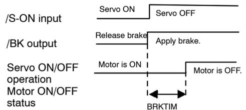
With the standard setting, the servo is turned OFF when /BK signal (brake operation) is output. The machine may move slightly due to gravitation. This movement depends on machine configuration and brake characteristics. If this happens, use this parameter to delay servo OFF timing to prevent the machine from moving.
