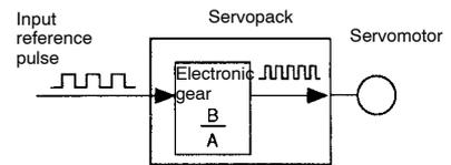
$$\text{Electronic gear ratio } \left(\frac{B}{A}\right) = \frac{\text{Cn-24}}{\text{Cn-25}}$$
