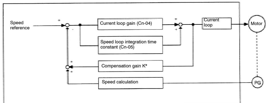
\* Compensation gain (K) is in proportion to the compensation constant (parameter Cn-28). Cn-28 = 0 shows no compensation status.
