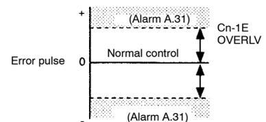
If the machine permits only a small position loop gain value to be set in Cn-1A, an overflow alarm may arise during high-speed operation. In this case, increase the value set in this parameter to suppress alarm detection.
