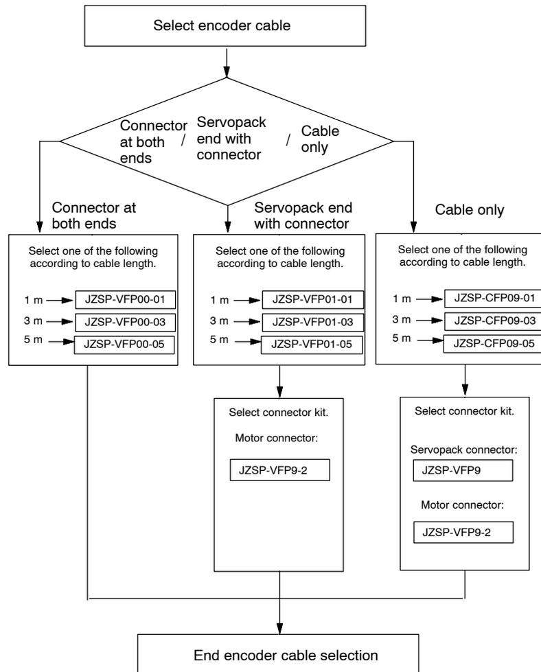
**Encoder Cables: Connector at Both Ends**
