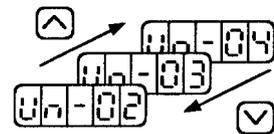
3) Press **DATA ENTER** to display the data for the monitor number selected at step 2.
