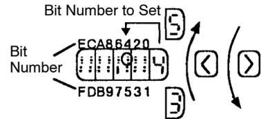
5) Press the **^** and **v** keys to set the memory switch data ON or OFF for the bit number.
