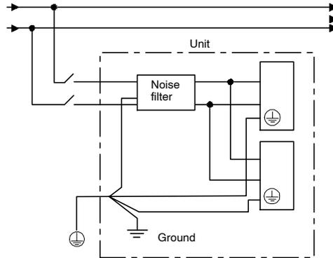
Multiple servos can share a single MCCB or noise filter. Always select an MCCB or noise filter that has enough capacity for the total power capacity (load conditions) of those servos. For details, refer to page 2-68.
