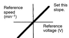
The factory setting is 500 [rated speed (3000 min<sup>-1</sup>)/6 V = 500].
