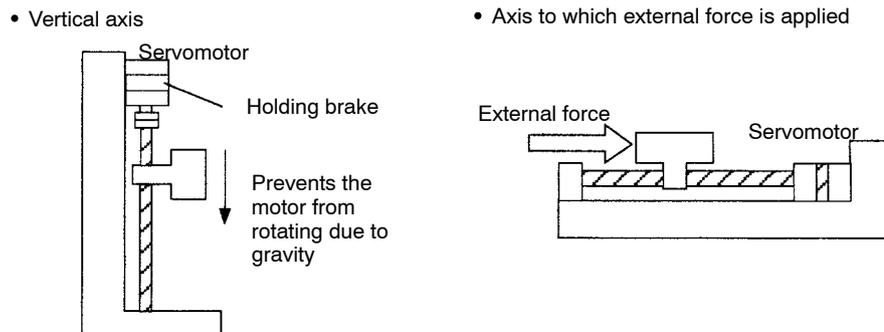
**Note** To prevent faulty operation caused by gravity (or external force), first check that the Servomotor and holding brake operate normally with the Servomotor disconnected from the machine. If all operations are normal, connect the Servomotor to the machine and conduct a test run.
