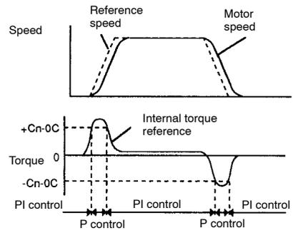
If a mode switch is not used and PI control is always performed, torque may enter a saturation state during acceleration or deceleration, causing the motor speed to have overshoot or undershoot.
