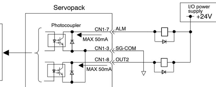
**Note** Provide an external I/O power supply separately. There are no power terminals to which the Servopack outputs signals externally. Yaskawa recommends that this external power supply be the same type as for the input circuit.
