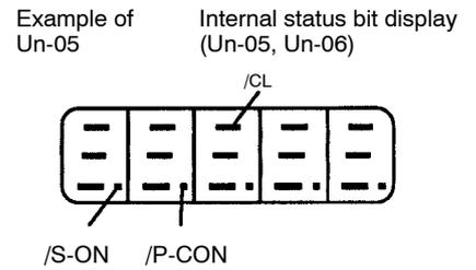
Turn each connected signal line ON and OFF to check that the monitor bit display changes accordingly as shown below.
