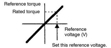
The factory setting is 30, so the rated torque is 3 V (30 x 0.1).
