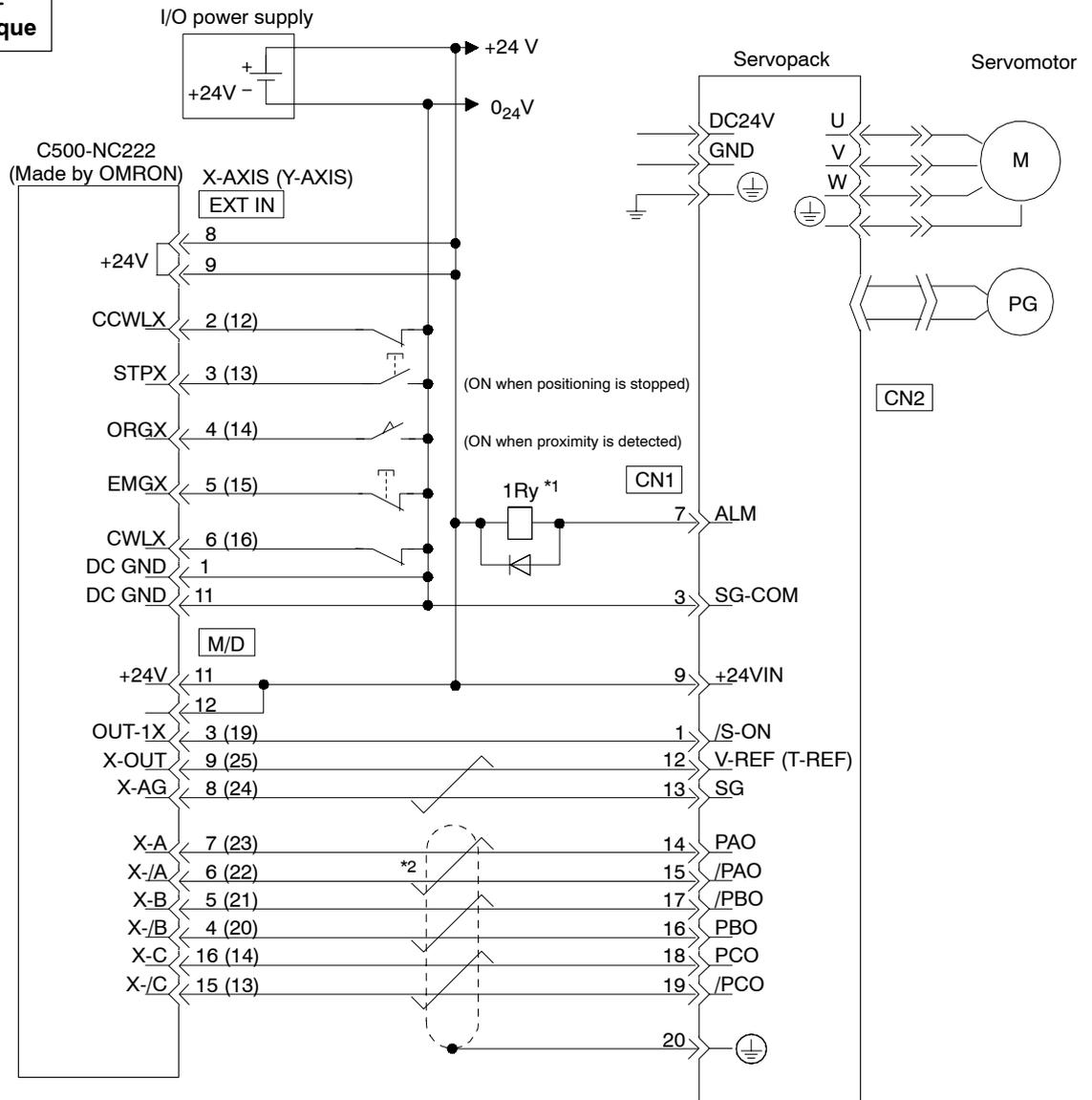
\*1 The ALM signal is output for approximately two seconds when the power is turned ON. Consider this when designing the power ON sequence.
