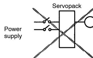
Do not start and stop by turning power ON and OFF
