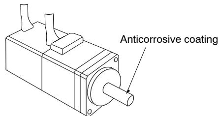
**Note** Do not get thinner on any other parts of the Servomotor when cleaning the shaft.
