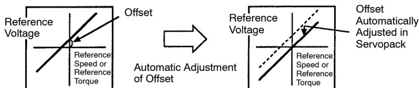
After completion of offset automatic adjustment, the amount of offset is stored in the Servopack.
