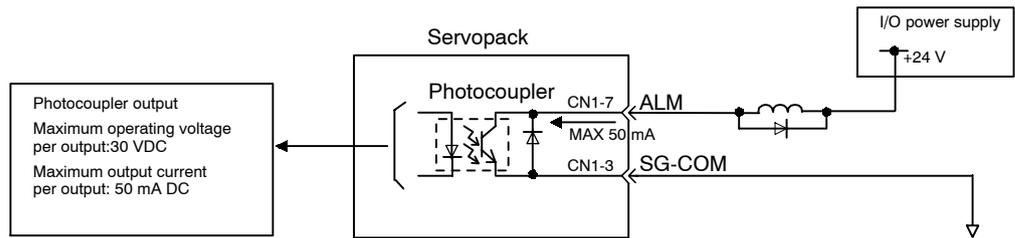
Provide an external I/O power supply separately. There are no DC power available from Servopack for output signals.
