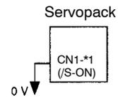
When external short-circuit wiring is omitted, set the memory switch to "1."
