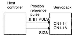
Set also the input pulse logic in bit D of Cn-02.
