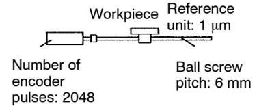
Machine conditions and reference unit must be defined for the electronic gear function beforehand.
