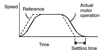
Mode switch is used to reduce settling time and suppress undershoot when the motor stops. It switches PI control to P control when certain conditions are met.
