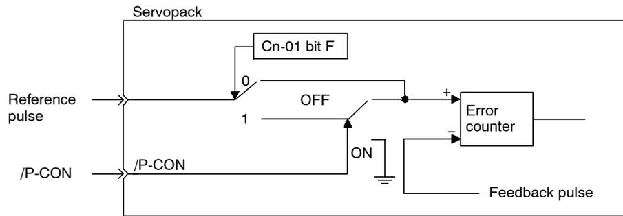
**Note** Use Cn-01 bit F to enable/disable the INHIBIT function.
