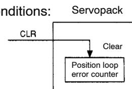
Use this signal to clear the error counter from the host controller.
