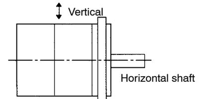
**Note** In Servomotors, an accurate detector is attached to the shaft at the opposite end from the load. Do not apply direct impact to the shaft as it may damage the detector.
