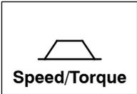
The soft start function adjusts progressive speed reference input inside the Servopack so that acceleration and deceleration can be as constant as possible. To use this function, set the following parameters.
