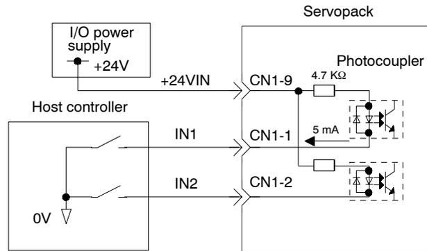
**Note** Provide an external I/O power supply separately. There are no power terminals to which the Servopack outputs signals externally.
