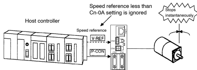
Set the following memory switch so that input signal /P-CON can be used to enable or disable the zero-clamp function.
