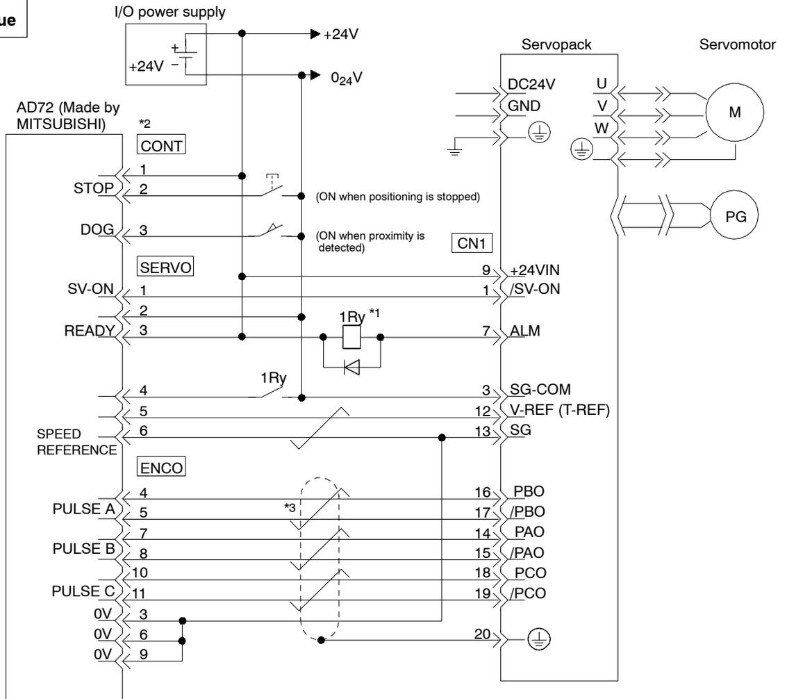
\*1 The ALM signal is output for approximately two seconds when the power is turned ON. Consider this when designing the power ON sequence.
