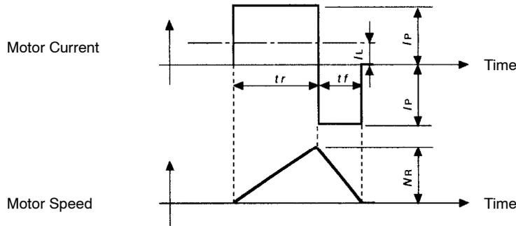
Motor Current (size) - Motor Speed Timing Chart
