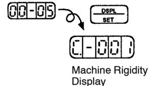
6) Press the and keys to select the machine rigidity. If the actual rigidity is unknown, select medium rigidity.
