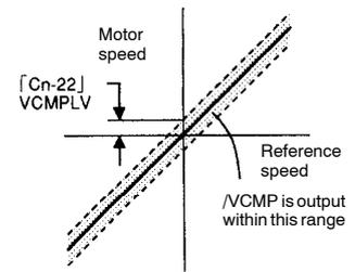
Example: When preset value is 100 and reference speed is 2000 min<sup>-1</sup>.
