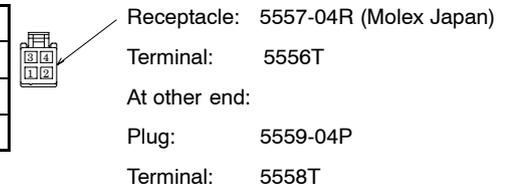
Motor Connection Specifications: With Brake
