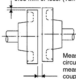
Measure this distance at four different positions in the circumference. The difference between the maximum and minimum measurements must be 0.03 mm or less. (Turn together with couplings)
