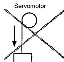
Do not apply regenerative braking continuously.
