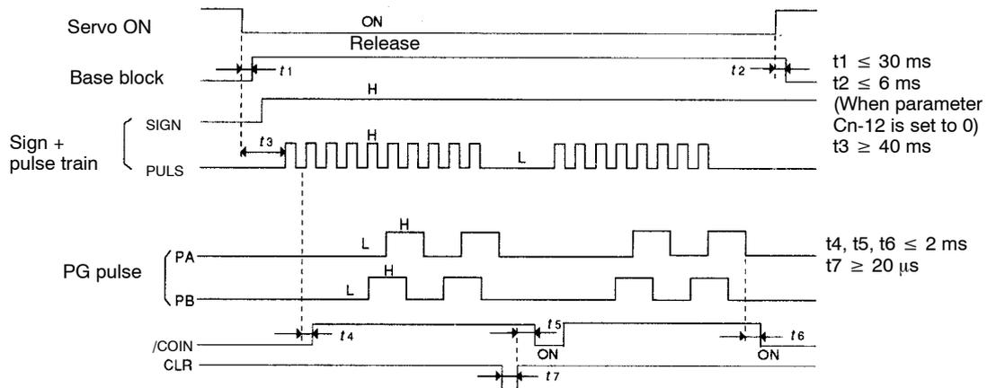
**Note** (1) The interval from the time the Servo ON signal is turned ON until a reference pulse is input must be at least 40 ms. Otherwise, the reference pulse may not be input.
