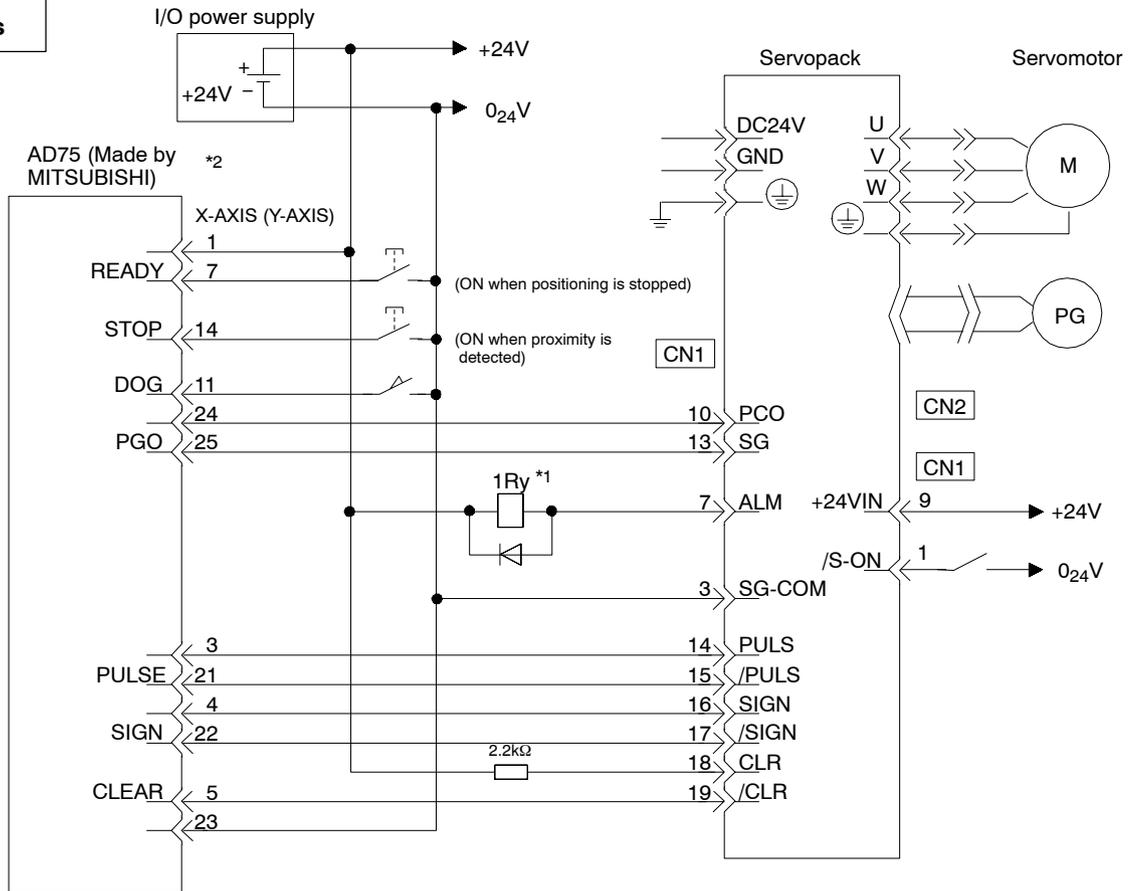
\*1 The ALM signal is output for approximately two seconds when the power is turned ON. Consider this when designing the power ON sequence. Use the ALM signal to operate the alarm detection relay (Relay 1Ry) and turn OFF the power supply to the Servopack.
