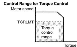
This parameter is used to prevent machine over-speed during torque control.
