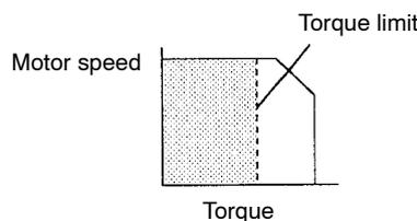
Too small a torque limit value will result in torque shortage at acceleration or deceleration.
