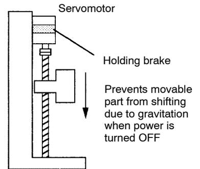
**Note** The Servomotor with brake has a built-in brake that is a de-energization operation type, which is used for holding purposes only. The brake cannot be used to stop the motor. Use the holding brake only to retain a stopped motor. Brake torque is more than 100% of the rated motor torque.
