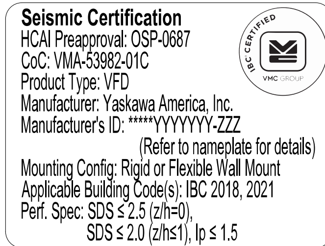
Figure 5.26 Seismic Certification Label Example for Drives
