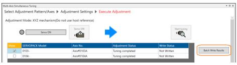
If using SCARA robot mechanism, tuning results for the axes that were optionally selected can be written individually. Select the [Show] check box for the axes to be written, and then click [Write Results] button.
