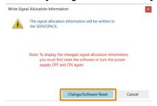
The software will be reset, the changes to the I/O signal allocations and polarities will be applied, and the backgrounds of the cell will return to white.
