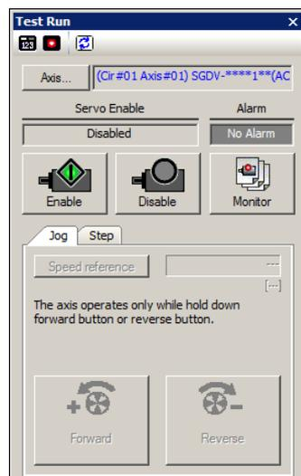
**Information** The Test Run can be performed only on the selected axis. To set up other axes, click the Axis Button and select the axis in the Axis Selection Dialog Box. Repeat this for each axis.
