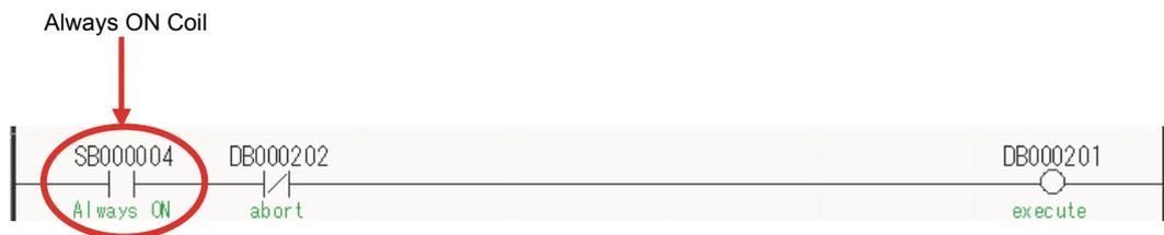
**2. Start the message send operation on the OMRON PLC.**
