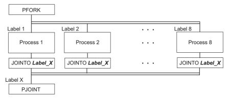
Fig. 6.63 Using the PFORK, JOINTO, and PJOINT Instructions
