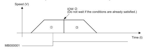
• When the Continuous Process Control Signal Turns ON during Distribution for MVS ① (during Deceleration)
