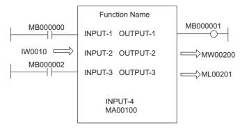
Fig. 6.70 Programming Example for the UFC Instruction
