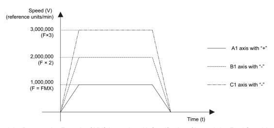
Fig. 6.27 Programming Example of MVS Instruction with Specification of Interpolation Feed Speed Axes
