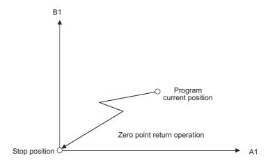
Fig. 6.45 Programming Example for the ZRN Instruction
