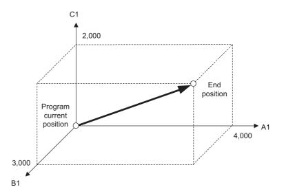
Fig. 6.35 Programming Example for MVS Instruction
