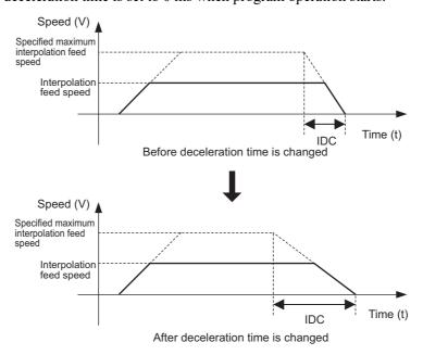
Fig. 6.23 Change Interpolation Deceleration Time
