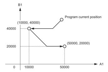
Fig. 6.2 Programming Example for the ABS Instruction
