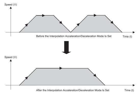
Fig. 6.29 Set Interpolation Acceleration/Deceleration Mode
