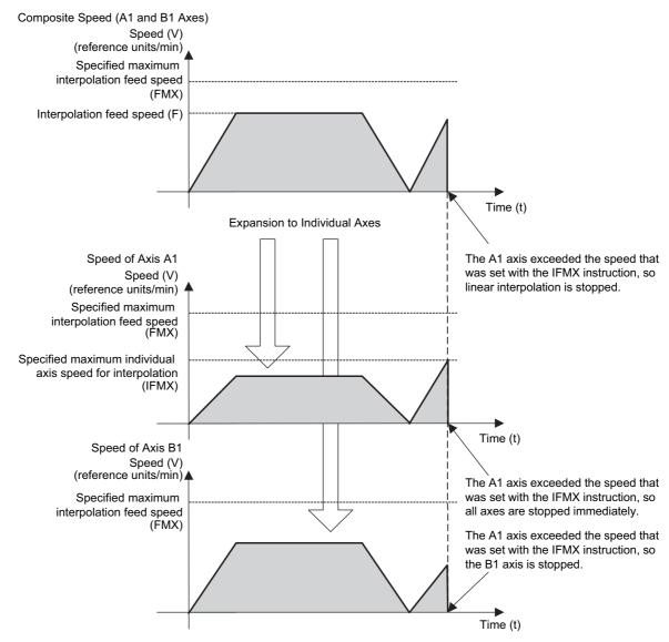
Fig. 6.18 Maximum Individual Axis Speed Settings for Interpolation
