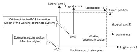
Fig. 6.54 Working Coordinate System Set with POS Instruction
