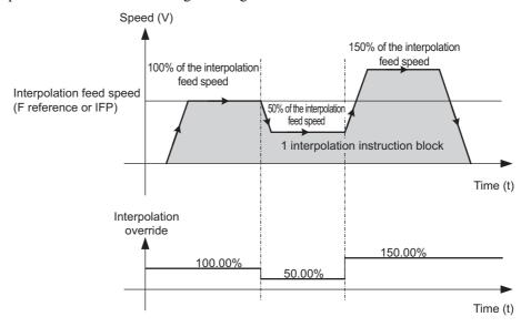
Fig. 6.34 Interpolation Override and Interpolation Instructions
