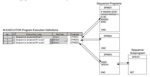
If the execution type is set to a high-speed scan sequence program or low-speed scan sequence program, then the program will be executed as soon as the definition is saved. If the execution type is set to a startup sequence program, then the program will be executed the next time when the power supply is turned ON.
