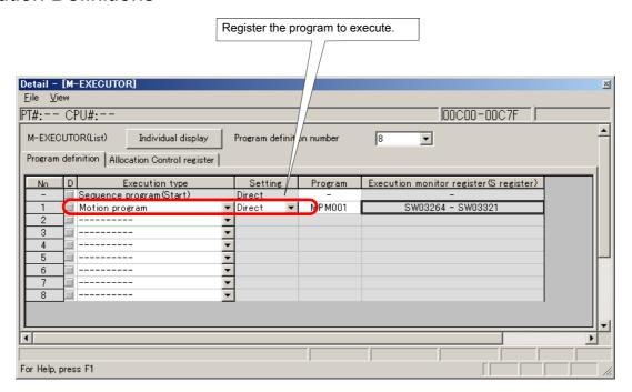
When a program is registered for execution, that program is assigned work registers to control and monitor the execution of the program. The work registers are used to send commands to the motion programs from the motion program control program, and to get the motion program status.
