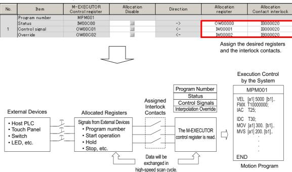
The assigned interlock contacts are used to interlock motion program operation. If you assign registers, always assign interlock contacts.
