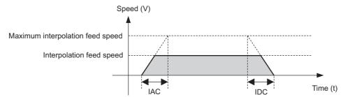
Before the Interpolation Acceleration/Deceleration Unit Is Changed
