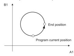
• If program current position = end position, the circular path consists of 3 circles.
