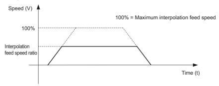
Fig. 6.19 Set Interpolation Feed Speed Ratio
