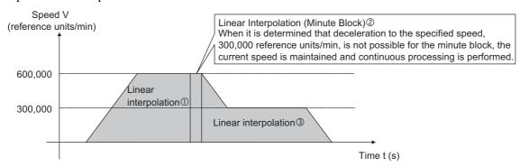
• Operation in Interpolation Acceleration/Deceleration Mode 3
