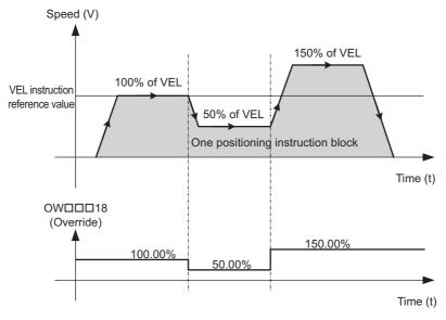
Fig. 6.15 OW□□□18 (Override) and Positioning Instructions
