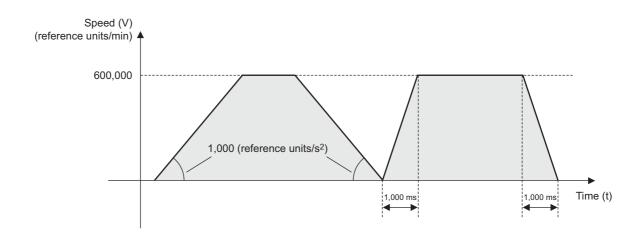
Set Interpolation Feed Speed Axes (+ and -)
