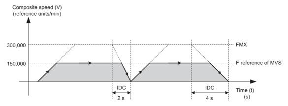
Fig. 6.24 Programming Example for IDC Instruction
