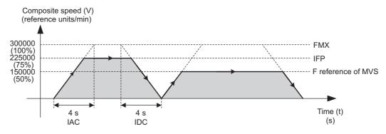
Fig. 6.17 Programming Example for the FMX Instruction
