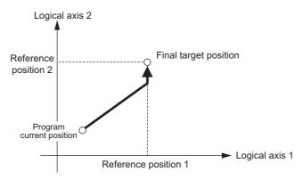
Fig. 6.1 Movement Mode for ABS Instruction
