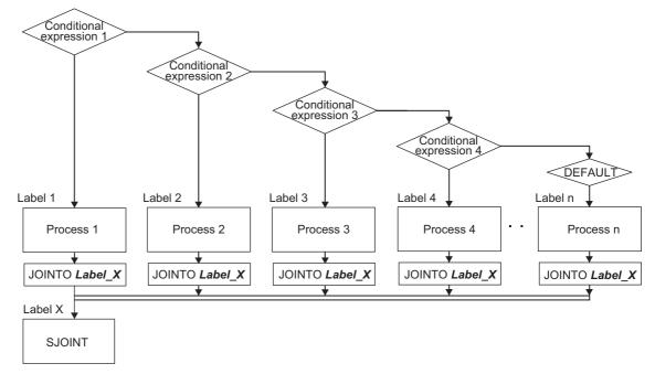
Fig. 6.66 Using the SFORK, JOINTO, and SJOINT Instructions
