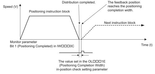
Fig. 6.31 In-Position Check Operation
