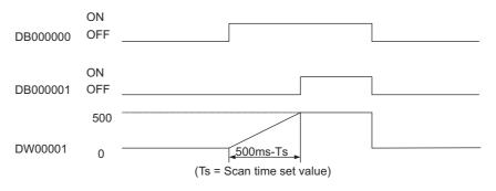
Off-delay Timer: Measurement unit = 10 ms (TOF)
