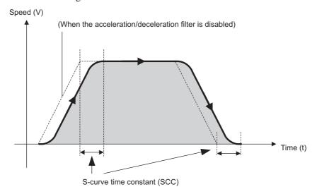
Specify a numerical value or register for the S-curve time constant for each axis by using the SCC instruction.
