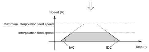
After the Interpolation Acceleration/Deceleration Unit Is Changed
