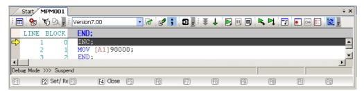
In Debug Operation Mode, the program line that is being executed is highlighted at the top of the tab page.
