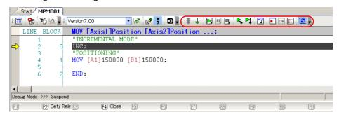
4. Click the lcon to execute the program line by line, and check the operation of the program.
