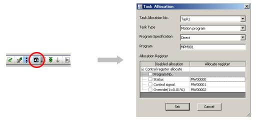
• Open the Detail Definition for the M-EXECUTOR under Module Configuration, then click the Individual display 1 Icon.
