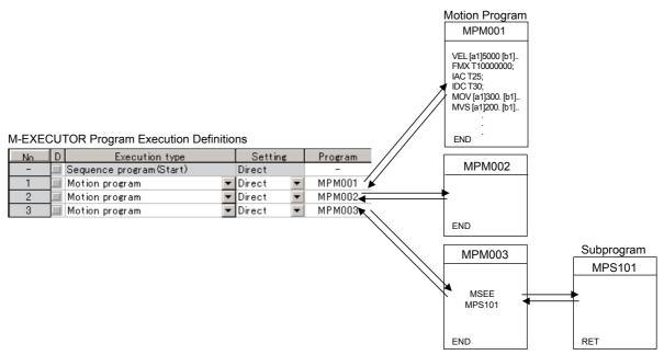
To execute a motion program, first register the program in the M-EXECUTOR program execution definitions, then use a control signal to turn ON the request for start of program operation.
