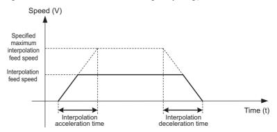
Fig. 6.16 Set Maximum Interpolation Feed Speed
