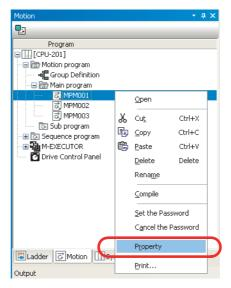
2. Select the parallel execution mode under **PFORK Parallel Execution Mode** in the Program Properties Dialog Box.
