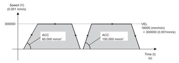
Fig. 6.7 Programming Example 2 for the ACC Instruction
