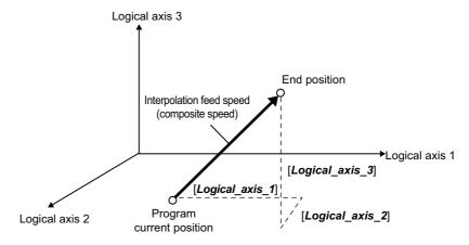
Fig. 6.33 Movement Path for the MVS Instruction
