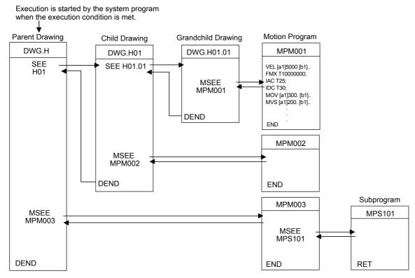
The ladder instructions in the high-speed drawing are executed every high-speed scan cycle according to the hierarchical organization of parent-child-grandchild drawings.
