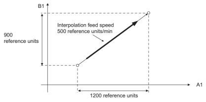
The feed speed of each axis is calculated using the following formula.
