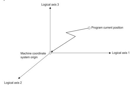
Fig. 6.44 Movement Path for the ZRN Instruction
