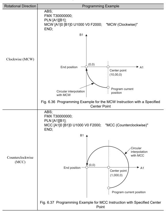
When used with a specified radius, the MCW or MCC instruction moves two axes simultaneously from the program current position to the end position on the specified plane at the interpolation feed speed along the circle determined by the radius.
