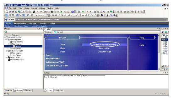
**2.** Select the desired communications port in the **Communication Port** Box on the Communications Setting Dialog Box. Click the **Connection** Button.
