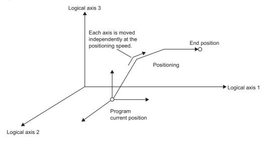
Fig. 6.30 Movement Path for the MOV Instruction
