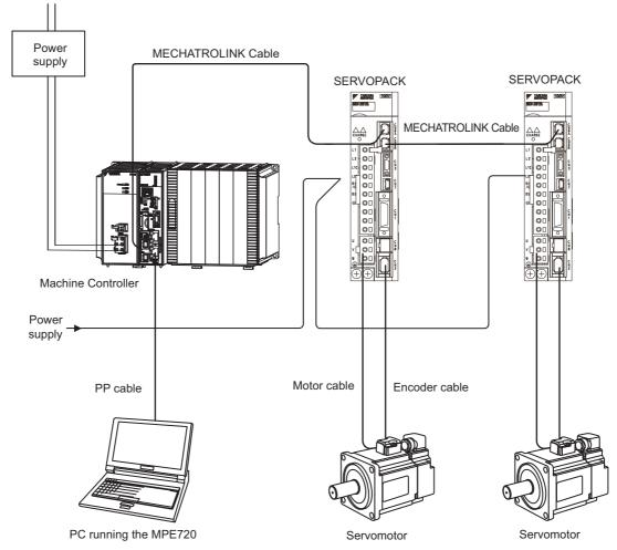
Note: In the system configuration example that is given above, the SERVOPACK station numbers are set to 1 and 2.
