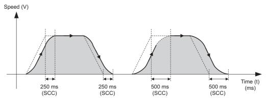
Fig. 6.12 Programming Example for the SCC Instruction
