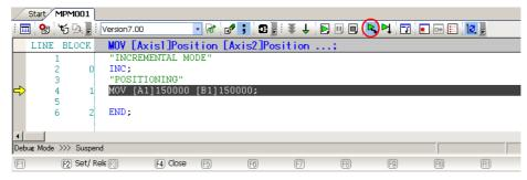
**5.** Step through the program until the END instruction. When debugging is completed, turn OFF the power to the Servomotor.
