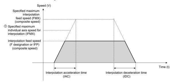
① Maximum Individual Axis Speed for Interpolation
