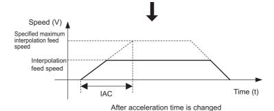
Fig. 6.21 Change Interpolation Acceleration Time
