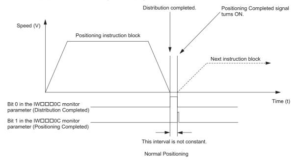
The following figure shows the positioning operation for the DEN instruction.
