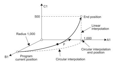
Fig. 6.43 Programming Example for the MCC Instruction with a Specified Radius
