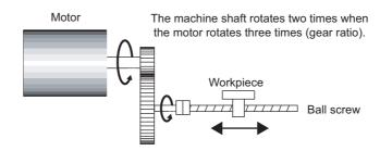
The table moves 10 mm per revolution. (travel distance per machine rotation)
