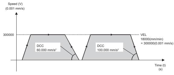
Fig. 6.10 Programming Example 2 for the DCC Instruction
