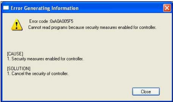
Fig. E.1 This Error Message is Displayed If an Attempt is Made to Open a User Application (i.e., ladder, motion, or C language).
