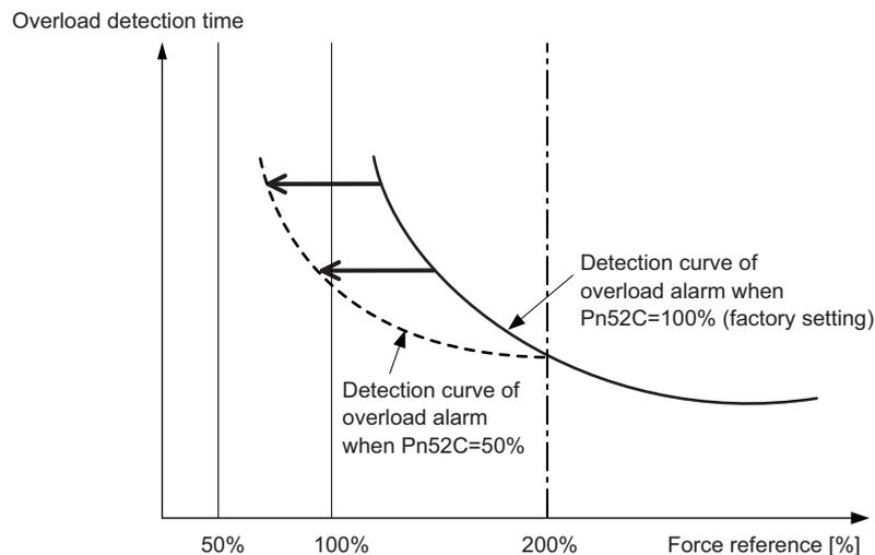
Note: For details, refer to *Overload Characteristics* listed in the section for the relevant servomotor in the *Σ-V Series Product Catalog* (No.: KAEP S800000 42).
