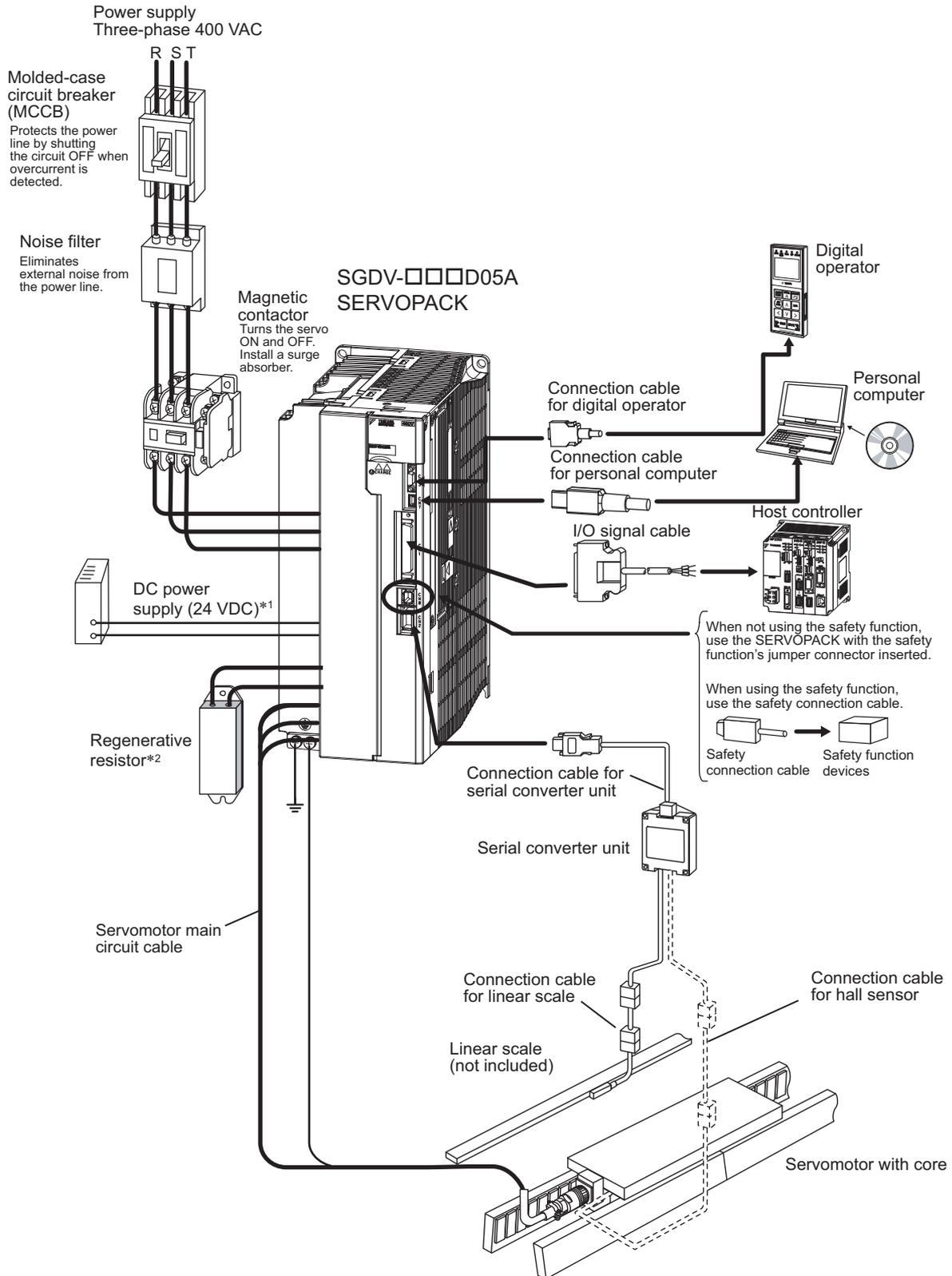
\*1. Use a 24-VDC power supply with double insulation or reinforced insulation. (The power supply is not included.)
