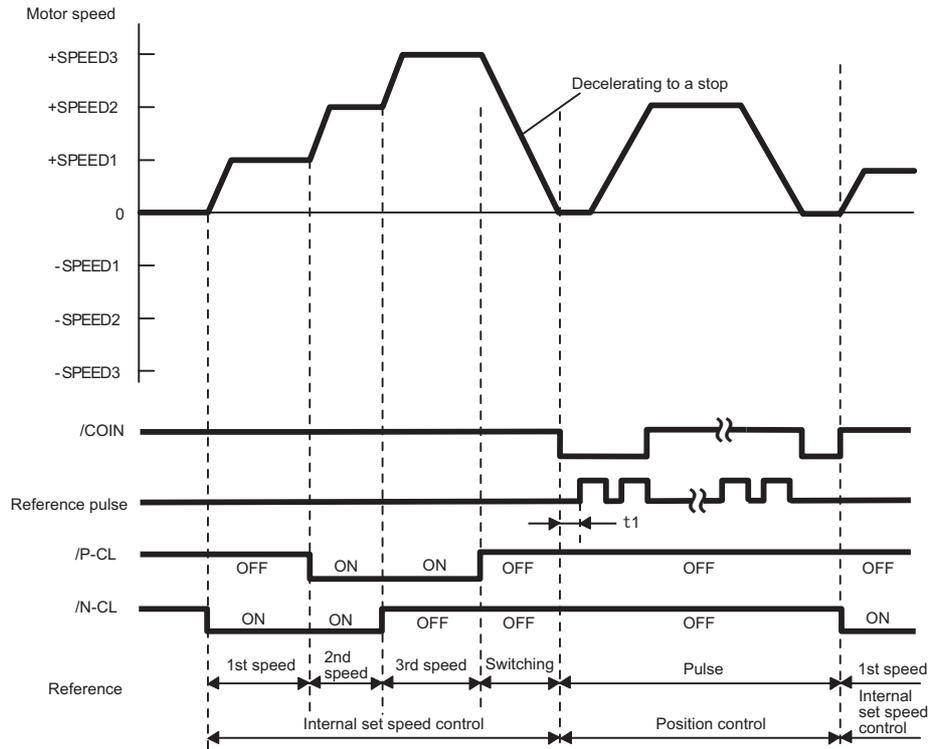
Note 1. The  $t_1$  value is not affected by whether the soft start function is used.
