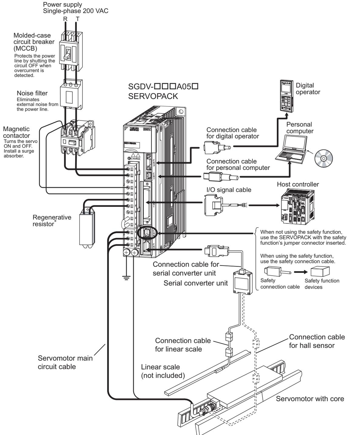
\* Before connecting an external regenerative resistor to the SERVOPACK, refer to 3.6 *Connecting Regenerative Resistors*.
