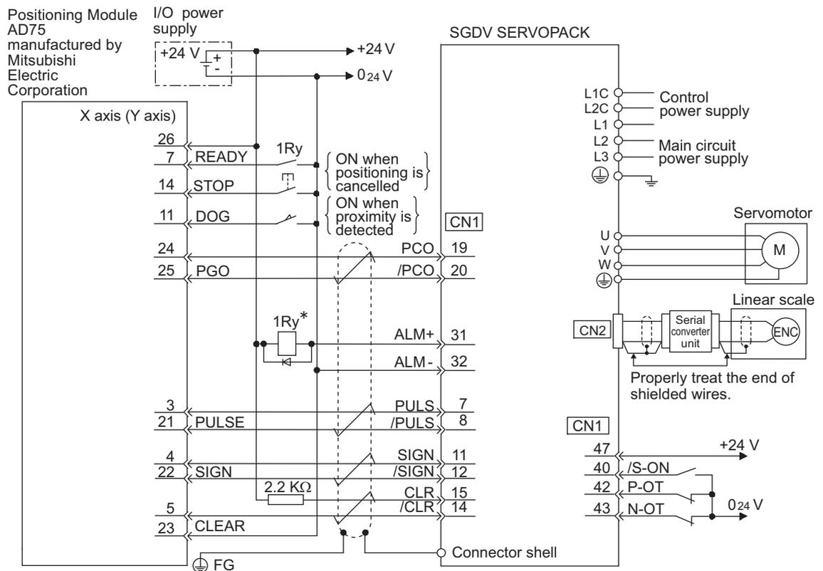
\* The ALM signal is output for about five seconds when the control power is turned ON. Take this into consideration when designing the power ON sequence. Also, use the ALM signal to actuate the alarm detection relay 1Ry to stop the main circuit power supply to the SERVOPACK.
