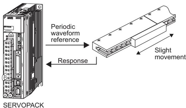
In addition to this function, online vibration monitor (Fn207) can be used to detect machine vibration and automatically make notch filter settings.
