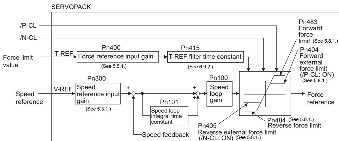
Note: This function cannot be used during force control since the force limit by analog voltage reference is input from T-REF (CN1-9, 10).
