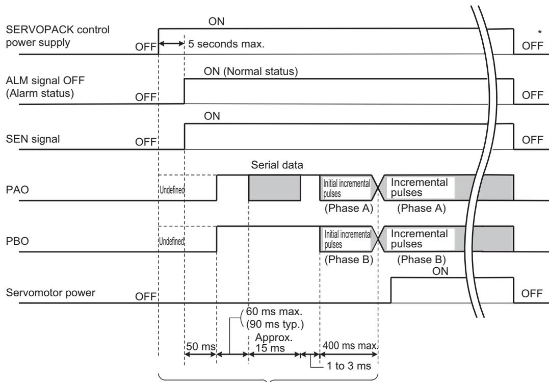
The servomotor will not be turned ON even if /S-ON is turned ON during this interval.
