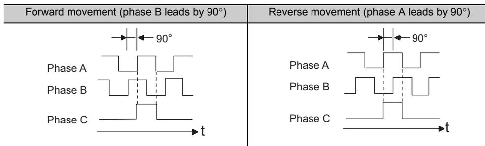
Note: The pulse width for phase C (origin pulse) changes according to the setting of the encoder output resolution (Pn281) and becomes the same as that for phase A.
