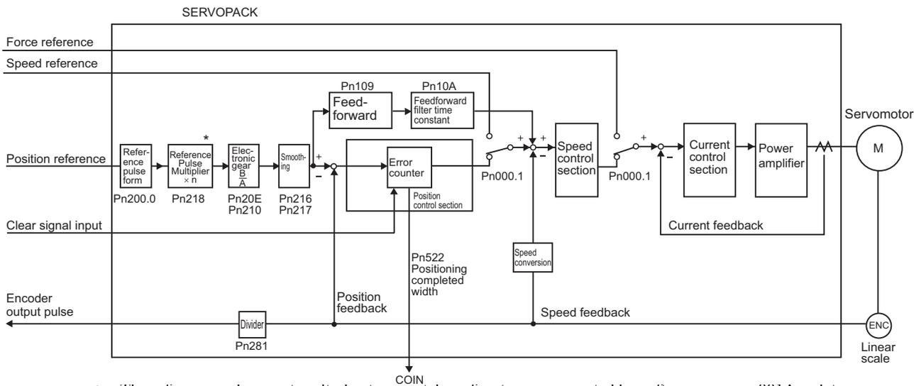
\* The reference pulse input multiplication switching function is supported by software version 001A or later.
