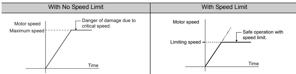
The parameters related to the speed limit, such as for selecting the speed limit method, are described next.
