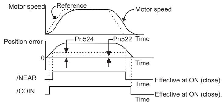
Note: Normally, the value of Pn524 should be larger than that for the positioning completed width (Pn522).
