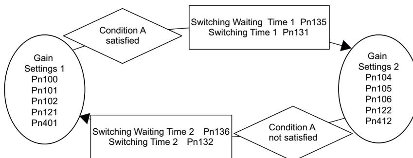
■ Relationship between the Waiting and Switching Times for Gain Switching
