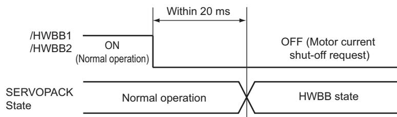
Note 1. The OFF status is not recognized if the total OFF time of the /HWBB1 and /HWBB2 signals is 0.5 ms or shorter.
