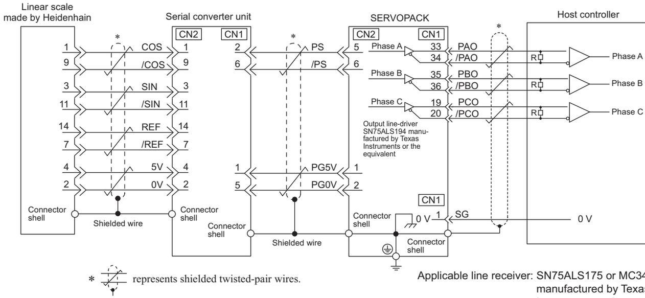
Applicable line receiver: SN75ALS175 or MC3486 manufactured by Texas Instruments, or the equivalent
