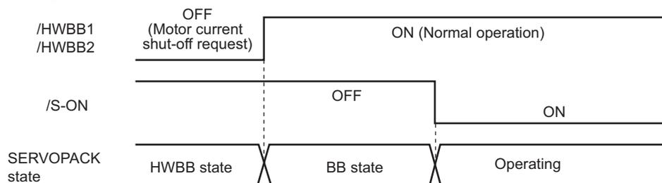
If the /HWBB1 and /HWBB2 signals are OFF and the servo ON signal is ON, the HWBB state will be maintained after the /HWBB1 and /HWBB2 signals are turned ON.
