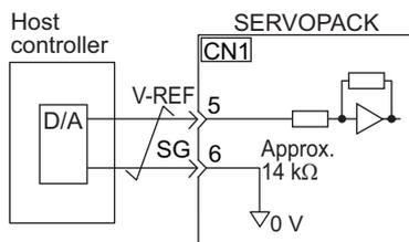
Note: Always use twisted-pair cable to control noise.
