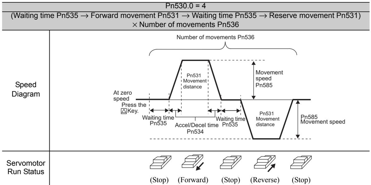
Note: When Pn536 (number of times of program JOG movement) is set to 0, infinite time operation is enabled. To stop infinite time operation, press the MODE/SET Key (or JOG/SVON Key of digital operator) to turn OFF the servomotor power.
