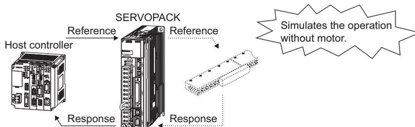
Use Pn00C.0 to enable or disable the test without a motor.
