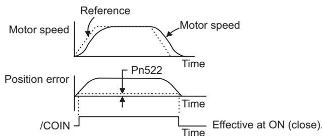
Note: If the parameter is set to a value that is too large, a positioning completed signal might be output if the position error is low during a low speed operation. This will cause the positioning completed signal to be output continuously. If this signal is output unexpectedly, reduce the set value until it is no longer output.
