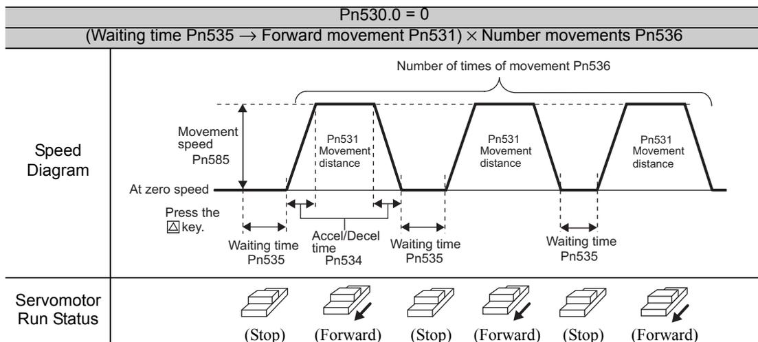
Note: When Pn536 (number of times of program JOG movement) is set to 0, infinite time operation is enabled. To stop infinite time operation, press the MODE/SET Key (or JOG/SVON Key of digital operator) to turn OFF the servomotor power.
