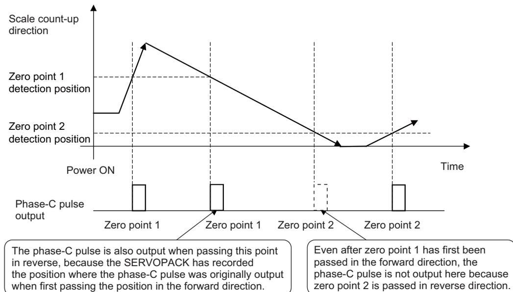
■ Linear Scale with Multiple Zero Points and Passing First Zero Point in Reverse Direction after Power ON
