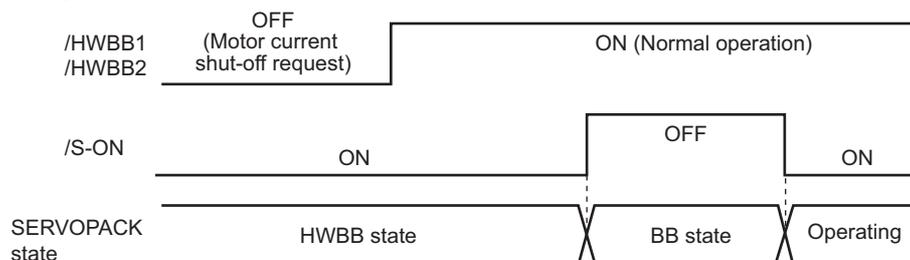
Note 1. If the SERVOPACK is placed in a BB state with the main power supply turned OFF, the HWBB state will be maintained until the servo ON signal is turned OFF.
