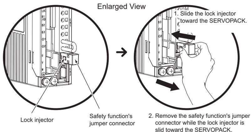
Note: The safety function's jumper connector may be damaged if removed while the lock is still on.
