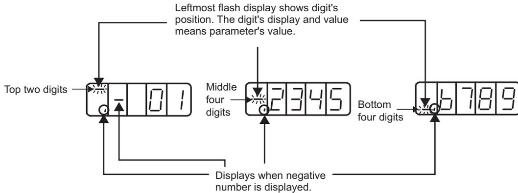
The example below shows how to set the positioning completed width (Pn522) to "0123456789."
