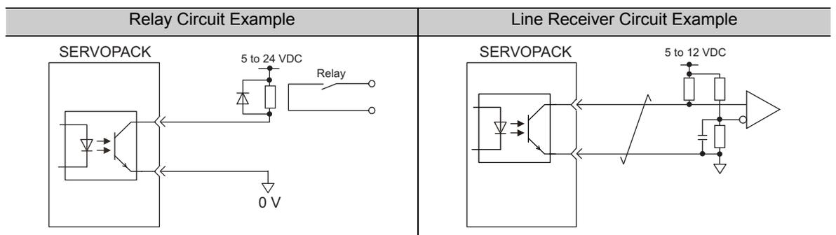
Note: The maximum allowable voltage and current range of the photocoupler output circuit are as follows:
