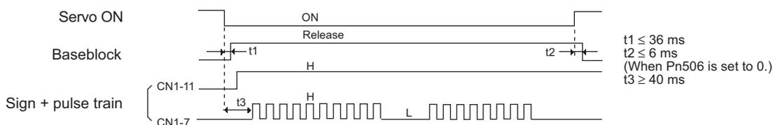
Note: The interval from servo ON to when the input pulse is input (t3) must be at least 40 ms. Otherwise the reference pulses may not be received by the SERVOPACK.
