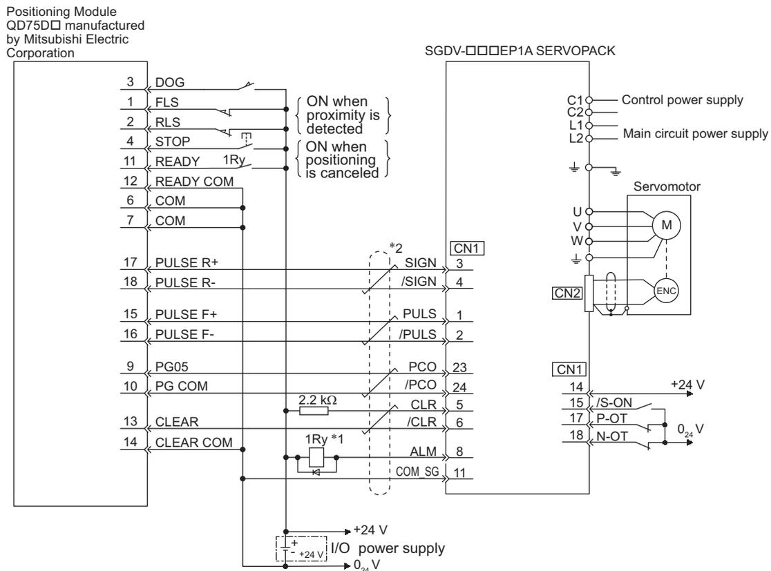
\*1. The ALM signal is output for about five seconds when the control power is turned ON. Take this into consideration when designing the power ON sequence. Also, use the ALM signal to actuate the alarm detection relay 1Ry to stop the main circuit power supply to the SERVOPACK.
