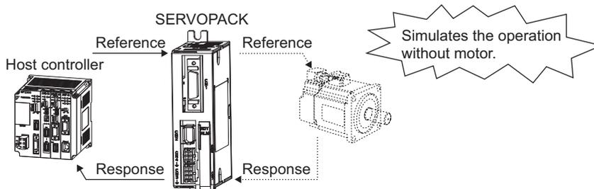
Use Pn00C.0 to enable or disable the test without a motor.
