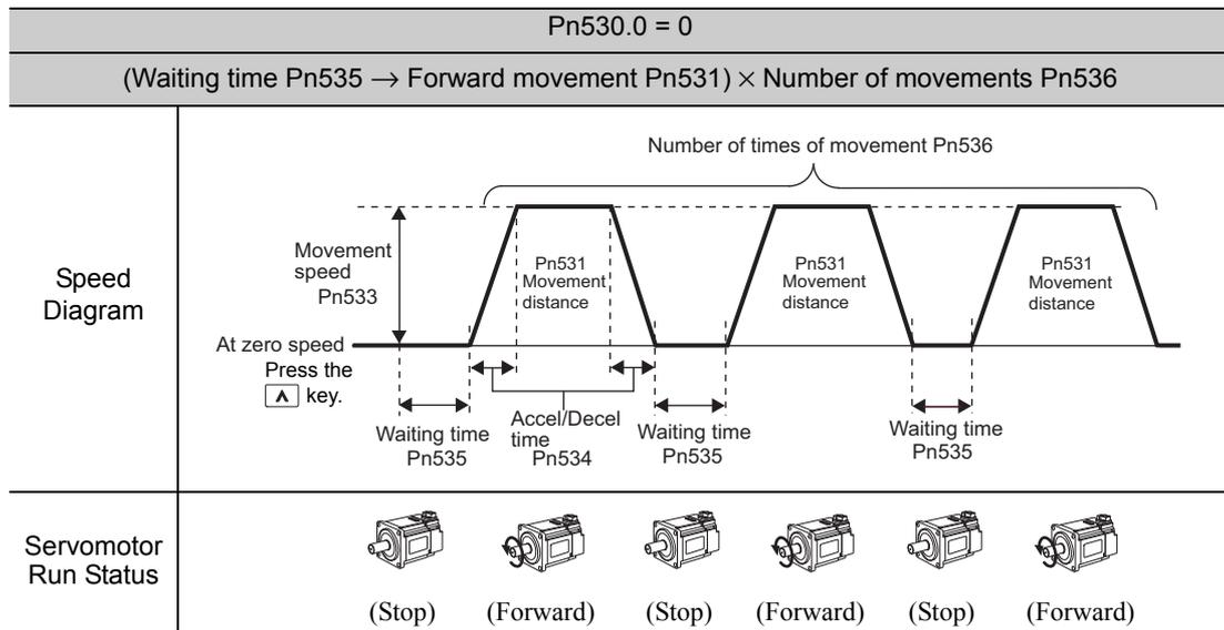
Note: When Pn536 (number of times of program JOG movement) is set to 0, infinite time operation is enabled. To stop infinite time operation, press the JOG/SVON Key of digital operator to turn OFF the servomotor power.
