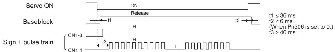
Note: The interval from the time the servo ON signal is turned ON until a reference pulse is input must be at least 40 ms. Otherwise the reference pulse may not be received by the SERVOPACK (t3).
