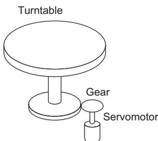
Because the turntable moves in only one direction, the upper limit for revolutions that can be counted by an absolute encoder will eventually be exceeded. The multiturn limit setting is used in cases like this to prevent fractions from being produced by the integral ratio of the motor revolutions and turntable revolutions.
