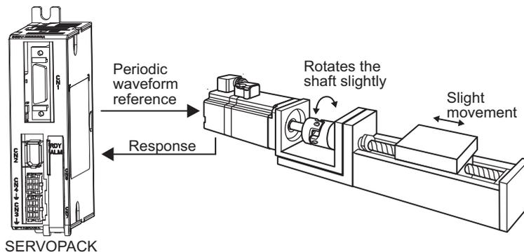
In addition to this function, online vibration monitor (Fn207) can be used to detect machine vibration and automatically make notch filter settings.
