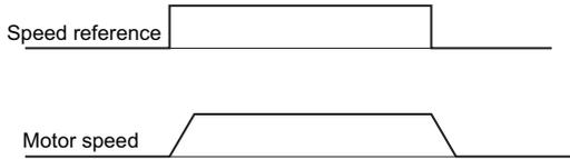
Use this function to smooth speed control (including selection of internal set speeds).
