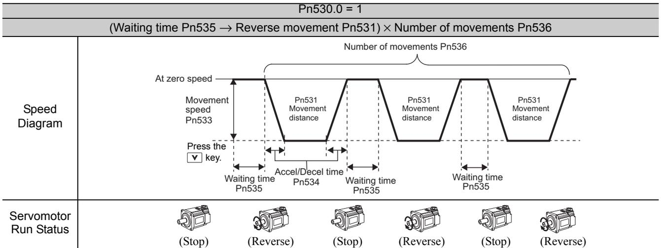
Note: When Pn536 (Number of Times of Program JOG Movement) is set to 0, infinite time operation is enabled. To stop infinite time operation, press the JOG/SVON Key of digital operator to turn OFF the servomotor power.
