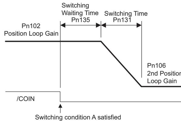
Note: Automatic gain switching is available in the PI and I-P controls (Pn10B).
