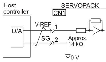
Note: Always use twisted-pair cable to control noise.
