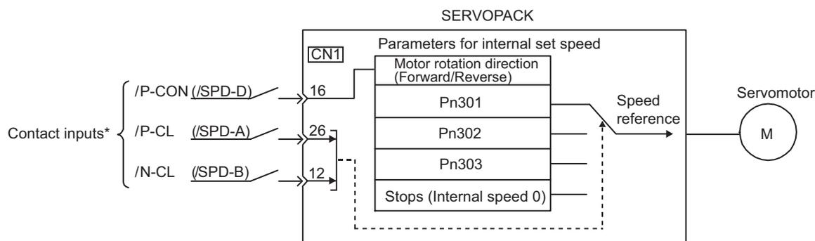
\* When using the external input signal pins as factory settings, the functions of /P-CON, /P-CL, and /N-CL change to the functions of /SPD-D, /SPD-A, and /SPD-B, respectively.
