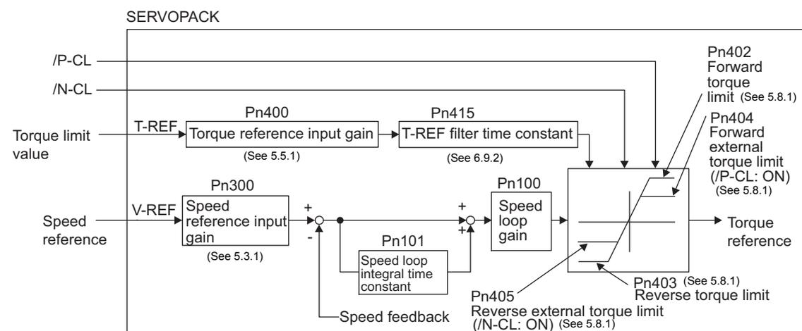
Note: This function cannot be used during torque control since the torque limit by analog voltage reference is input from T-REF (CN1-3, 4).
