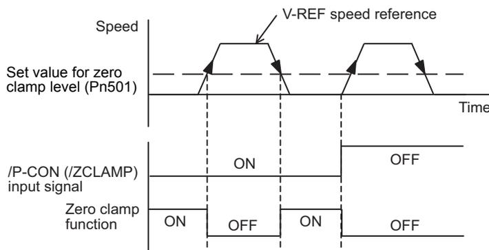
Adjust the position loop gain (Pn102) if the servomotor oscillates in the zero clamp state. If the gain switching function is used, adjusting the 2nd position loop gain (Pn106) is required as well. For details, refer to 6.8.1 *Switching Gain Settings*.
