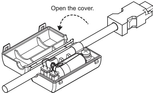
3. Remove the old battery and mount the new JZSP-BA01 battery as shown below.
