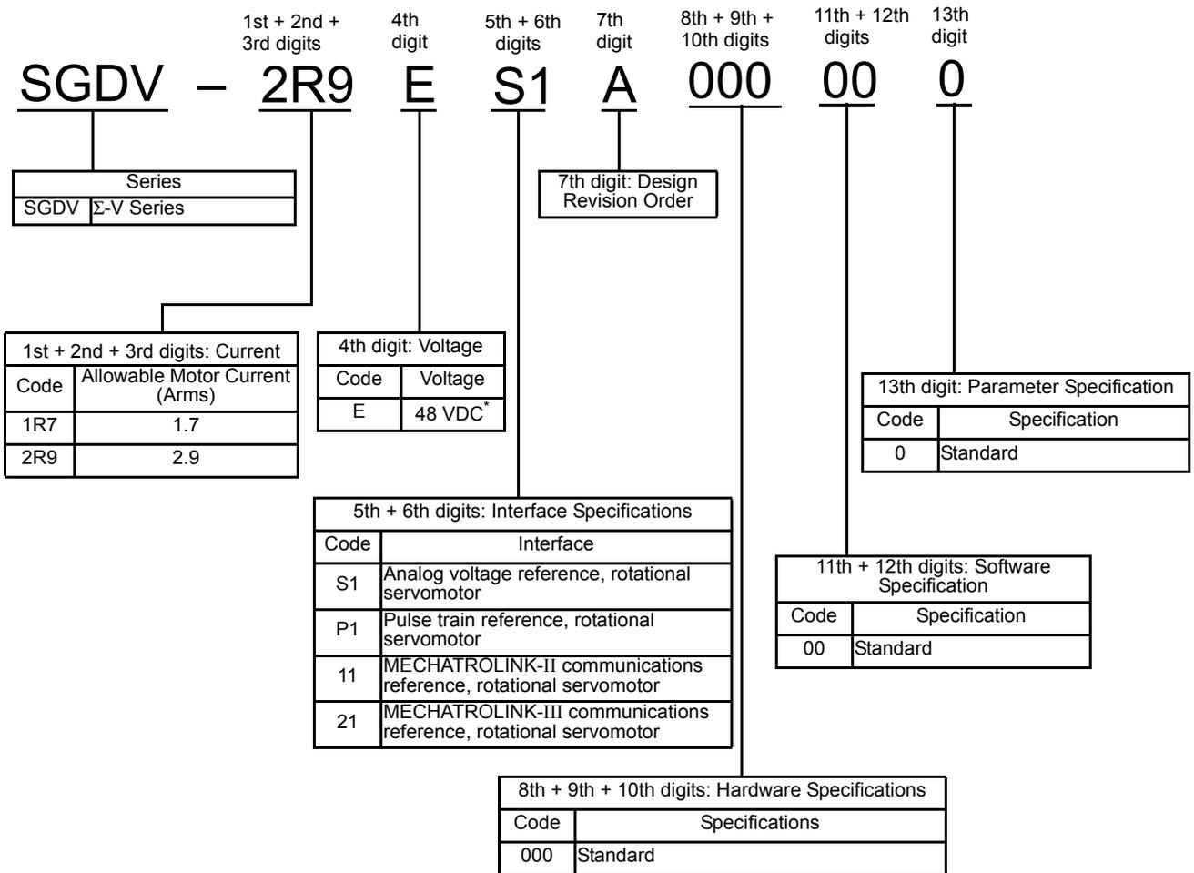
\* 24 VDC for the main circuit power supply also can be used.
