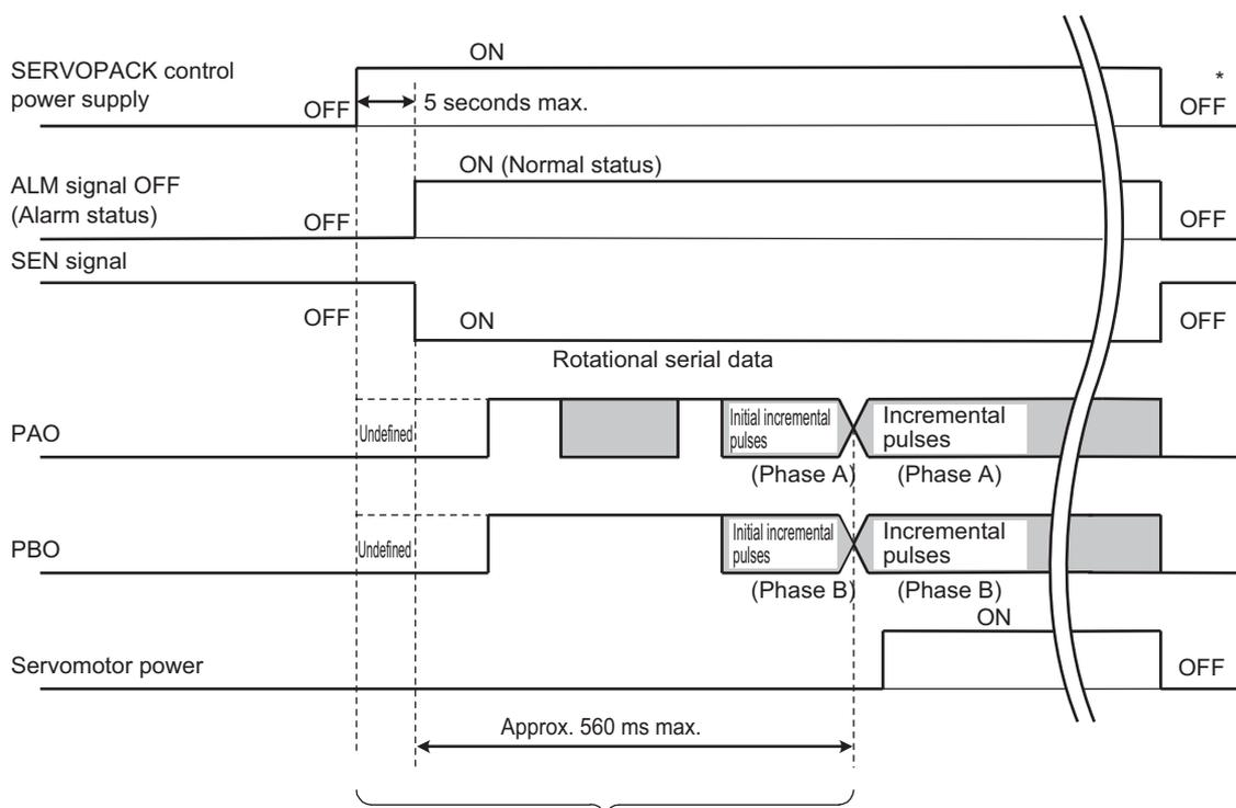
The servomotor will not be turned ON even if /S-ON is turned ON during this interval.
