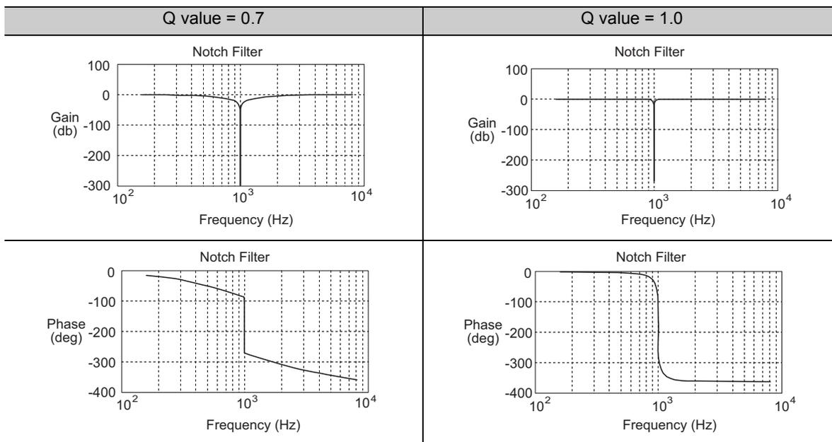
The notch filter can be enabled or disabled with Pn408.
