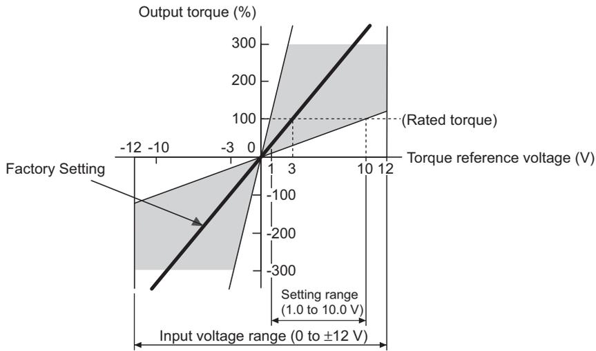
Note: A torque reference above the rated torque can be applied but it may cause an overload (high load) alarm (A.710) or overload (low load) alarm (A.720) if excessive torque is output for a long time. Refer to 9.1.2 *Troubleshooting of Alarms*.
