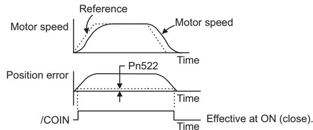
Note: If the parameter is set to a value that is too large, a positioning completed signal might be output if the position error is low during a low speed operation. This will cause the positioning completed signal to be output continuously. If this signal is output unexpectedly, reduce the set value until it is no longer output.
