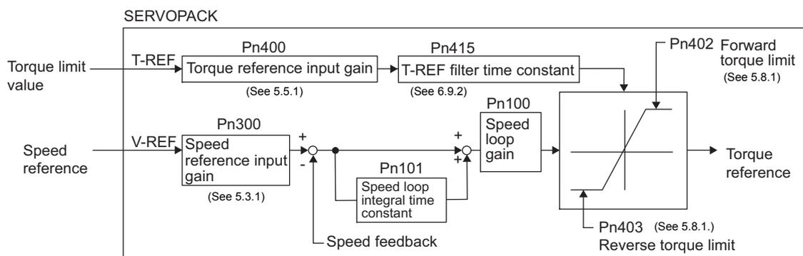
There is no polarity in the input voltage of the analog voltage reference for torque limiting. The absolute values of both + and - voltages are input, and a torque limit value corresponding to that absolute value is applied in the forward and reverse direction.
