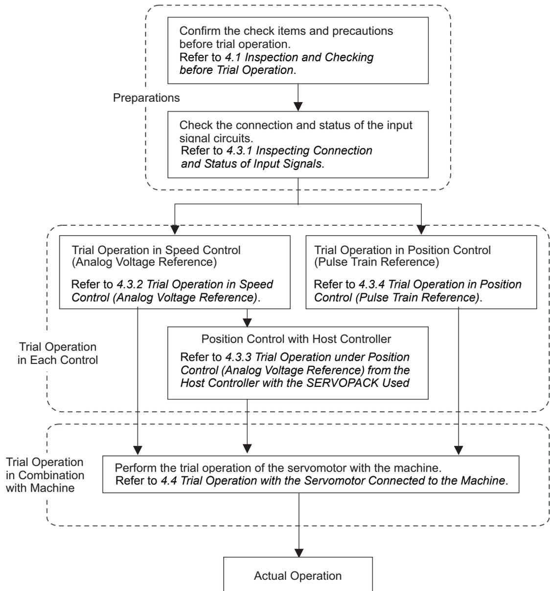
Note: To perform trial operation of a servomotor with a brake, refer to 4.5 Trial Operation of Servomotor with Brakes.
