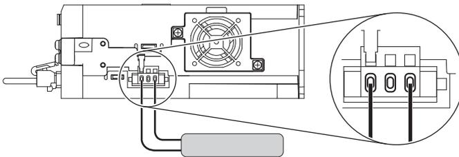
2. Set Pn601 (Dynamic Brake Resistor Allowable Energy Consumption) and Pn604 (Dynamic Brake Resistance).
