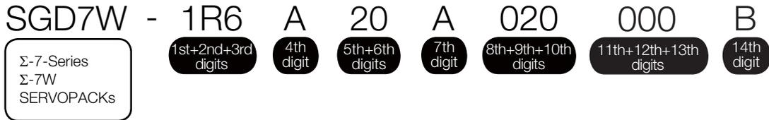
**1st+2nd+3rd digits** Maximum Applicable Motor Capacity per Axis
