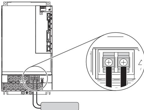
2. Set Pn601 (Dynamic Brake Resistor Allowable Energy Consumption) and Pn604 (Dynamic Brake Resistance).
