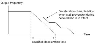
Figure 5.75 Stall Prevention Operation during Deceleration
