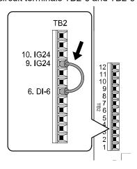
Figure 10.24 Self-Diagnostics Jumper Terminals
