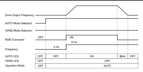
Figure 4.4 LEDs and Drive Operation in AUTO and HAND Modes
