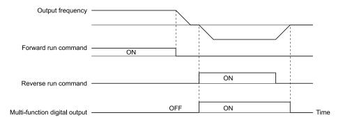
Figure 5.58 Reverse Operation Output Time Chart
