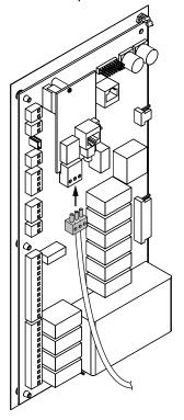
Figure 7.7 Connect Network Cable to Option (SI-W3 LonWorks Example)
