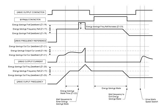
Figure 5.108 Drive Bypass Energy Savings Mode Sequence Example
