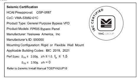
Figure 11.2 Seismic Certification Label Example for Bypasses
