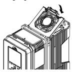
Figure 8.8 Install the Fan Finger Guard
