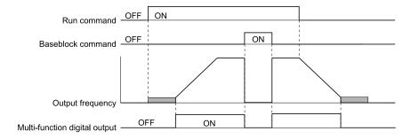
Figure 5.59 Active Frequency Output Time Chart
