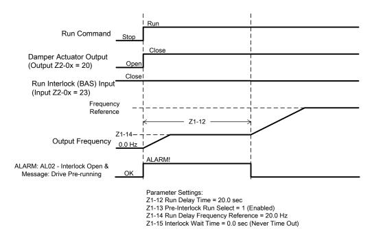
Figure 5.105 Run Delay with Preset Speed Example: Preset Speed
