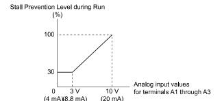
Figure 5.63 Stall Prevention Level during Run with Analog Input
