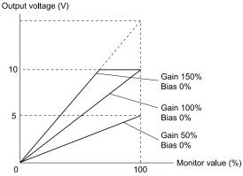
Figure 5.64 Analog Output Gain/Bias Configuration Example 1
