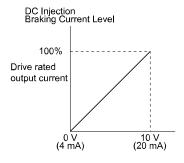
Figure 5.62 DC Injection Braking Current through Analog Input
