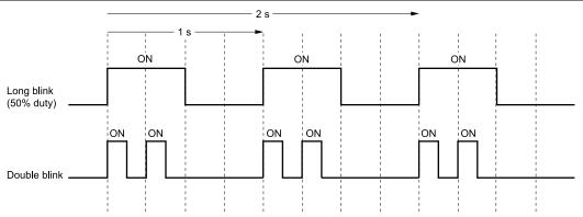
Figure 4.3 AUTO LED and HAND LED Timing Status
