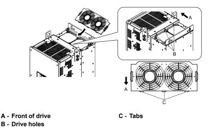
Figure 8.44 Install the Fan Finger Guard
