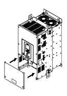
Figure 2.21 Reattach the Terminal Cover
