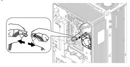
Figure 8.34 Disconnect the Connector
