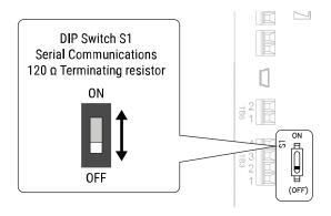
Figure 10.12 Termination Resistor DIP Switch S1
