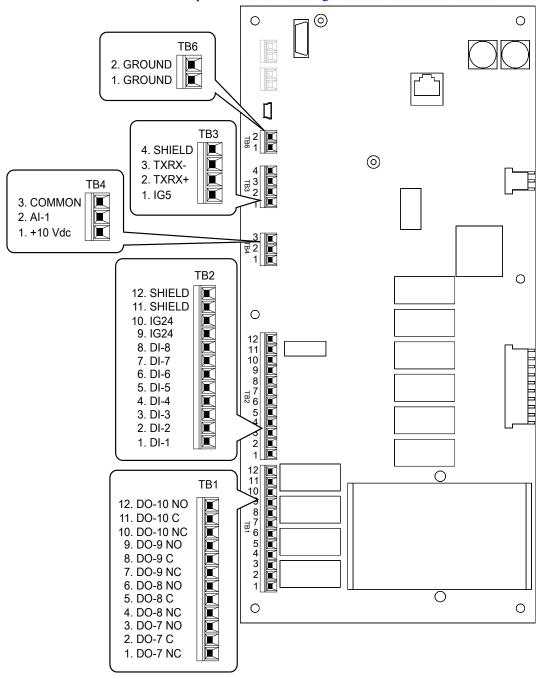
Figure 3.6 Bypass Control Circuit Terminal Arrangement
