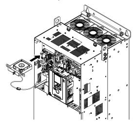
Figure 8.60 Install the Fan Unit
