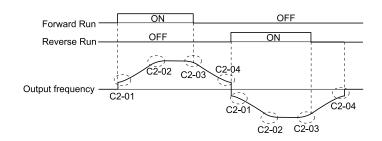
Figure 5.31 S-Curve Timing Diagram - Forward/Reverse Operation
