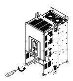
Figure 2.16 Loosen the Front Cover Screws
