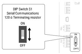
Figure 10.3 Termination Resistor DIP Switch S1
