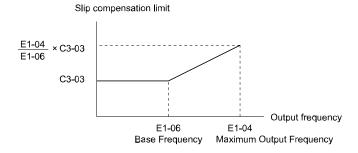
Figure 5.32 Slip Compensation Limit
