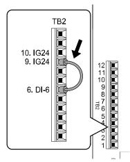
Figure 10.16 Self-Diagnostics Jumper Terminals
