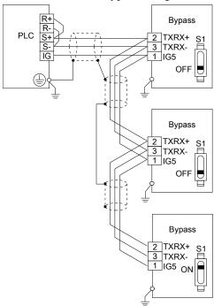
Figure 10.13 Wiring Diagram for More than One Bypass
