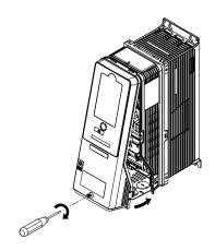
Figure 2.12 Reattach the Front Cover
