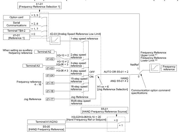
Figure 5.34 Frequency Reference Setting Hierarchy
