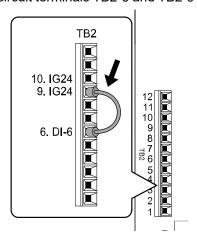
Figure 10.5 Self-Diagnostics Jumper Terminals
