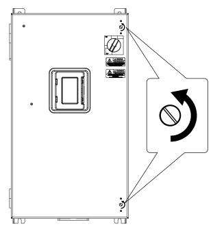
Figure 2.8 Turn the Screw Fasteners
