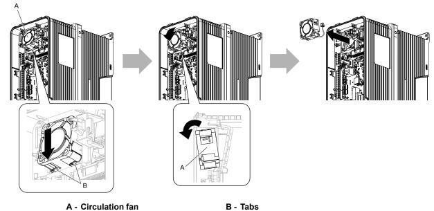
Figure 8.10 Remove the Circulation Fan
