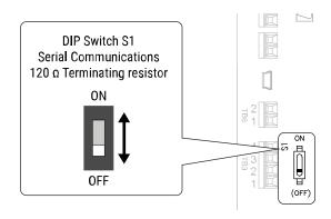
Figure 10.7 Termination Resistor DIP Switch S1
