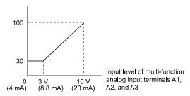
Figure 5.76 Stall Prevention Level during Run with Analog Input
