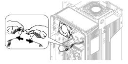
Figure 8.21 Disconnect the Power Supply Connector
