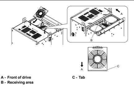
Figure 8.51 Install the Fan Finger Guard
