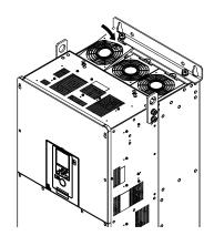
Figure 8.52 Install the Fan Finger Guard
