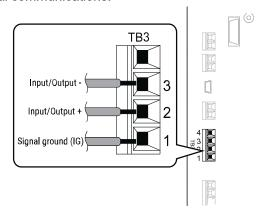
Figure 10.6 Communications Cable Connection Terminal (TB3)
