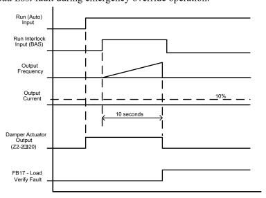
Figure 5.109 Motor Disconnected at Start
