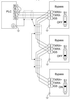
Figure 10.20 Wiring Diagram for More than One Bypass
