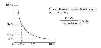
Figure 5.61 Acceleration/Deceleration Time Gain through Analog Input
