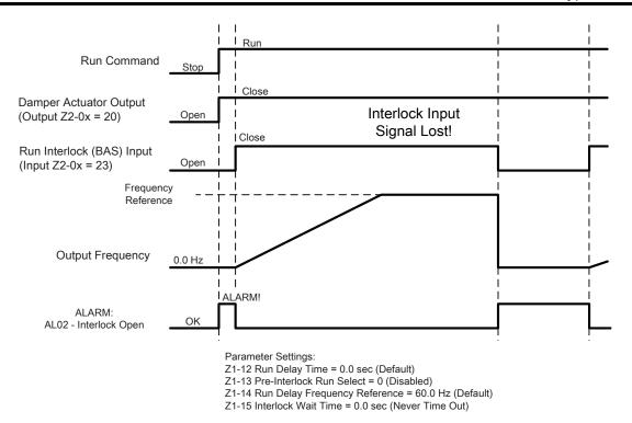
Figure 5.104 Run Interlock Lost Example: Default Settings
