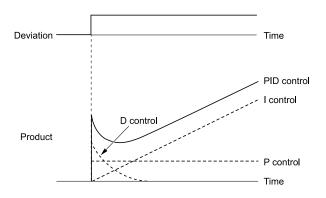
Figure 5.22 PID Control Operation
