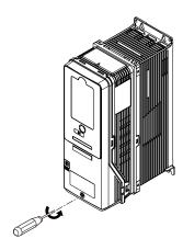
Figure 2.10 Loosen the Front Cover Screw
