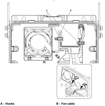
Figure 8.26 Put the Cables Back into the Drive
