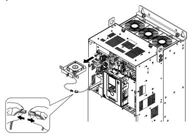
Figure 8.55 Remove the Fan Unit
