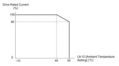
**Figure 7.4 Derating for IP55/UL Type 12 (L8-35 = 3)**
