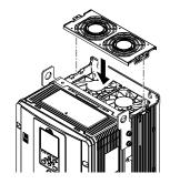
Figure 8.32 Install the Fan Finger Guard
