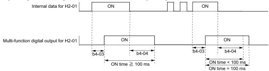
Figure 5.21 Example of How the Timer Function Works with H2-01 Terminals
