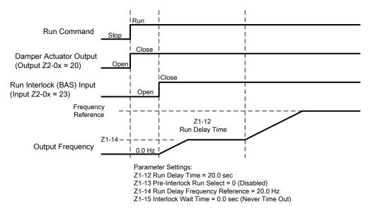
Figure 5.107 Run Delay with Preset Speed Example: Preset Speed with Run Delay
