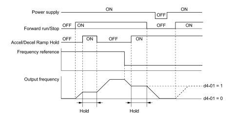
Figure 5.38 Frequency Reference Hold with Accel/Decel Hold Function
