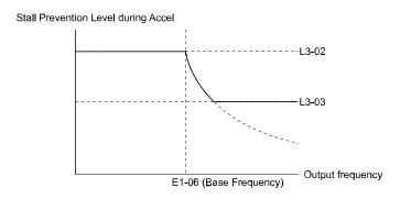
Figure 5.74 Stall Prevent Level during Accel/Limit
