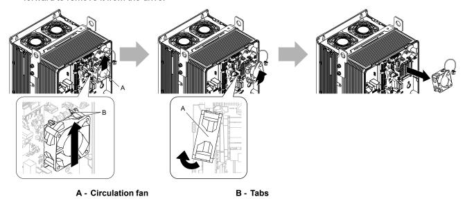
Figure 8.35 Remove the Circulation Fan
