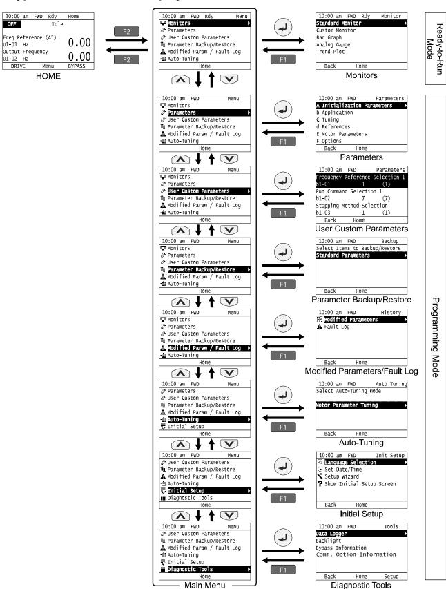
Figure 4.5 Keypad Functions and Display Levels
