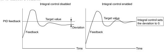
Figure 5.25 Integral Time and Deviation
