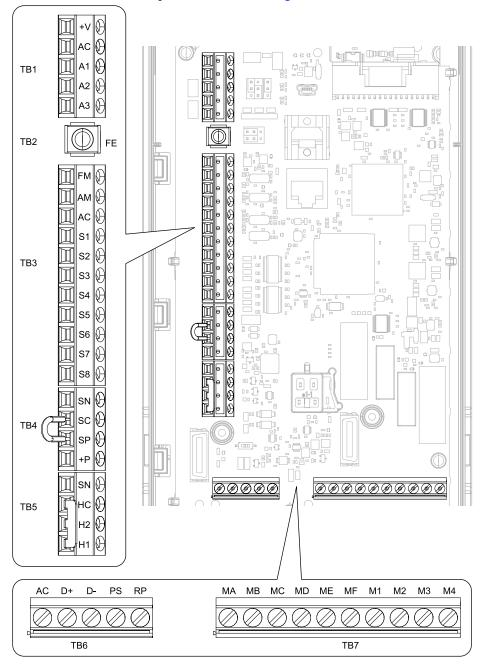
**Figure 3.11 Control Circuit Terminal Arrangement**
