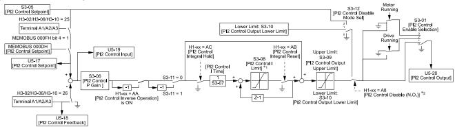
Figure 5.94 PI2 Control Block Diagram
