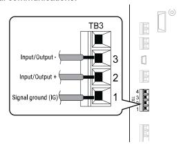
Figure 10.11 Communications Cable Connection Terminal (TB3)
