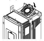
Figure 8.19 Install the Fan Finger Guard
