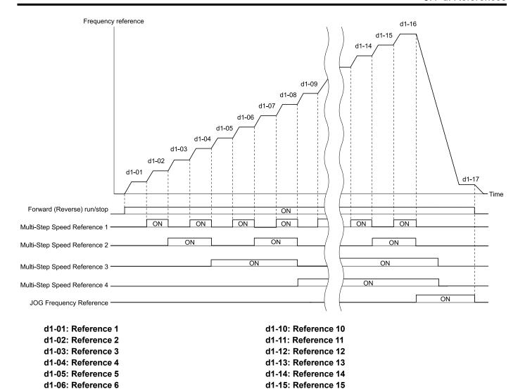
Figure 5.35 Time Chart for Multi-step Speed Reference/JOG Reference
