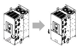
Figure 2.13 Loosen the Terminal Cover Mounting Screws
