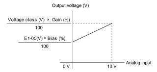
Figure 5.60 Output Voltage Bias through Analog Input
