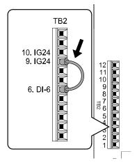
Figure 10.9 Self-Diagnostics Jumper Terminals
