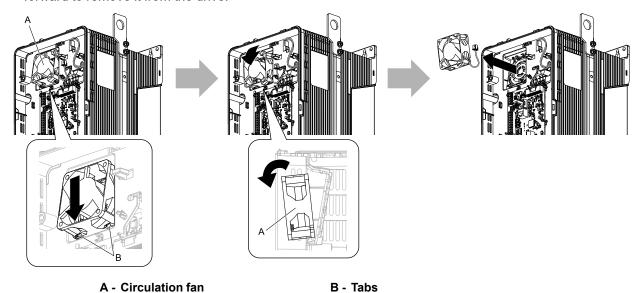
Figure 8.22 Remove the Circulation Fan
