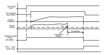
Figure 5.110 Motor Disconnected during Run
