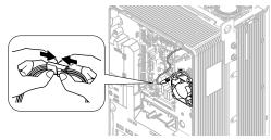
Figure 8.37 Connect the Power Supply Connector
