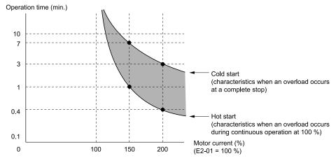
Figure 5.72 Protection Operation Time for a General-purpose Motor at Rated Output Frequency
