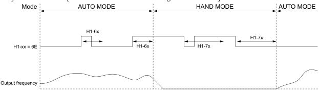
Figure 5.41 Example of ON-Delay and OFF-Delay Timers
