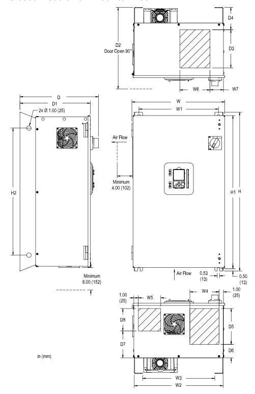
Figure 2.22 Enclosed Exterior and Mounting Dimensions Diagram
