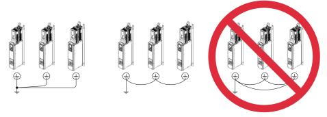
Figure 3.3 Wiring More than One Bypass
