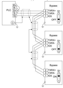
Figure 10.8 Wiring Diagram for More than One Bypass
