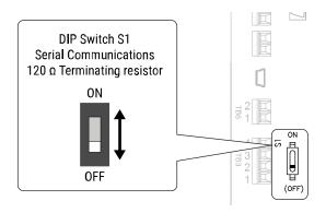
Figure 10.19 Termination Resistor DIP Switch S1
