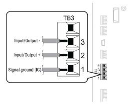
Figure 10.2 Communications Cable Connection Terminal (TB3)
