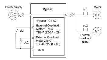
Figure 5.71 Protection Circuit Configuration to Connect More than One Motor to One Drive
