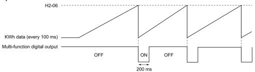
Figure 5.47 Example MFDO when Configured for Watt Hours
