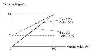
Figure 5.65 Analog Output Gain/Bias Configuration Example 2
