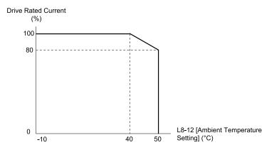
Figure 7.2 Derating for Side-by-Side Mounting (L8-35 = 1)
