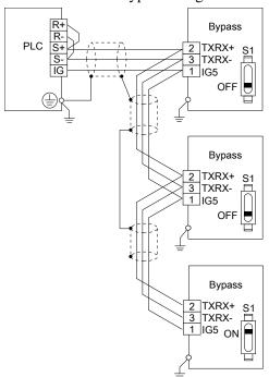
Figure 10.4 Wiring Diagram for More than One Bypass
