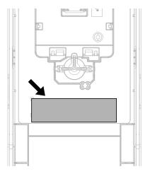
Figure 3.12 Tightening Torque Display Location (Reverse Side of Drive Front Cover)
