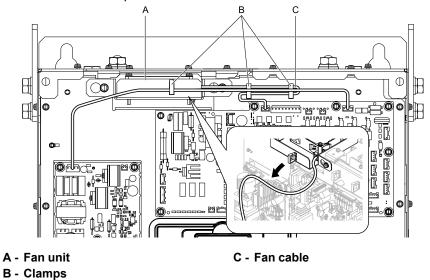
Figure 8.53 Remove the Fan Cables
