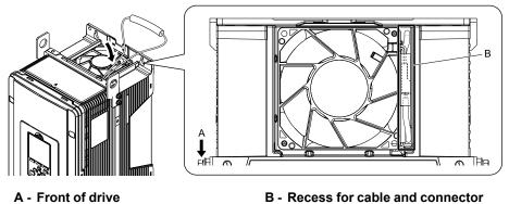
Figure 8.17 Put the Cable in the Drive Recess
