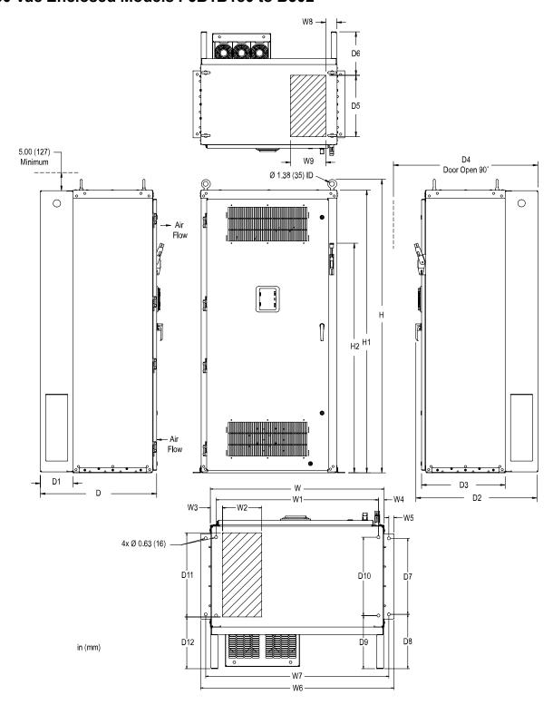
Figure 2.23 Enclosed Exterior and Mounting Dimensions Diagram
