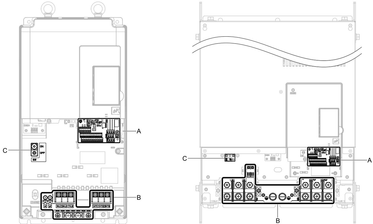
**A** – Terminal board (*Refer to Control Circuit Wiring on page 64*)
