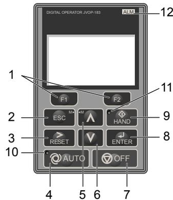
Figure 4.1 Description of HOA Keypad Keys and Displays
