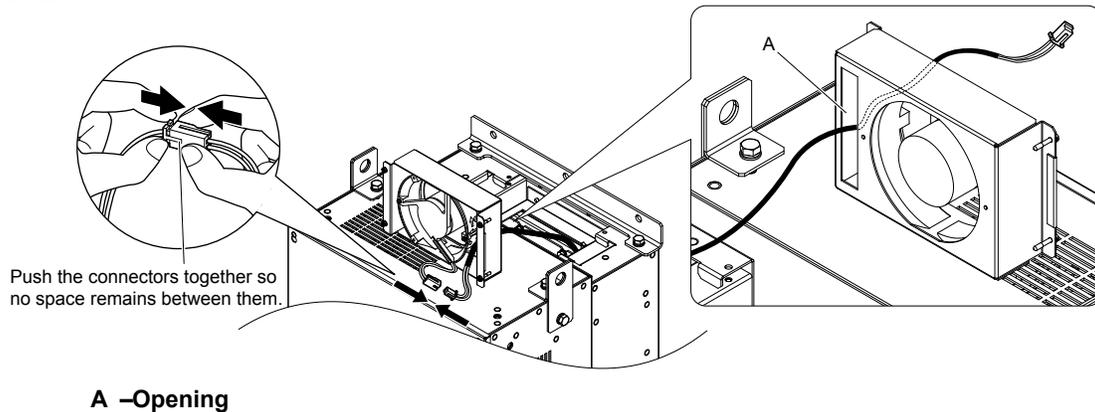
Figure 7.27 Attach the Relay Connector
