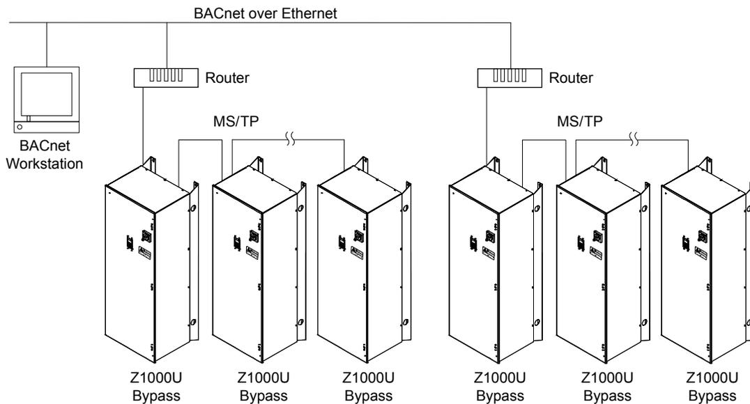
**Figure C.1 Connecting Multiple Bypasses to a BACnet Workstation**
