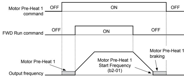
Figure 5.19 Motor Pre-Heat 1 Input Timing Diagram
