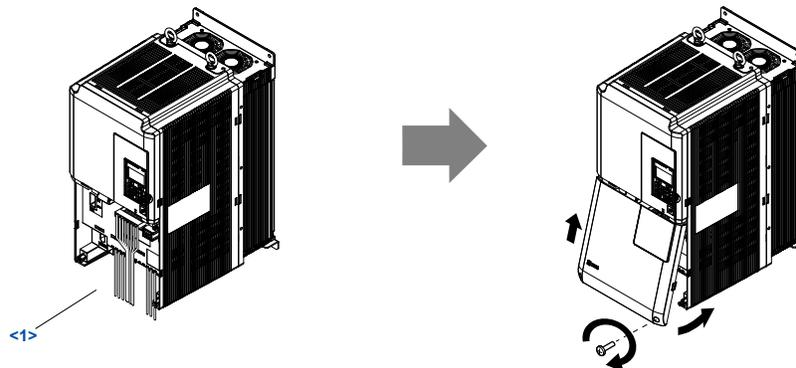
Figure 3.23 Reattaching the Terminal Cover
