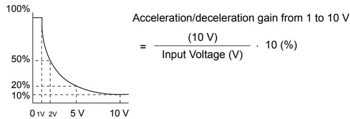
Figure 5.34 Accel/Decel Time Gain with Analog Input Terminal
