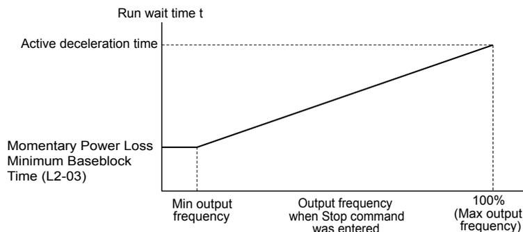
**Figure 5.5 Run Wait Time Depending on Output Frequency**
