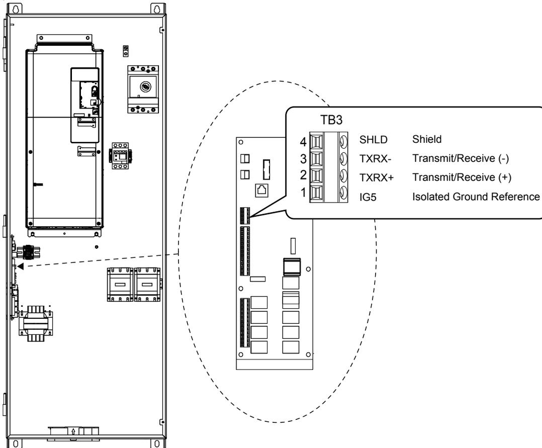
Figure C.2 Serial Communications Cable Connection Terminal (TB3)
