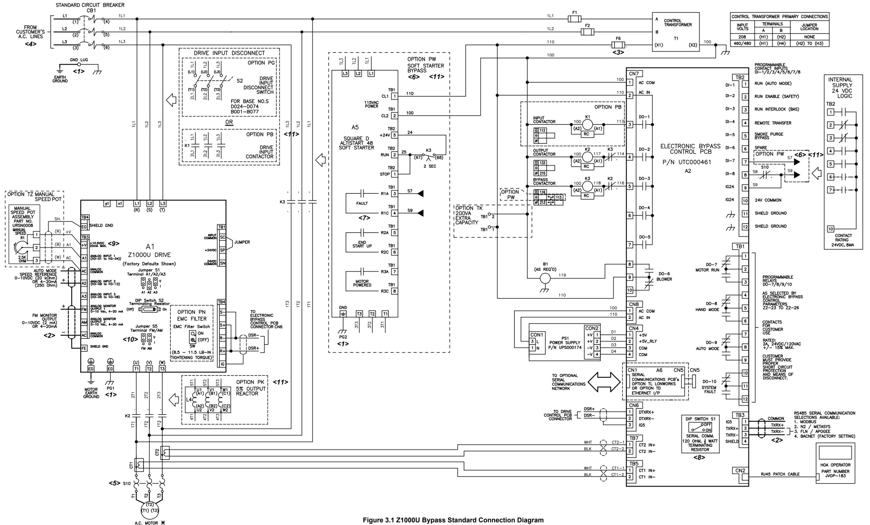
Figure 3.1 Z1000U Bypass Standard Connection Diagram
