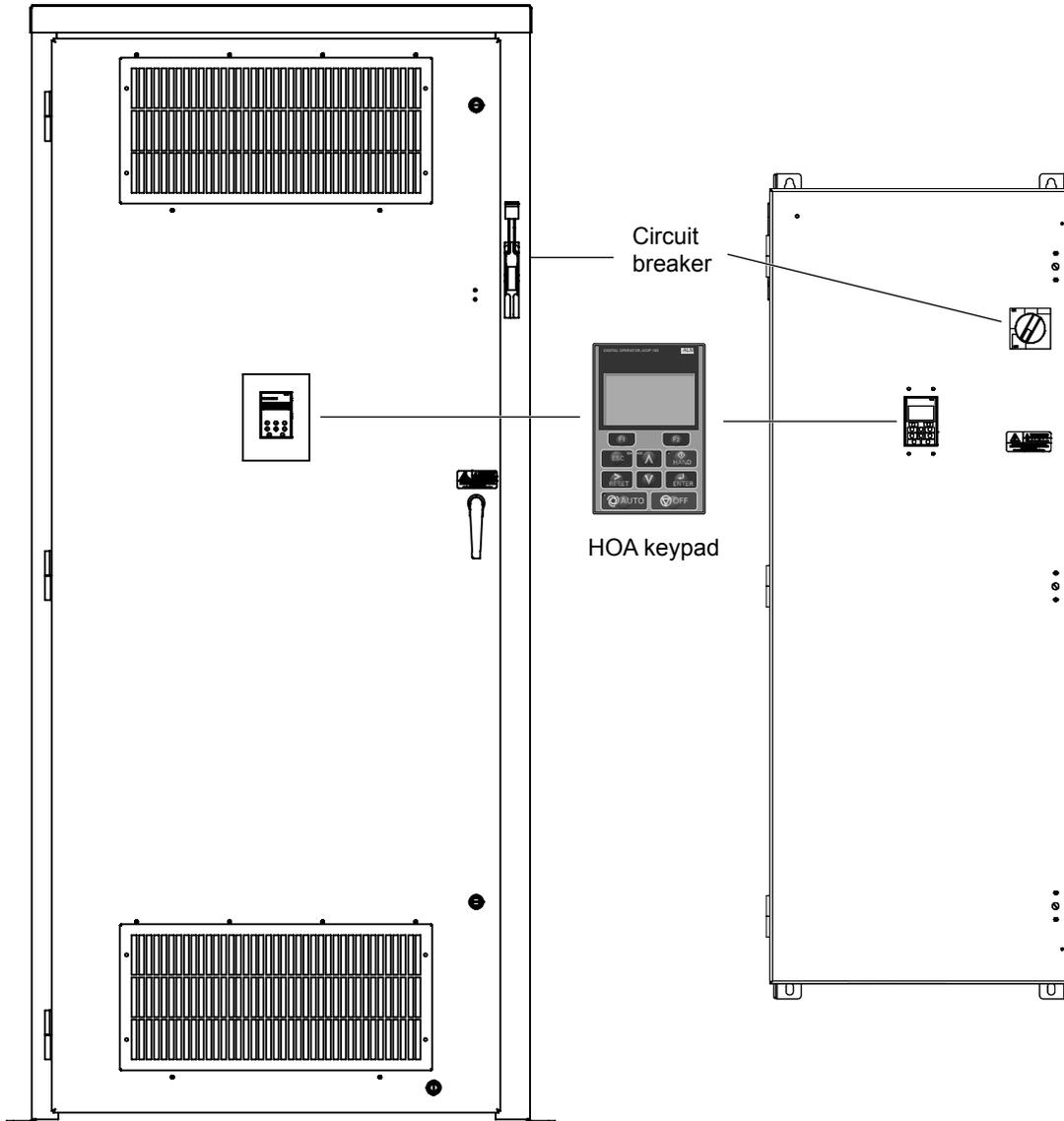
Figure 1.5 Bypass Control Panel with Keypad Operator Controls
