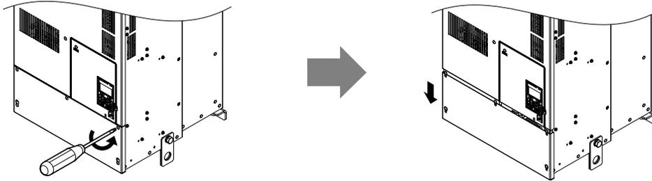
Figure 3.24 Removing the Terminal Cover
