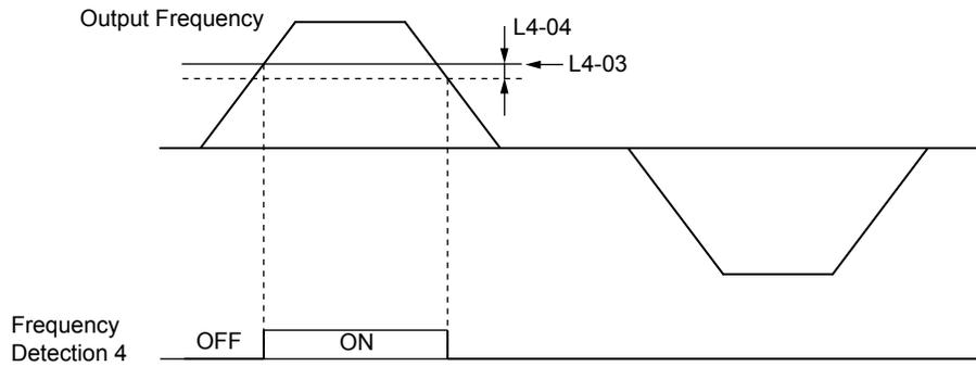
Figure 5.29 Frequency Detection 4 Example with Positive L3-04 Value
