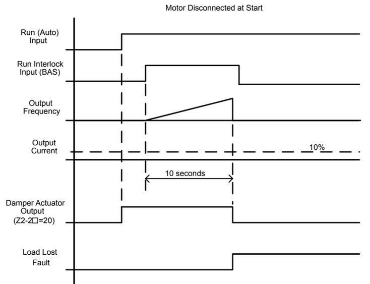
Figure 5.59 Motor Disconnected at Start
