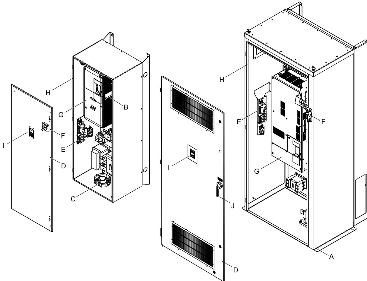
**A – Bypass bracket mounting hole**
