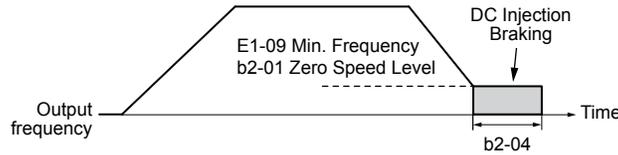
Figure 5.6 DC Injection Braking at Stop for V/f
