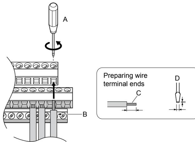
A – Loosen screw to insert wire.
