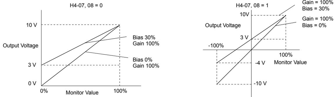
Figure 5.38 Analog Output Gain and Bias Setting Example 3
