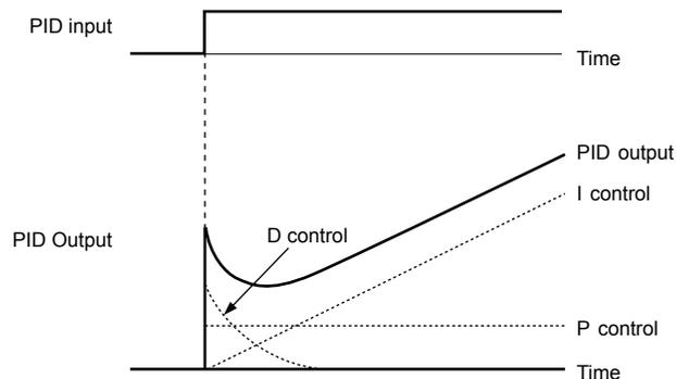
Figure 5.10 PID Operation
