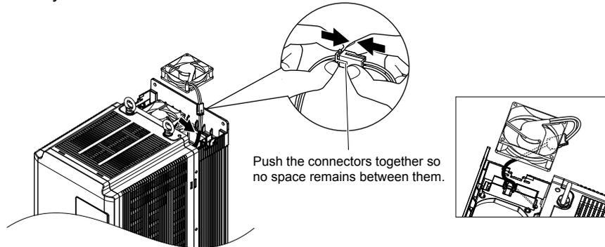
Figure 7.6 Plug the Relay Connector
