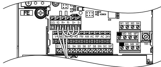
Figure 3.32 Terminal Board Location Inside the Drive
