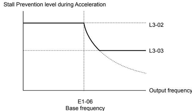
Figure 5.41 Stall Prevention Level and Limit During Acceleration
