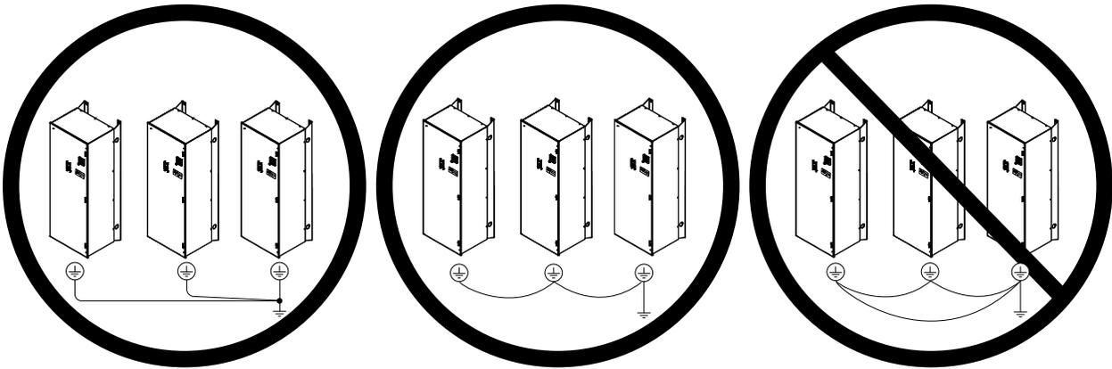
Figure 3.9 Ground Wiring for Multiple Bypass Units
