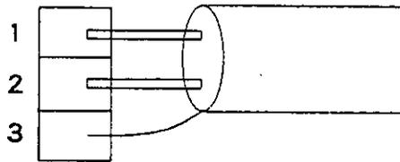
Shielded Twisted-pair Cable Connection
