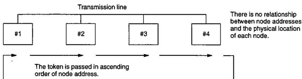
2) MEMOBUS PLUS devices have communications processors to control various network transmissions. These processors perform functions such as rotating tokens, sending/receiving messages, acknowledging reception, etc.
