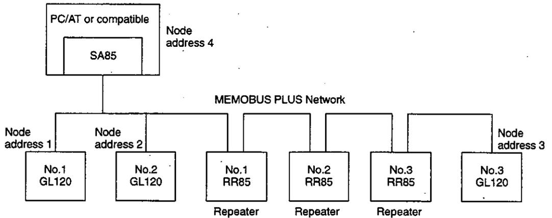
\*Up to 3 Repeaters can be used in a single network.
