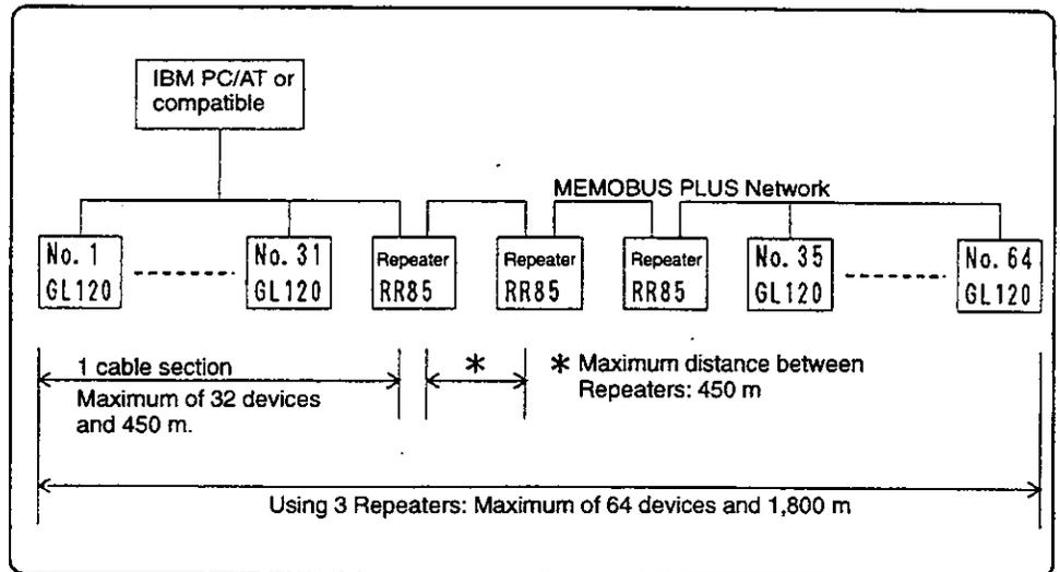
**Note** Computers connected to the MEMOBUS PLUS Network must be equipped with an SA85 Network Adapter.
