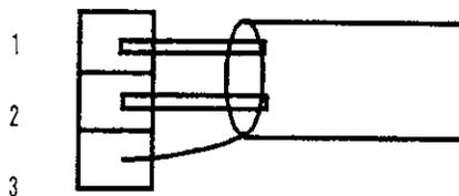
Shielded Twisted-pair Cable Connection
