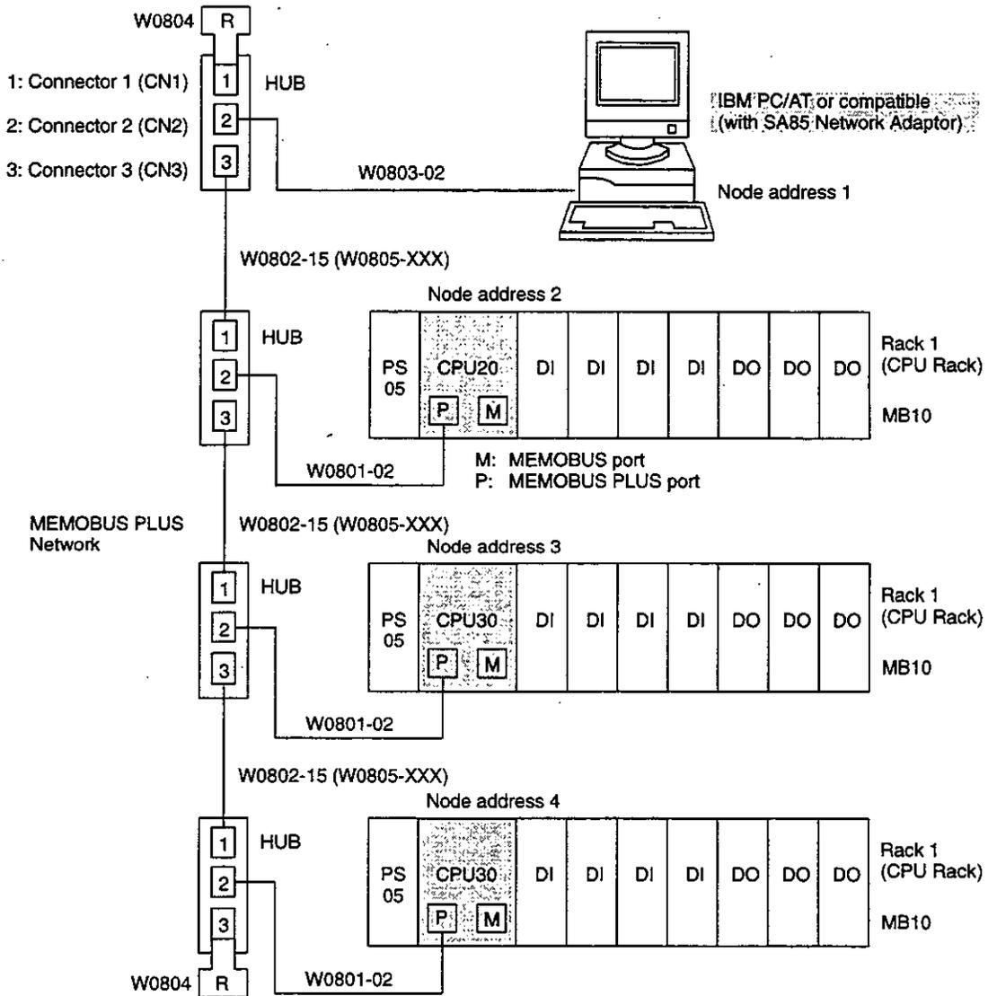
PS05: AC Input Power Supply Module (3 A)
