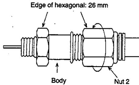
**Note** Fully insert the body and tighten nut 2.
