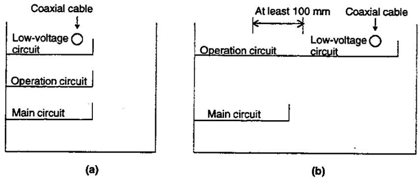
Figure 6.2 Separating Wire Ducts
