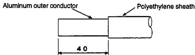
b) Remove the aluminum outer conductor and insulating material to 15 mm from the cable end.
