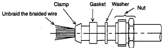
**Note** a) Place the nut, washer, and gasket over the sheath.
