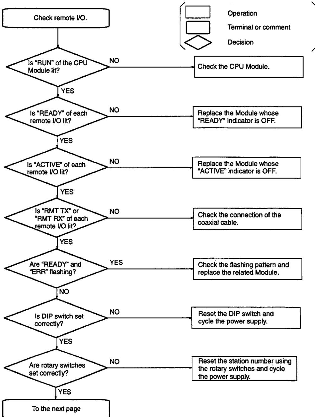
7.2.2 Fault Checking Procedure cont.
