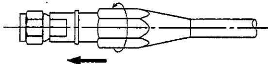
**Note** Fix the body with a wrench or an adjustable spanner (12 mm width across flat) and turn the nut for tightening with a wrench or an adjustable spanner (14 mm width across flat).
