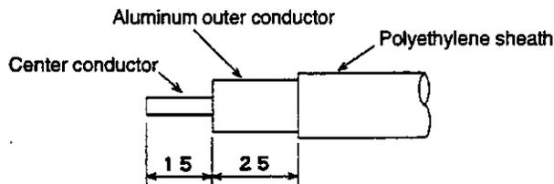
**Note** Be careful not to bend or damage the center conductor.
