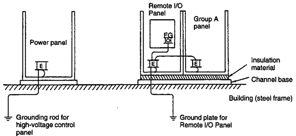
Figure 6.7 Remote I/O Panel Insulation
