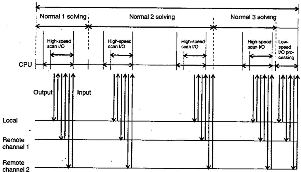
c) Remote I/O Station I/O Timing
