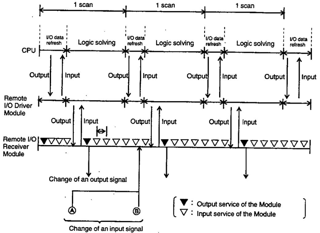
a) The input servicing of the Remote I/O Receiver Modules varies depending on the number of Input Modules; however, scanning occurs between 1 ms to 7 ms.
