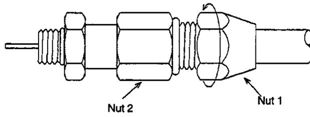
**Note** Secure nut 2, then turn to tighten nut 1.
