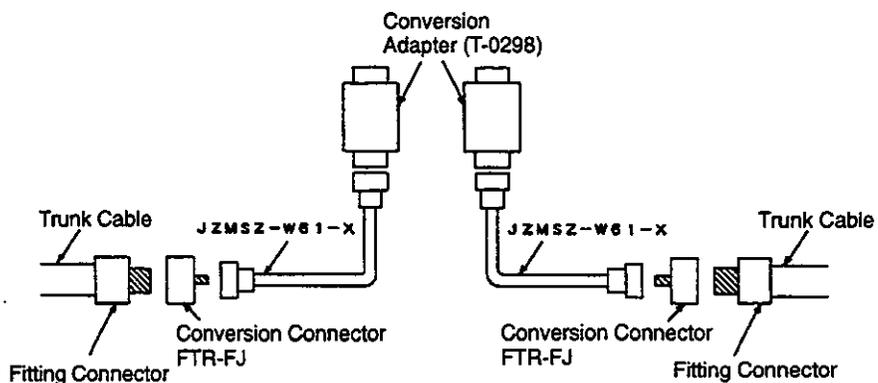
c) Connecting between Coaxial Cables
