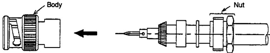
**Note** Insert the contact into the body to the end.
