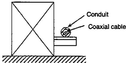
Construction on ground (with iron frames)
