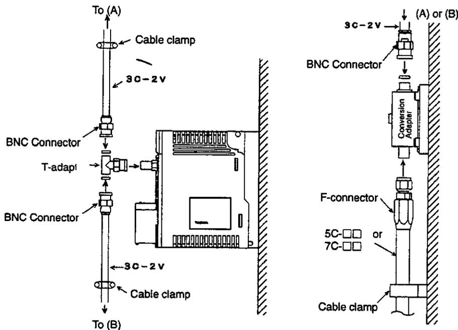
Figure 6.1 Device Connections
