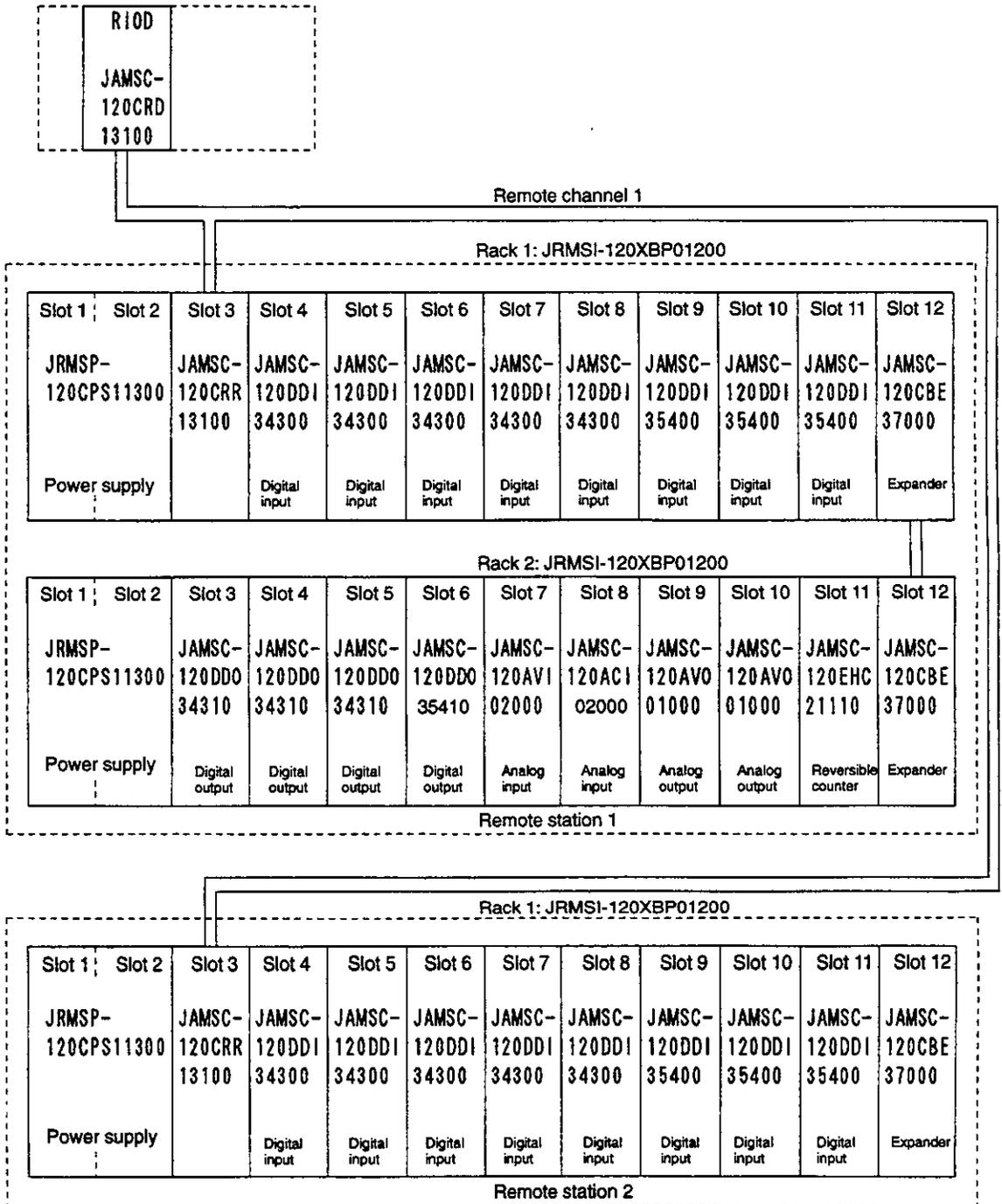
Figure 2.6 Example of I/O Module Layout
