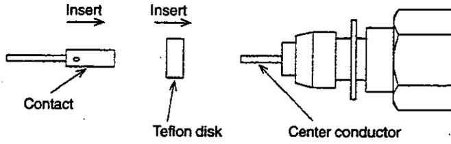
5) Press to bond the contact, using 9.5 mm coaxial-cable press-pliers.
