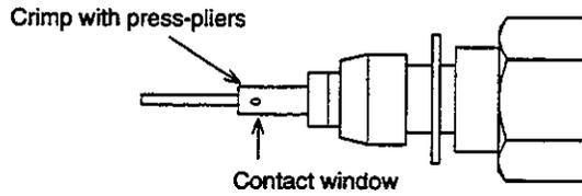
**Note** Check through the contact window to make sure that the contact is inserted.
