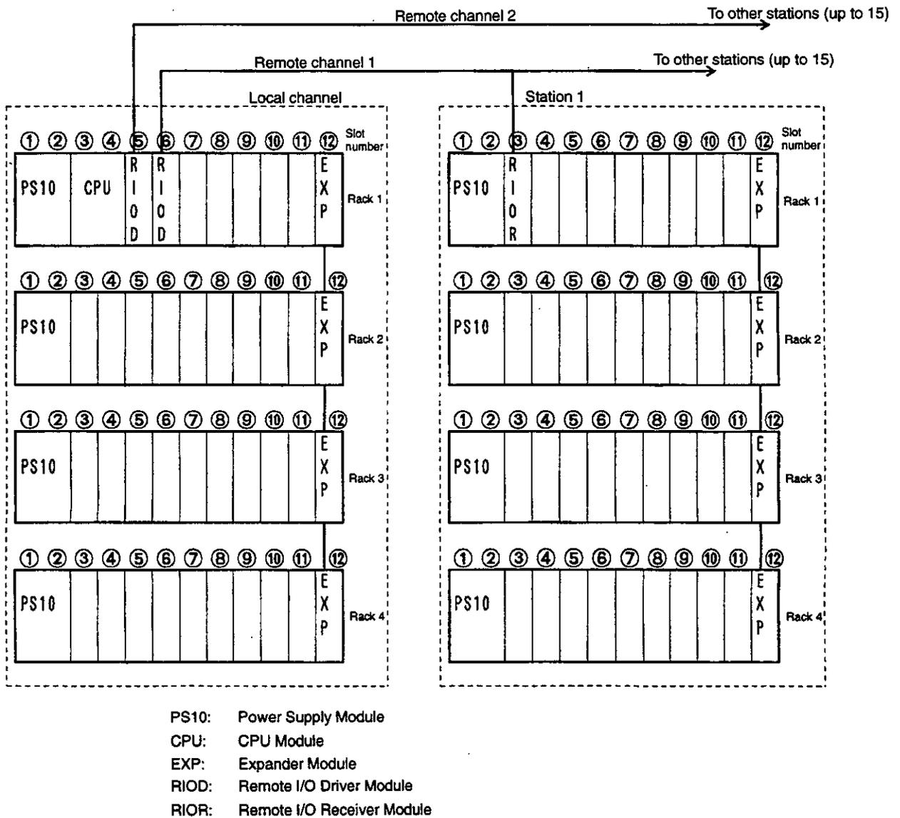
Figure 2.1 System Configuration Diagram
