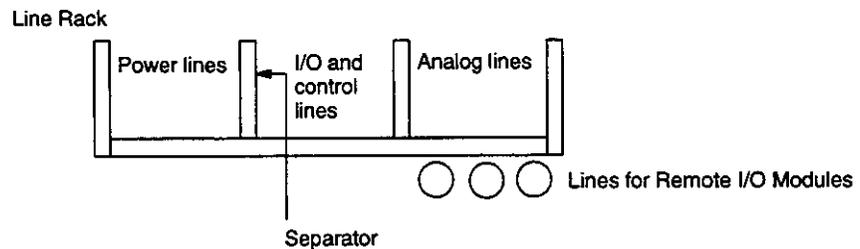
When wiring Remote I/O Module cables outside of the control panel, place them in a duct or conduit by themselves to minimize the affects of noise. Faulty operation can result if MEMOBUS lines are not sufficiently insulated.
