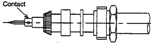
**Note** a) Solder quickly, being careful not to deform the insulating material.
