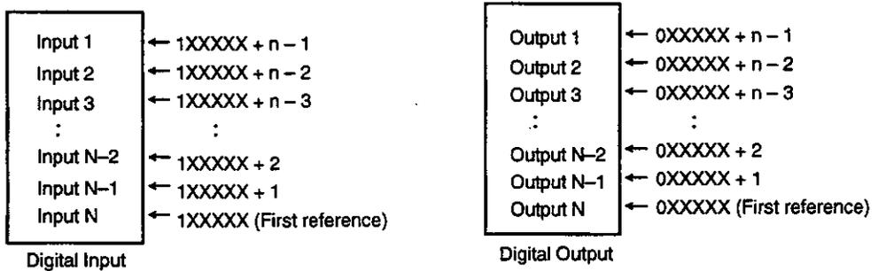
Figure 2.4 Digital I/O Data Format with Bit Sequence Specification = LSB
