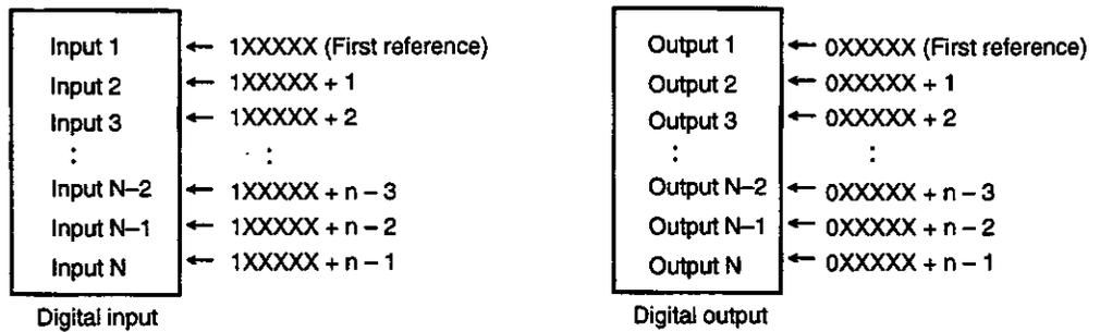
Figure 2.3 Digital I/O Data Format with Bit Sequence Specification = MSB
