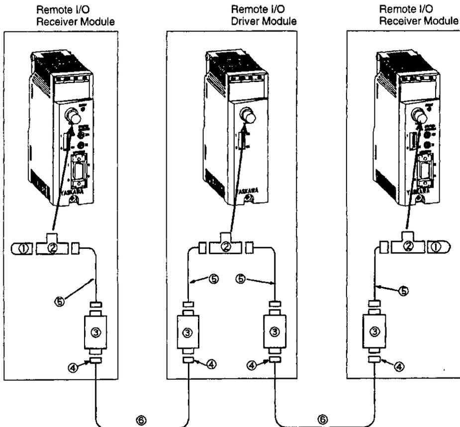
c) Remote I/O Driver and Receiver Modules Installed in Same Panel
