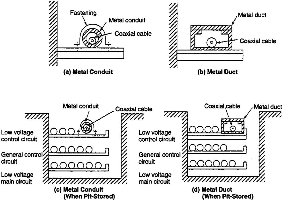
Figure 6.3 Coaxial Cable Installation
