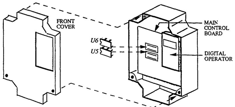
Figure 1. Installation of HVAC EPROM Set in GPD 503
