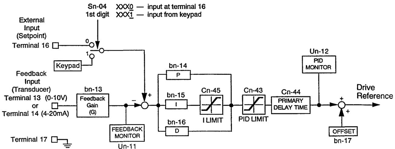
Figure 3. HVAC Software – PID Control Block Diagram
