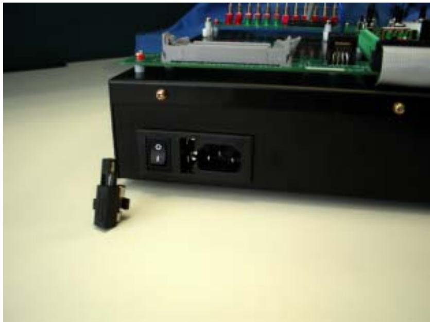
Figure 6: Power entry module with on/off switch and spare fuse inserts
