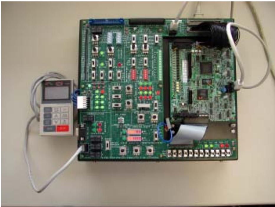
**Figure 2: Simulator with G7 control card installed and running under simulated load**
