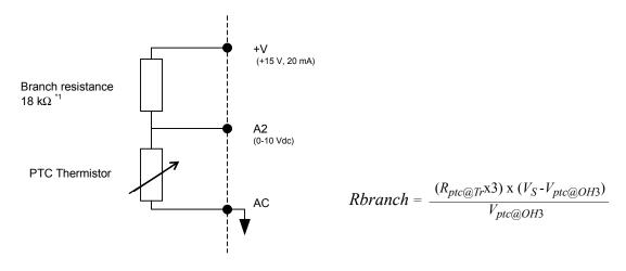
\*1 The resistance value of 18 k $\Omega$  is only valid for using a 3-phase PTC with the characteristics shown in the figure above.
