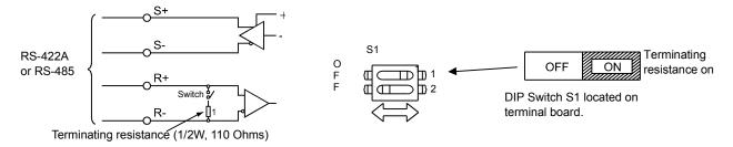
Fig. 63 Communication Connection Terminals and Terminating Resistance
