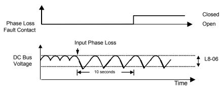
Fig. 83 Input Phase Loss Detection Diagram
