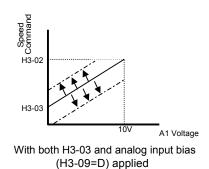
Fig. 55 Frequency Bias 2 Applied to Analog Speed Command
