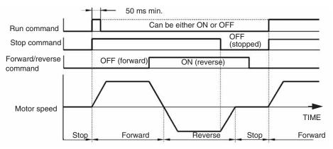
Fig. 31 3-Wire Control Timing Diagram
