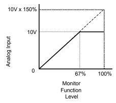
Fig. 60 Analog Output gain Setting Adjustment
