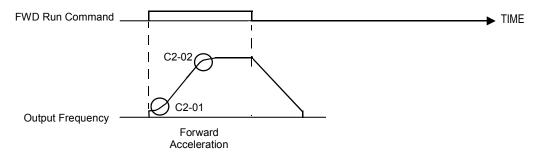
Fig. 23 S-Curve Characteristic Timing Diagram
