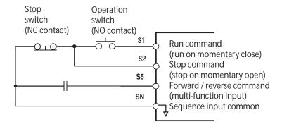
Fig. 30 Terminal Configuration for 3-Wire Control
