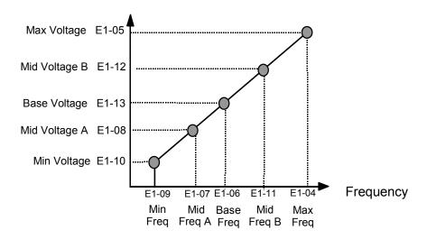
Fig. 29 Custom V/f Pattern Programming Curve
