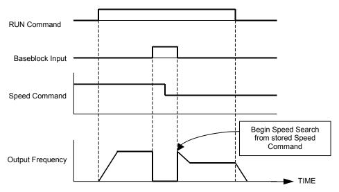
Fig. 33 External Baseblock Characteristics
