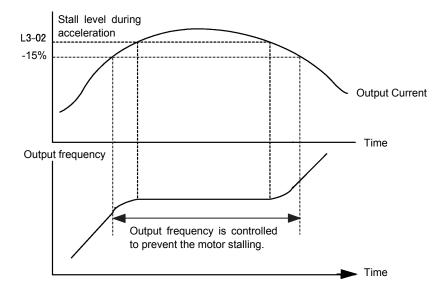
Fig. 75 Detailed Time Chart for Stall Prevention During Acceleration
