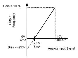
Fig. 50 Output Frequency with Reduced Bias Setting
