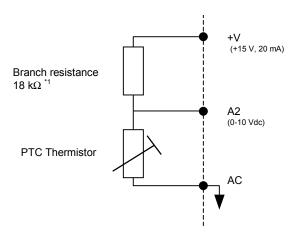
\*1 The resistance value of 18 k $\Omega$  is only valid for using a 3-phase PTC with the characteristics shown in the figure on following page.
