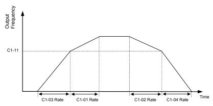
Fig. 21 Accel/Decel Switch Frequency Operation
