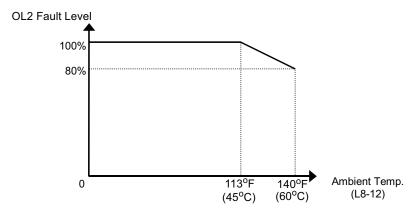
Fig. 85 Ambient Temperature Derating Curve
