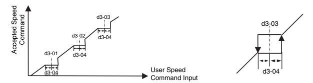
Fig. 27 Jump Frequency Characteristics
