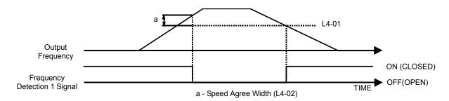
Fig. 42 Freq Detect 1 Timing Diagram
