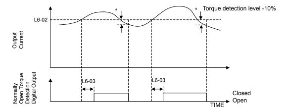
\* When the output current drops below the Torque Detection Level by approximately 10% of the Drive's rated output current the digital output is reset.
