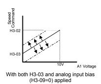
Fig. 54 Frequency Bias Applied to Analog Speed Command
