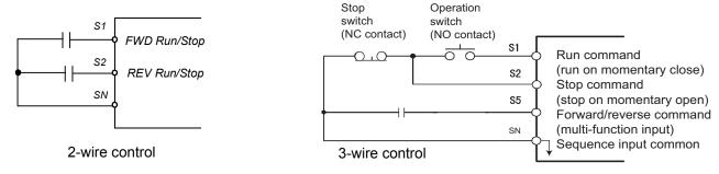
Fig. 1 2 & 3-Wire Control Wiring Examples
