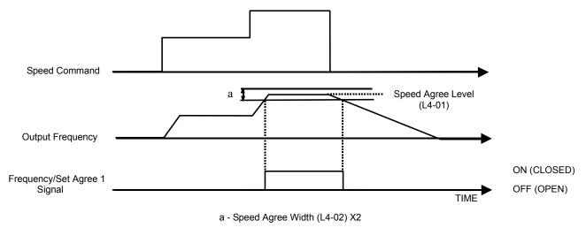
Fig. 41 Fref/Set Agree 1 Timing Diagram
