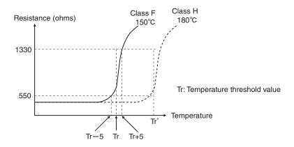
Fig. 74 PTC Thermistor Temperature-Resistance Value Characteristics
