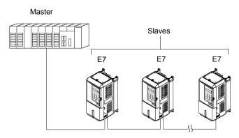
Fig. 62 Example of Connections between Master and Drive
