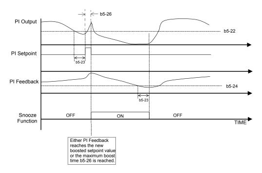
Fig. 20 Snooze Function Operation
