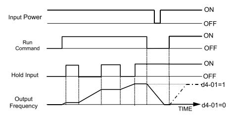
Fig. 34 Accel/Dec RampHold Function Timing Diagram
