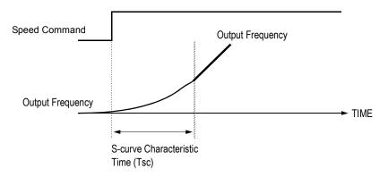
Fig. 22 S-curve Characteristic Timing Diagram
