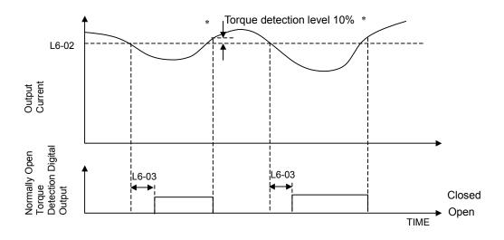
Fig. 81 Over Torque Detection
