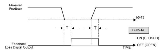
Fig. 18 Loss of PI Feedback Feature
