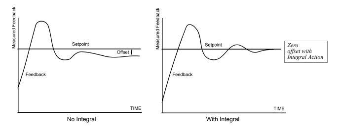
Fig. 17 PID Feedback Response Characteristics
