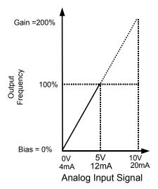
Fig. 49 Output Frequency as Commanded via Analog Input with Increased Gain Setting
