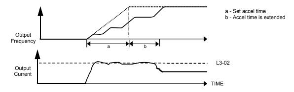
Fig. 76 Time Chart for Stall Prevention During Acceleration
