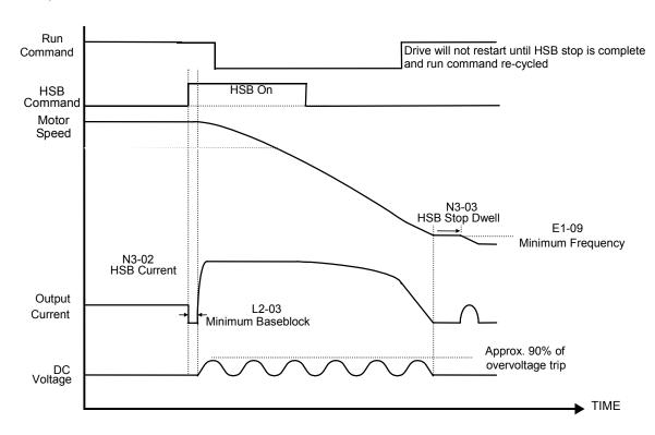
Fig. 86 High Slip Braking Timing Diagram
