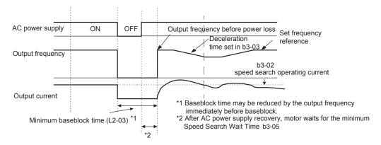
Fig. 13 Speed Search (Current Detection Method) after momentary power loss where the power loss time is less than the minimum baseblock time
