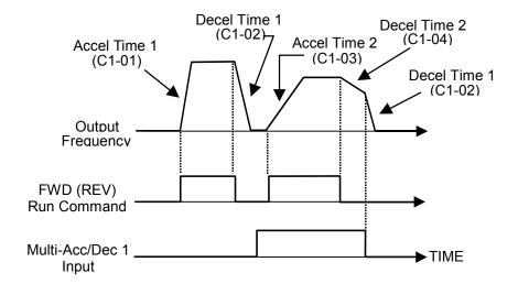
Fig. 32 Multi-Accel/Dec Timing Diagram
