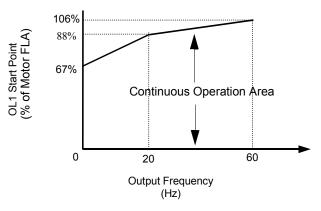
Fig. 71 Motor Overload Protection Curve
