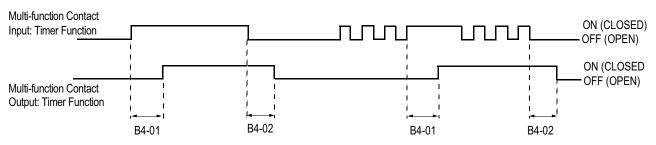
Fig. 15 Timing Diagram of Timer Function
