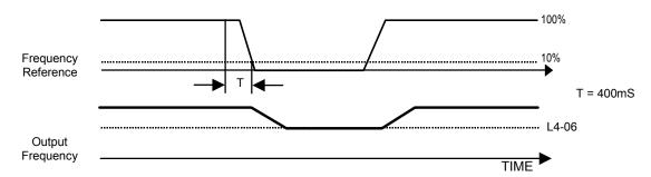
Fig. 79 Loss of Frequency Reference Timing Diagram
