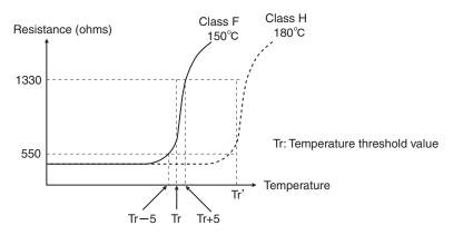
Fig. 56 PTC Thermistor Temperature-Resistance Value Characteristics
