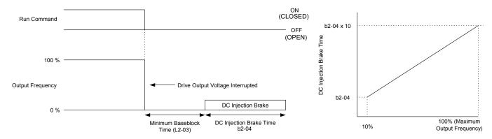
Fig. 6 DC Injection Braking to Stop
