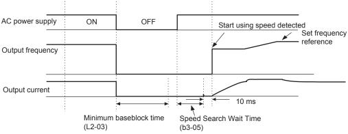
Note: If the frequency immediately before the baseblock is low or the power supply off time is long, operation may be the same as the search in case 1.
