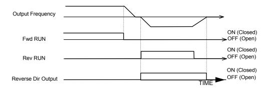
Fig. 47 Reverse Direction Timing Diagram
