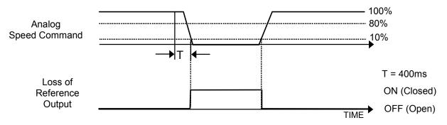
Fig. 45 Loss of Reference Function Characteristics
