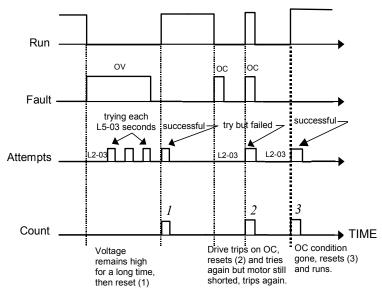
Fig. 80 Automatic Restart Timing Diagram
