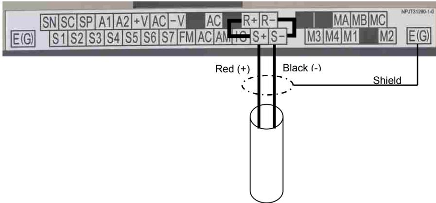
Figure 2.2 – Metasys N2 Network Cable Connections
