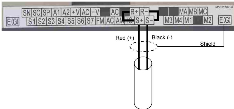
Figure A.1 – E7 Metasys N2 Network Connections
