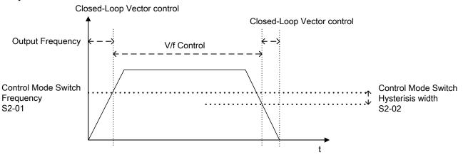
The following parameters are configurable only when A1-02 = 3 [Control Method Selection = Closed Loop Vector Control].
