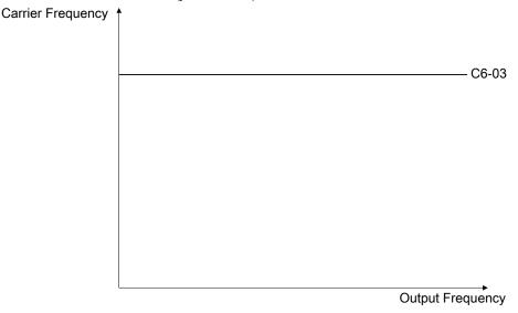
The figure below shows setting a Variable Carrier Frequency in Synchronization with Output Frequency (Applicable when *S1-10 [Carrier Synchronization Method Selection]* is set to 1).
