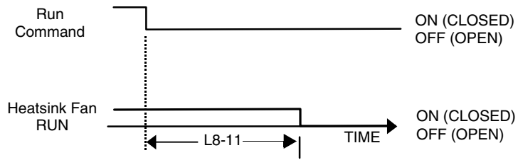
Fig. 84 Heatsink Cooling Fan Operation Timing Diagram
