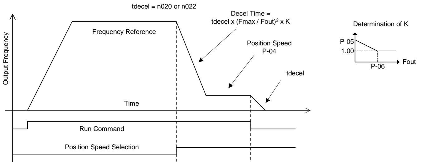
Figure 3: Operation When P-02 = 1 (Position Speed Mode Enabled)
