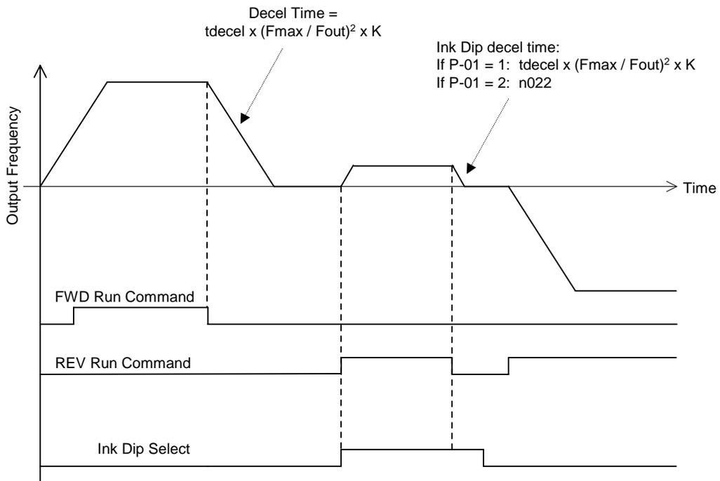
Figure 4: Operation of Ink Dip Mode
