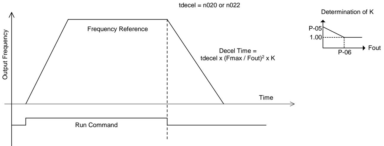
Figure 2: Operation When P-02 = 0 (Position Speed Mode Disabled)
