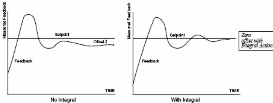
**Figure 137 PI Feedback Response Characteristics**
