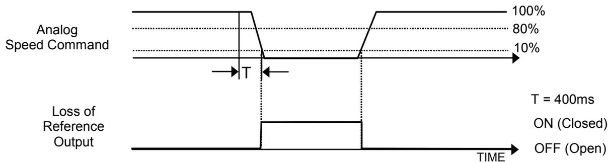
**Figure 56 Loss of Reference Function Characteristics**
