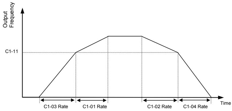
**Figure 24 Accel/Decel Switch Frequency Operation**
