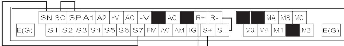
**Figure 85 Communication Terminal Connection for Self -Diagnosis Function**
