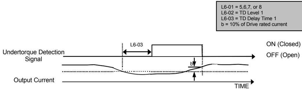
**Figure 55 Trq Det 1 N.O. Timing Diagram**
