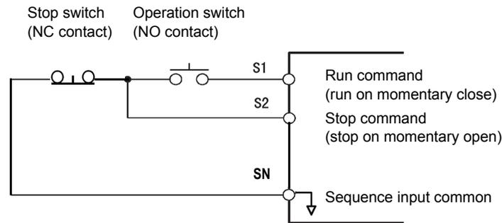
**Figure 32 Terminal Configuration for 3-Wire Control**
