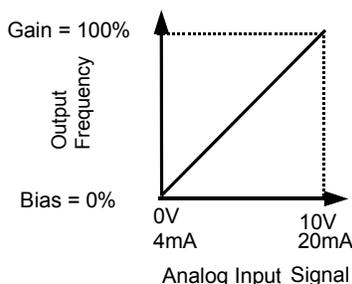
**Figure 61 Output Frequency as Commanded Via Analog Input**
