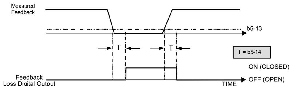
**Figure 23 Loss of PI Feedback Feature**
