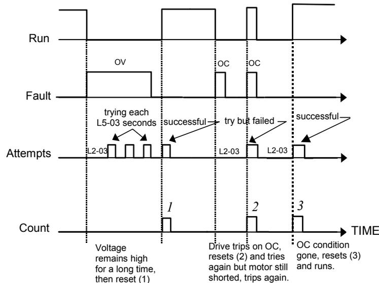
**Figure 95 Automatic Restart Timing Diagram**
