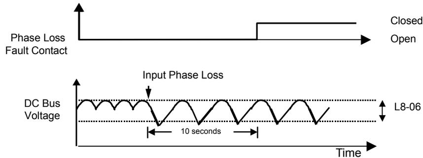
Figure 98 Input Phase Loss Detection Diagram
