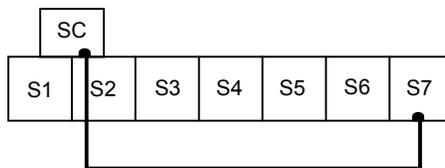
2. Wire the R+ and S+ terminals of the RS-485/422 port together
