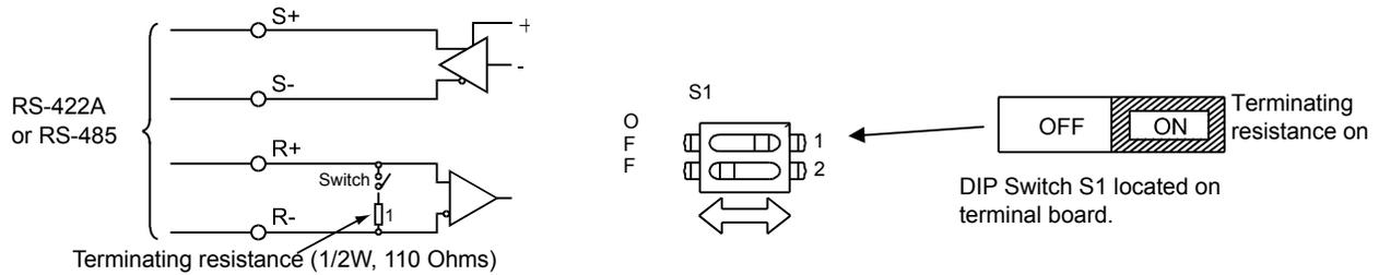
**Figure 77 Communication Connection Terminals and Terminating Resistance**
