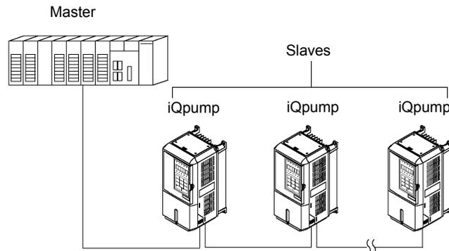
Figure 76 Example of Connections between Master and Drive
