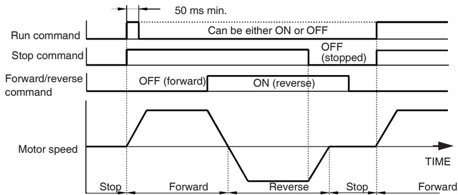
**Figure 33 3-Wire Control Timing Diagram**
