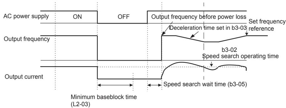
**Figure 19 Speed Search (Current Detection Method) after momentary power loss where the power loss time exceeds the minimum baseblock time**
