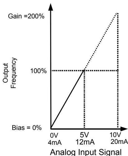
**Figure 62 Output Frequency as Commanded via Analog Input with Increased Gain Setting**
