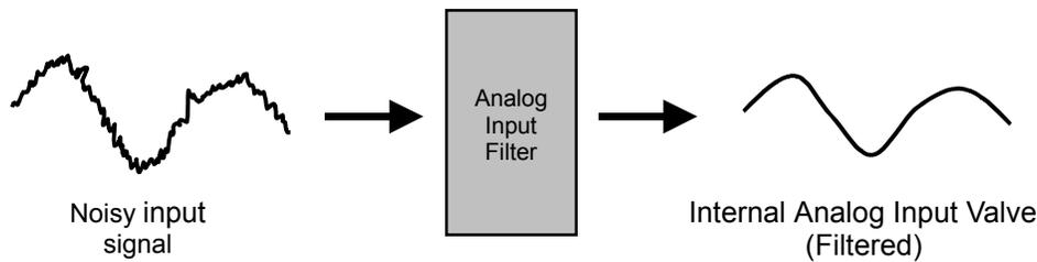
Figure 72 Analog Input Filter Time Constant Effect on “Noisy” Signal
