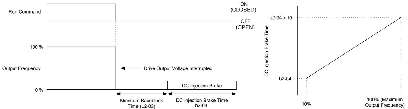
**Figure 11 DC Injection Braking to Stop**
