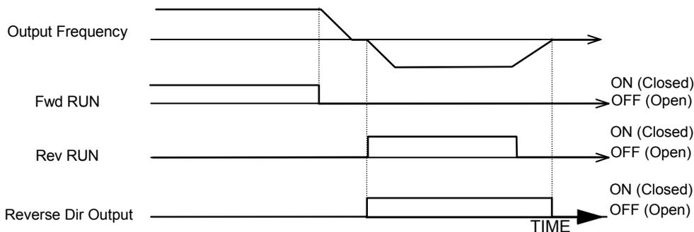
**Figure 58 Reverse Direction Timing Diagram**
