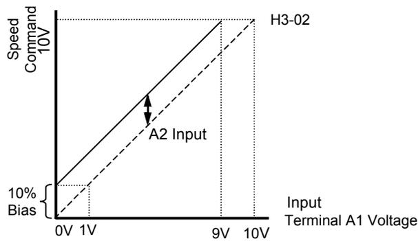
**Figure 66 Effect of Frequency Bias Function on Speed Command**
