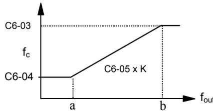
**Figure 27 Synchronous Carrier Frequency Characteristics**
