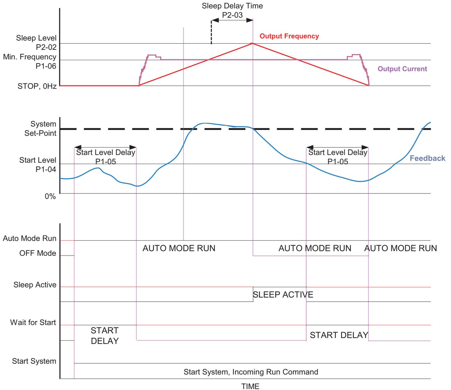
**Figure 105 Sleep Function Based on Output Current**
