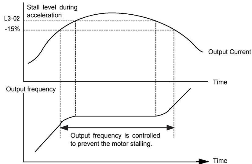
**Figure 90 Detailed Time Chart for Stall Prevention During Acceleration**
