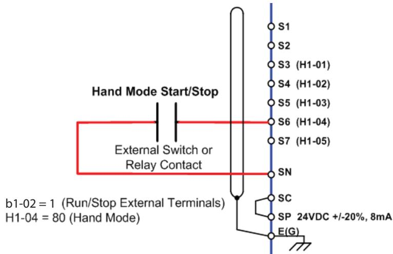
**Figure 42 Connection Diagram for External Hand Mode Contact (b1-02 = 1)**
