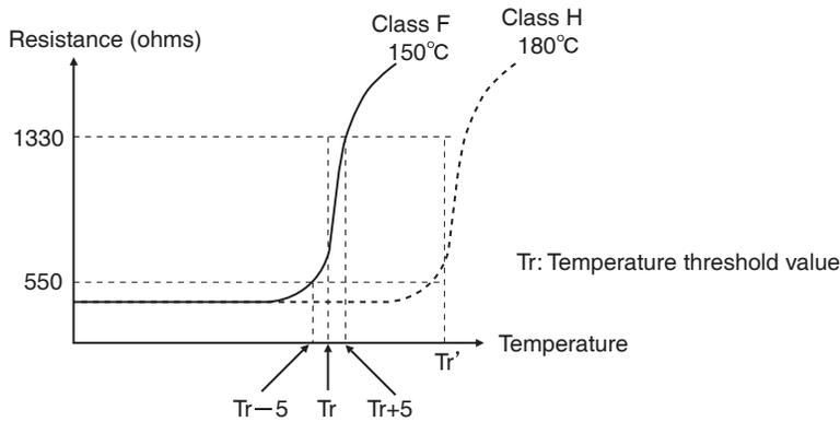
**Figure 89 PTC Thermistor Temperature-Resistance Value Characteristics**
