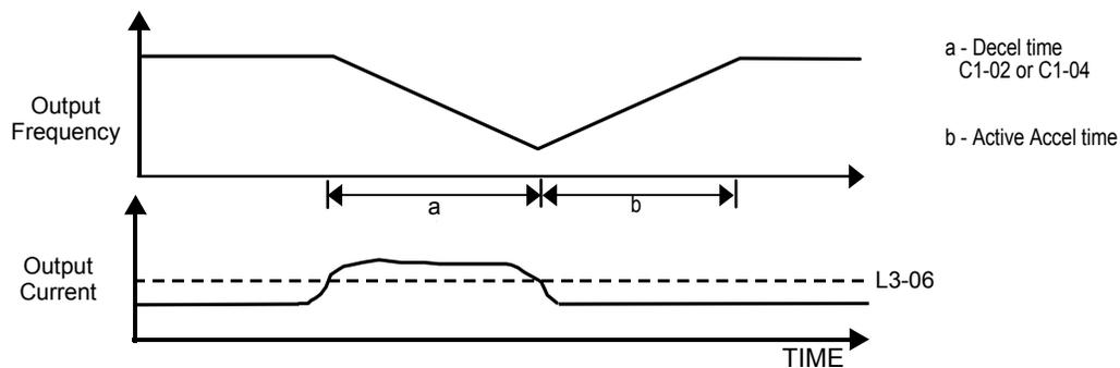
**Figure 93 Time Chart for Stall Prevention Level During Running**
