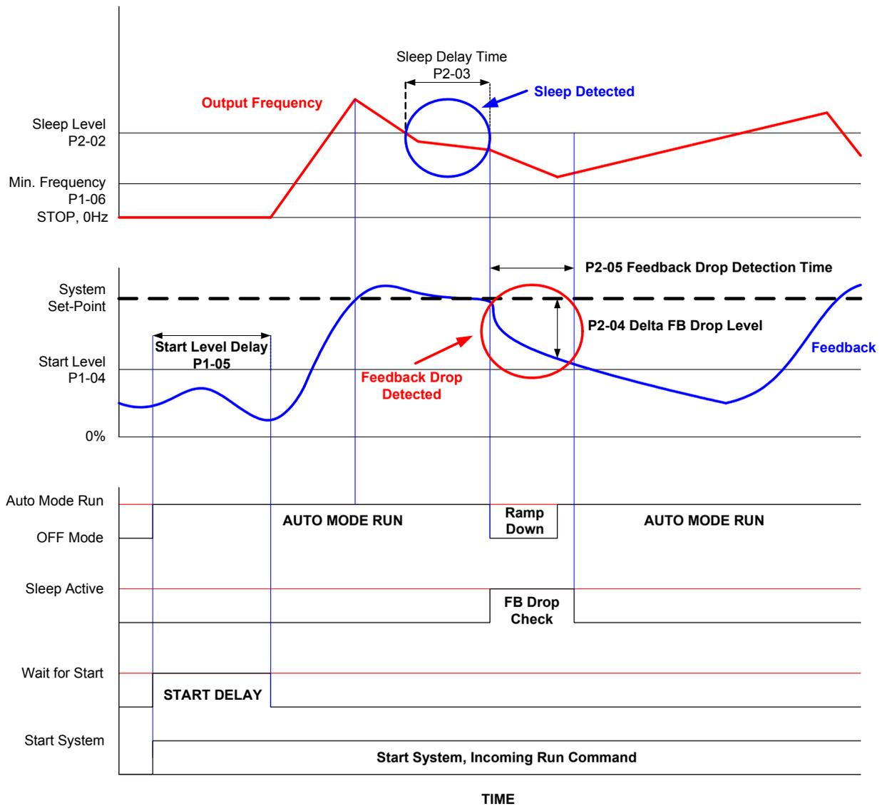
**Figure 107 No-Flow Detection During Deceleration**
