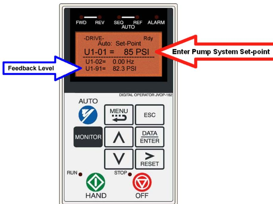
Figure 2 Digital Operator Auto Setpoint
