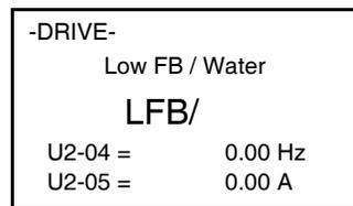
**Figure 48 Lower Water Fault on Operator**
