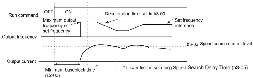
**Figure 17 Speed Search (Current Detection Method) at Startup**
