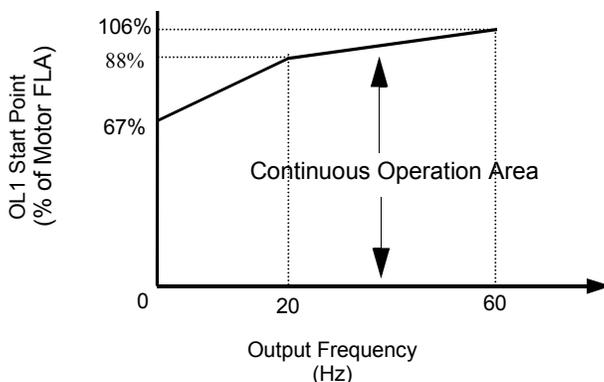
**Figure 86 Motor Overload Protection Curve**
