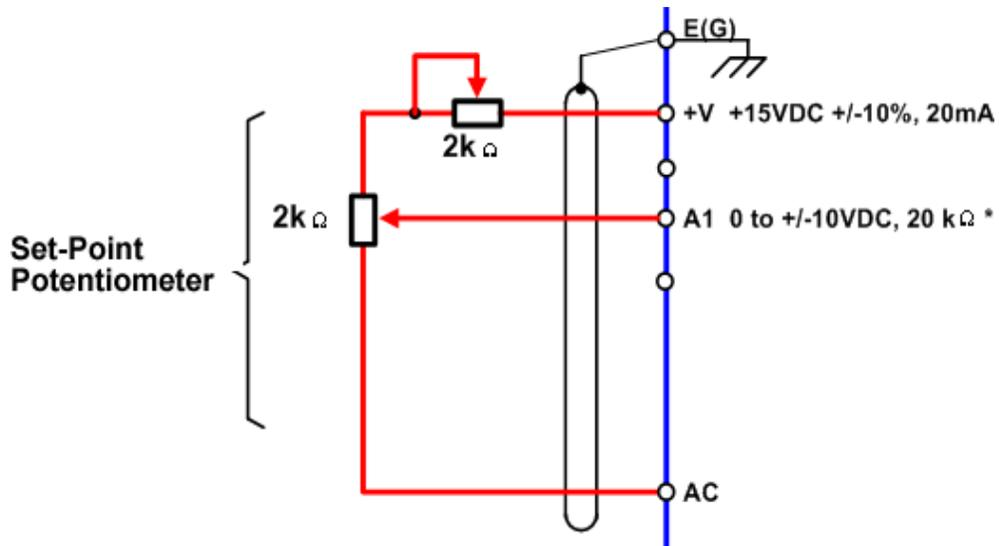
**Figure 3 Setpoint Potentiometer Connection Diagram**
