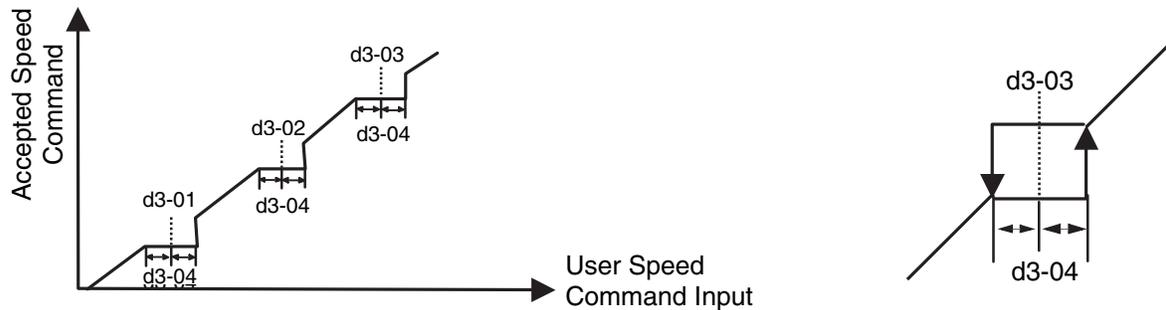
**Figure 30 Jump Frequency Characteristics**
