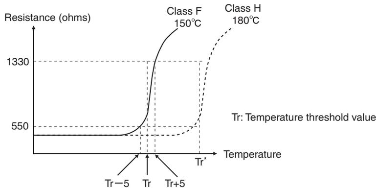
**Figure 69 PTC Thermistor Temperature-Resistance Value Characteristics**
