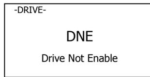
If a Run command is closed prior to the iQpump drive Enable input being closed the iQpump drive will not run until the Run command is cycled.
