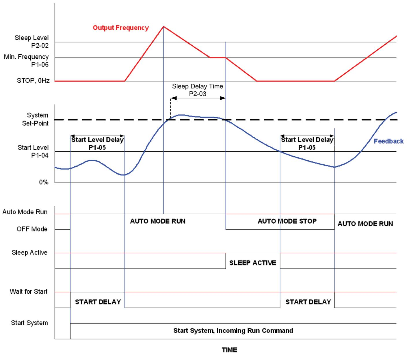
Figure 106 Sleep Function Based on Feedback Level
