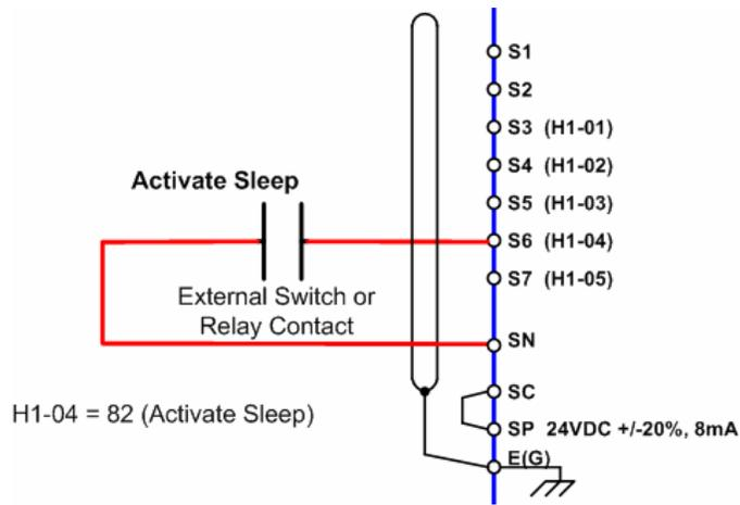
Figure 44 Wiring Diagram
