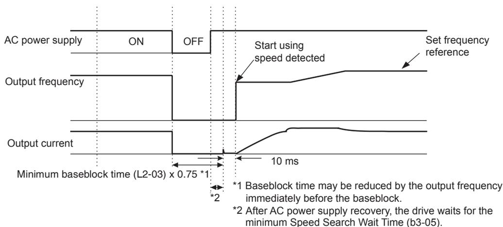
**Figure 15 Speed Search (Estimated Speed Method) after momentary power loss where the power loss time is less than the minimum baseblock time**
