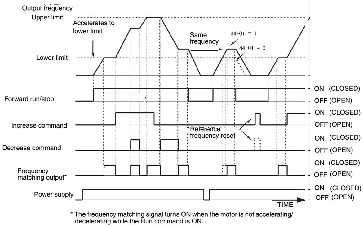
**Figure 37 Floating Point Control Time Chart**
