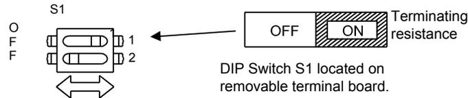
**Figure 41 DIP Switch Setting for Terminating Resistor**
