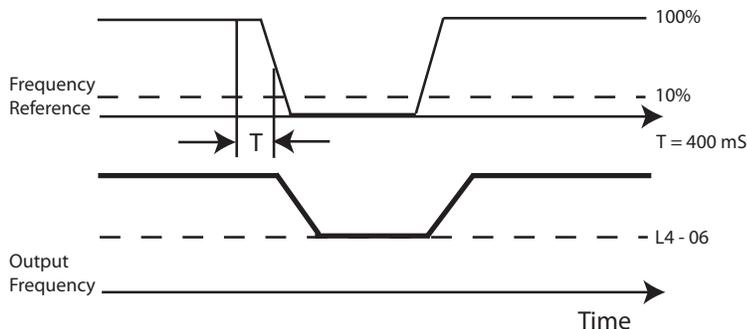
**Figure 94 Loss of Frequency Reference Timing Diagram**
