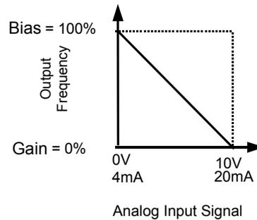
**Figure 64 Output Frequency with Inverted Gain and Bias Settings**
