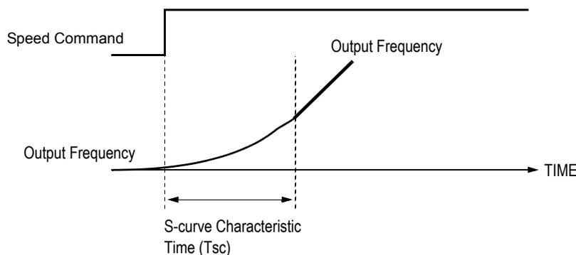
**Figure 25 S-curve Characteristic Timing Diagram**
