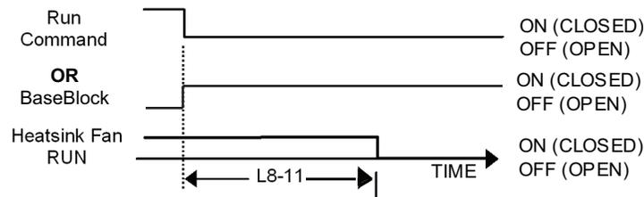
**Figure 99 Heatsink Cooling Fan Operation Timing Diagram**
