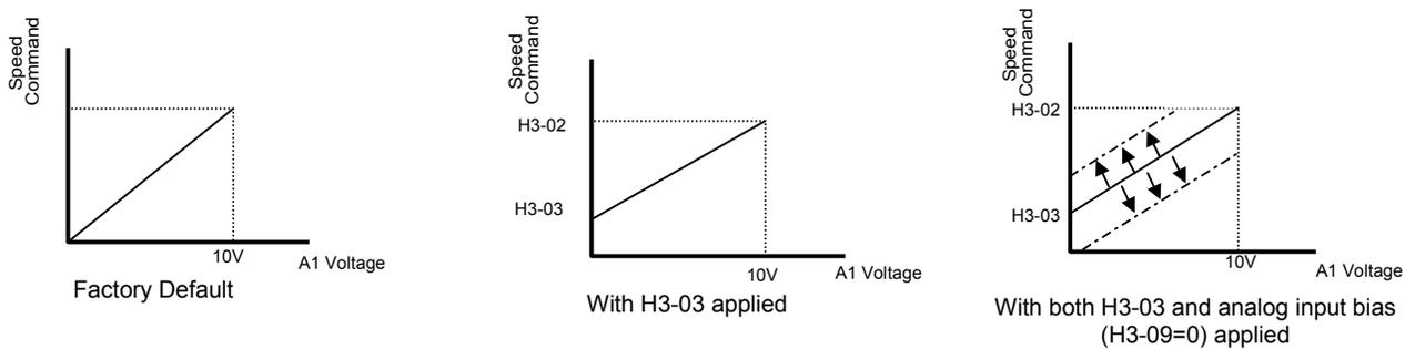
**Figure 67 Frequency Bias Applied to Analog Speed Command**
