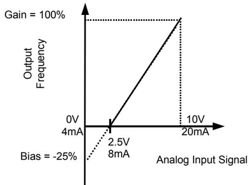
**Figure 63 Output Frequency with Reduced Bias Setting**
