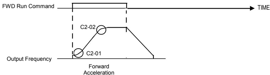
**Figure 26 S-Curve Characteristic Timing Diagram**
