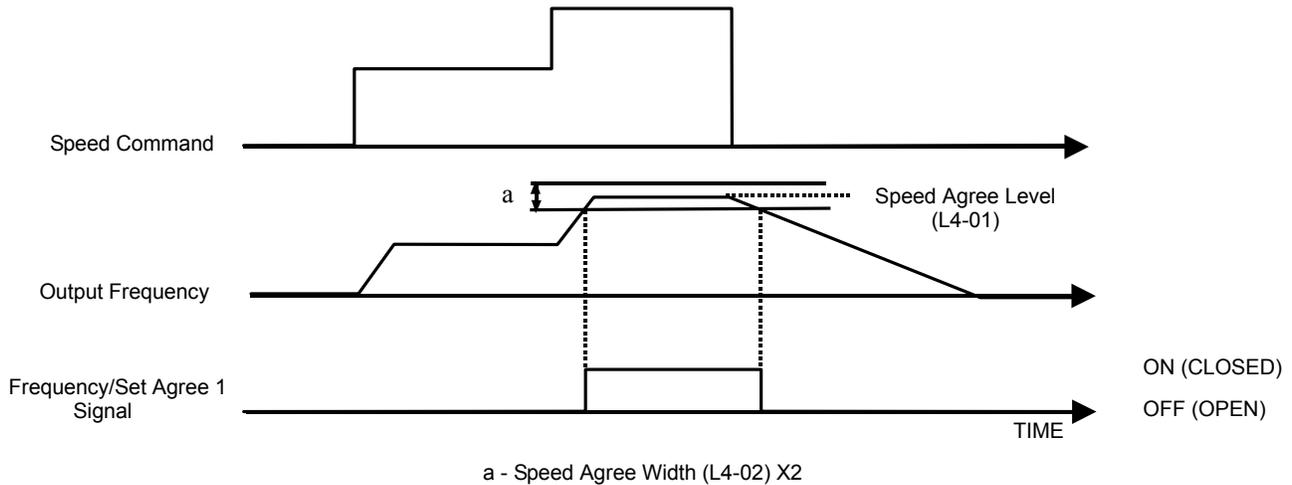
**Figure 52 Fref/Set Agree 1 Timing Diagram**
