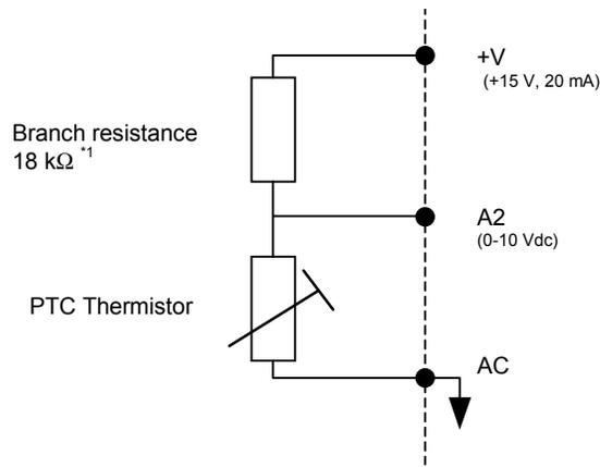
\*1 The resistance value of 18 kΩ is only valid for using a 3-phase PTC with the characteristics shown in the figure on following page.
