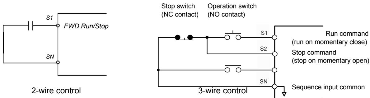
Figure 1 2 & 3-Wire Control Wiring Examples
