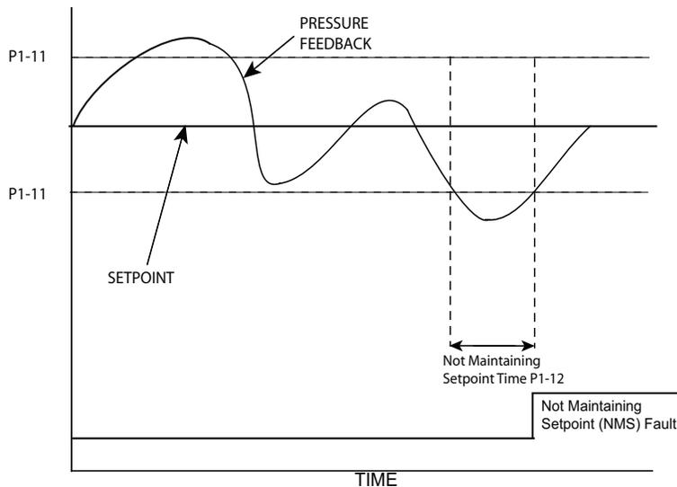
Figure 102 Not Maintaining Setpoint (NMS) Fault
