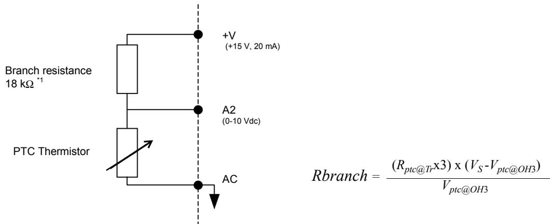
\*1 The resistance value of 18 kΩ is only valid for using a 3-phase PTC with the characteristics shown in the figure above.
