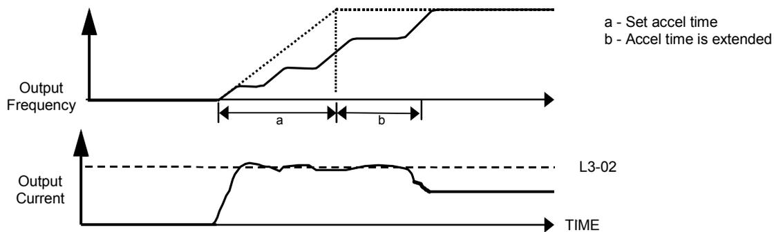
**Figure 91 Time Chart for Stall Prevention During Acceleration**
