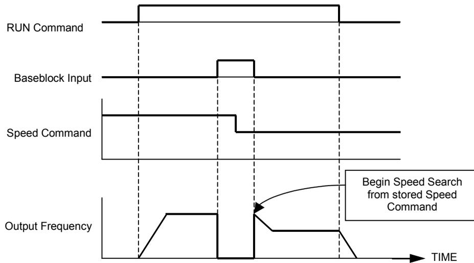
**Figure 35 External Baseblock Characteristics**
