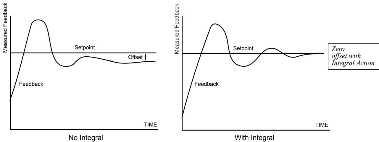
**Figure 22 PI Feedback Response Characteristics**
