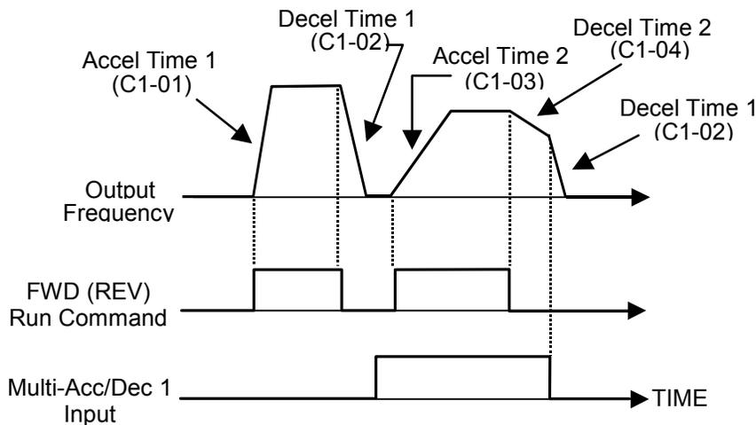
**Figure 34 Multi-Accel/Dec Timing Diagram**
