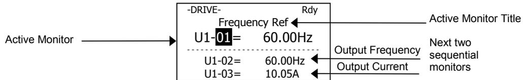
For example, if the iQpump drive needs to display the Elapsed Timer as the Power-On monitor, then o1-01 must be set to “13” and o1-02 must be set to “4”. The next time iQpump drive power is cycled, the digital operator displays U1-13 (Elapsed Time), U1-14 (Flash ID), and U1-15 (Term AI Level).
