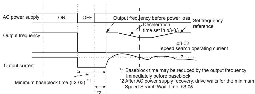
**Figure 18 Speed Search (Current Detection Method) after momentary power loss where the power loss time is less than the minimum baseblock time**
