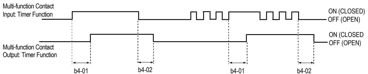
Figure 20 Timing Diagram of Timer Function
