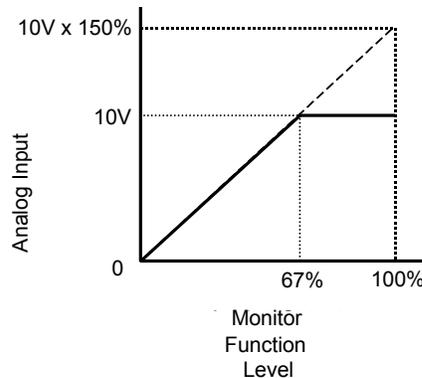
**Figure 74 Analog Output gain Setting Adjustment**
