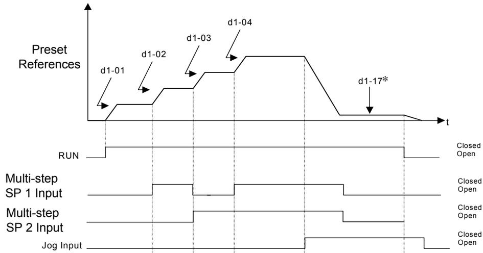
**Figure 28 Setpoint and Jog Reference Timing Diagram**
