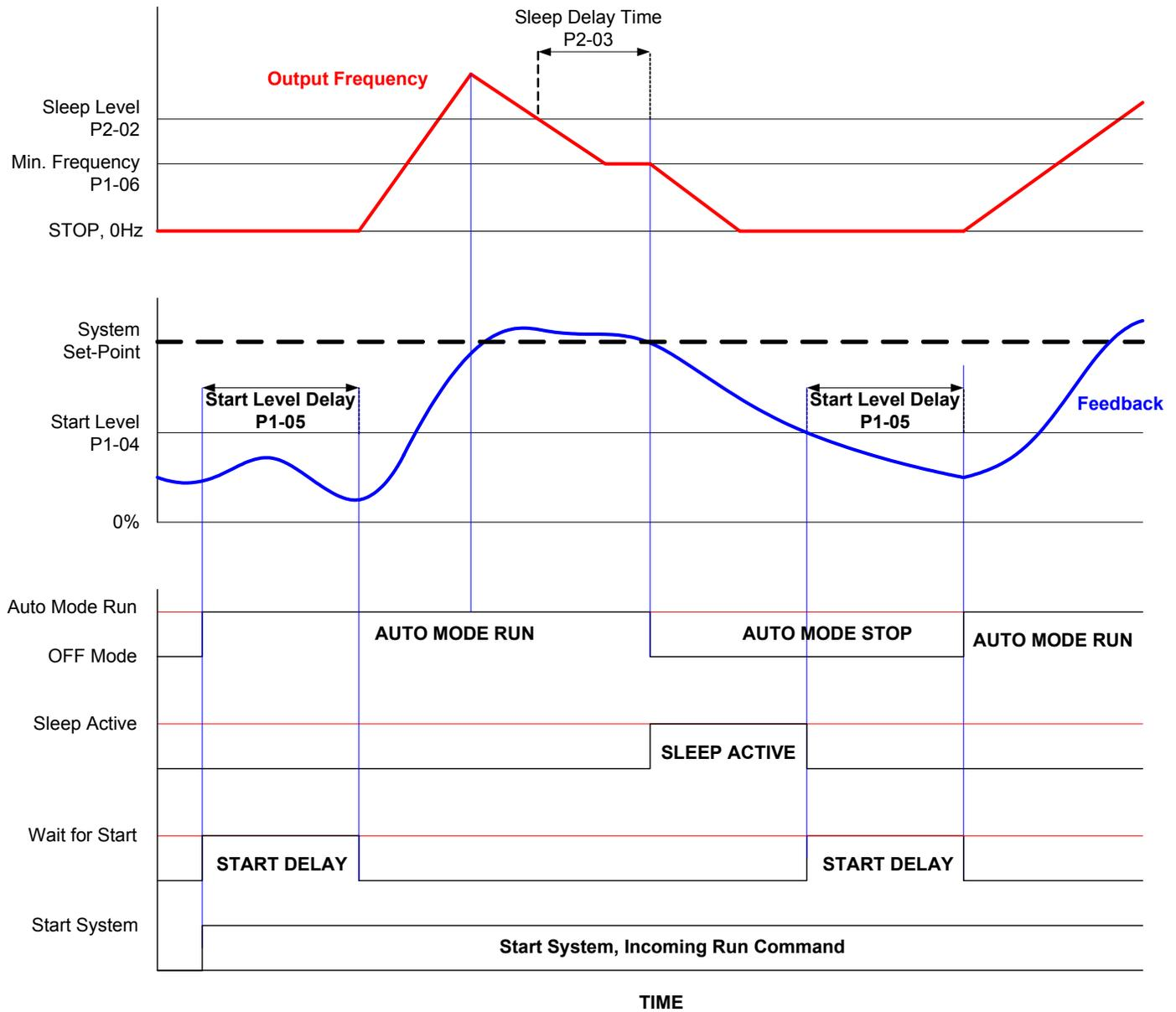
**Figure 104 Sleep Function Based on Output Frequency**
