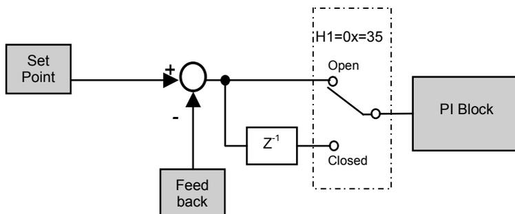
**Figure 40 PI Error signal Inversion Block Diagram**
