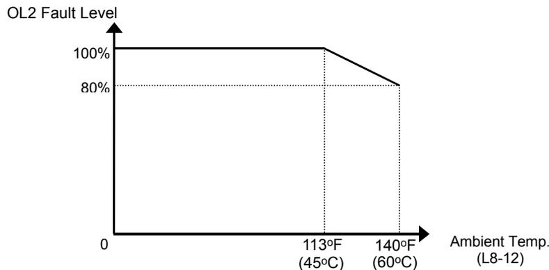
**Figure 100 Ambient Temperature Derating Curve**
