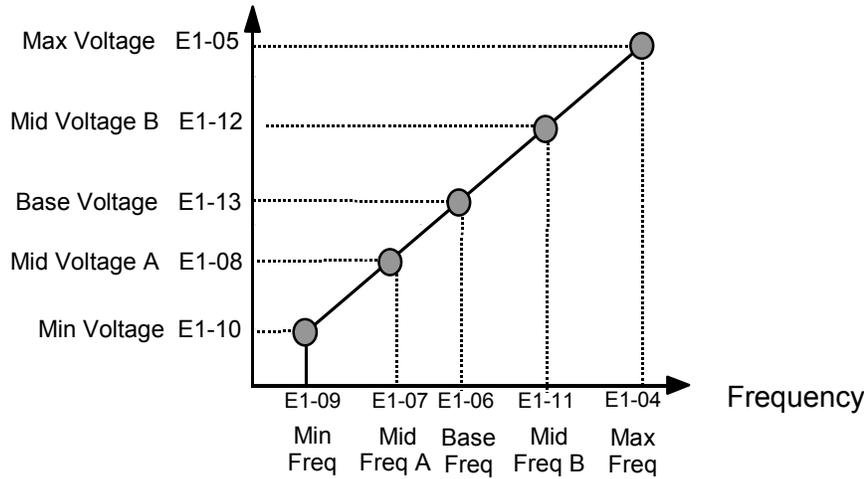
**Figure 31 Custom V/f Pattern Programming Curve**
