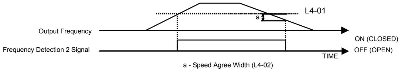
**Figure 54 Freq Detect 2 Timing Diagram**
