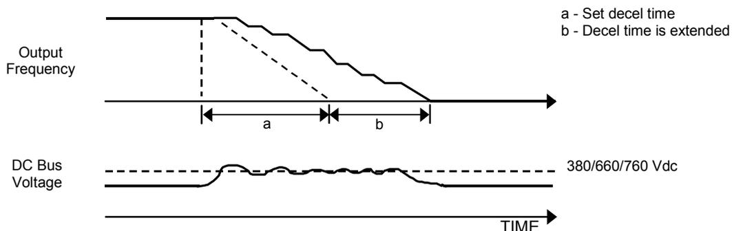
**Figure 92 Time Chart for Stall Prevention During Deceleration**
