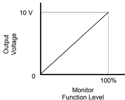
**Figure 73 Analog Output Signal Level as a Function of the Monitor Value**
