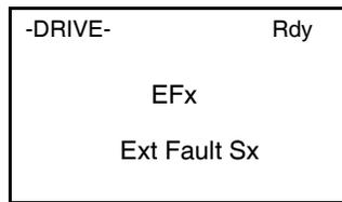
with the x in EFx and Sx represent the terminal number of the digital input that the fault was received on.
