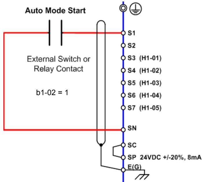
**Figure 6 Connection Diagram of External Start/Stop Switch**
