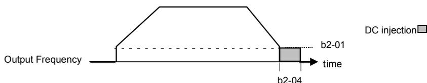
Figure 13 DC Injection Braking During Stopping
