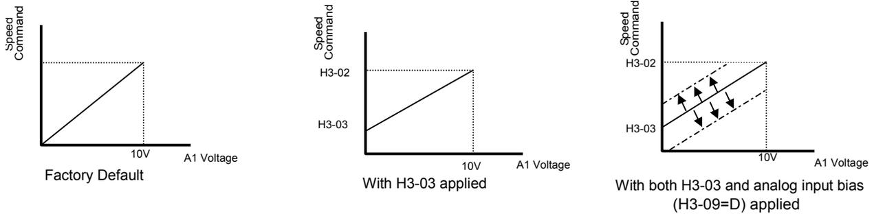
**Figure 68 Frequency Bias 2 Applied to Analog Speed Command**
