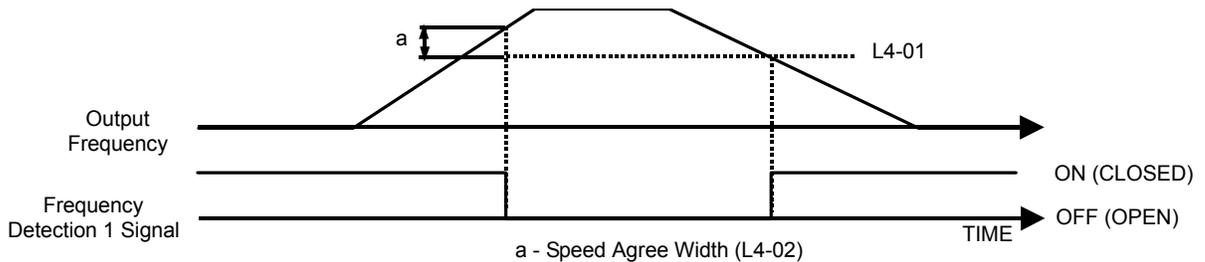
**Figure 53 Freq Detect 1 Timing Diagram**
