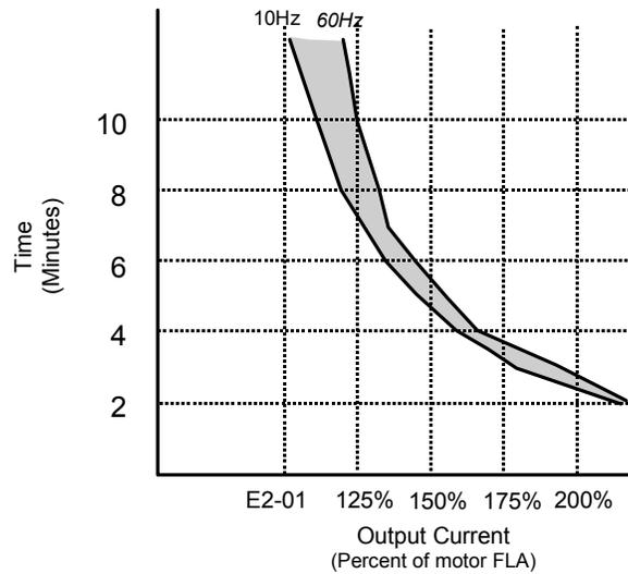
**Figure 87 Motor Overload Protection Time based on Output frequency and Load**
