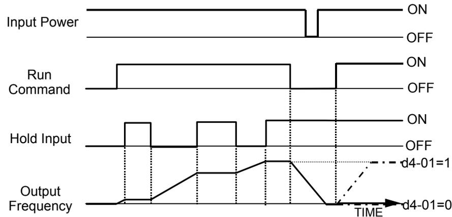
**Figure 36 Accel/Dec RampHold Function Timing Diagram**
