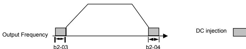
Figure 14 DC Injection Braking During Starting and Stopping
