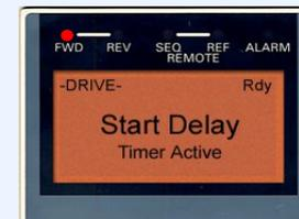
Displays when the iQpump is about to start. The feedback level has fallen below the Start Level (P1-04) and the start delay timer is active. Once the Start Level Delay Time (P1-05) expires the iQpump will start.
