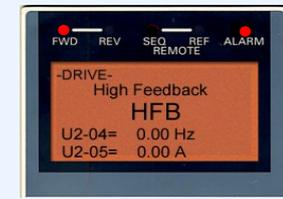
The feedback level has risen above P1-09 level for the time specified in P1-10. High feedback fault is active in Hand Mode, Auto Mode, Pre-Charge and Thrust Mode when the iQpump is running.
