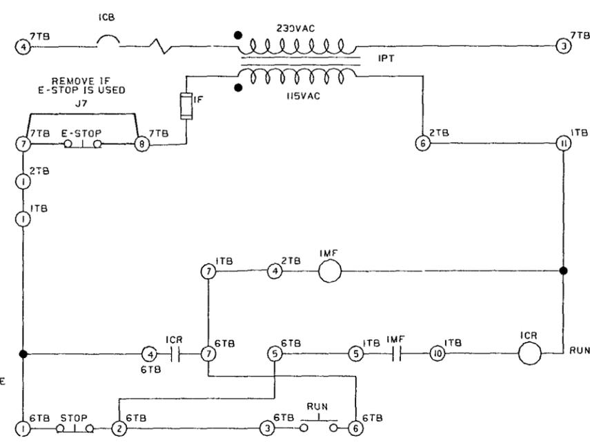
REVERSING ARMATURE FEEDBACK VOLTAGE REGULATOR WITH ANTI-PLUG, E-STOP
