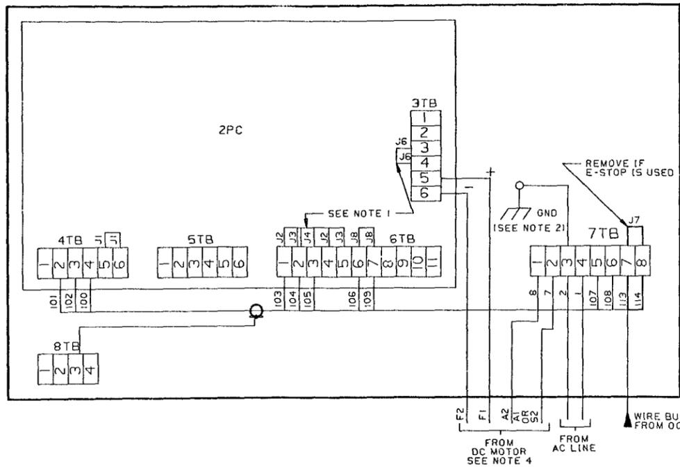
NON-REVERSING/ARMATURE VOLTAGE FEEDBACK REGULATOR WITH E-STOP
