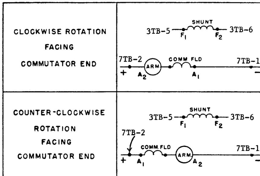
Figure 3-2. Shunt Motor
