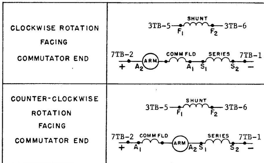
Figure 3-4. Compound Field Motor
