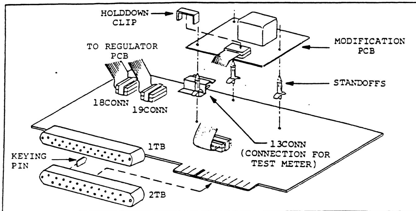
Figure 7-2. Mod Kit Installation on Relay/Interface PCB
