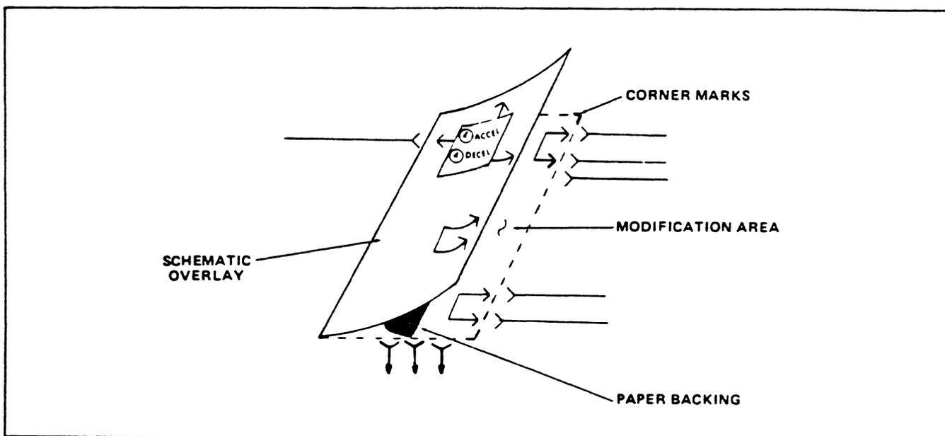
Figure 7-3. Application of Schematic Overlay
