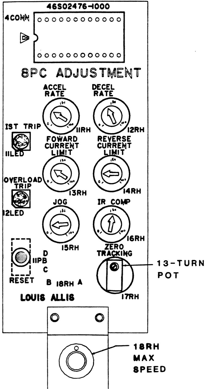
Figure 4-1. Location of Adjustment Controls
