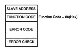
Figure 7. Response For Improper Command Message
