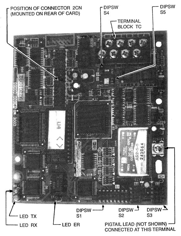
Figure 2. SCB Serial Communications Interface Card (shown larger than actual size)
