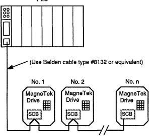
Figure 3. Serial Communication Data Link
