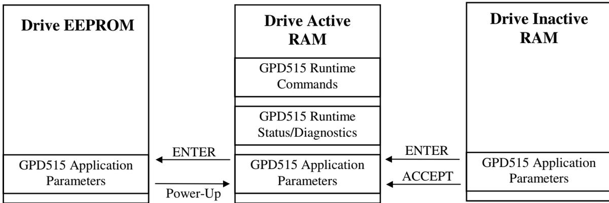
Some Parameter Data registers may be written to while the drive is running. These parameters are called run operative parameters. For a list of these parameters refer to Appendix A, Table A1-11 of the GPD 515 Technical Manual (TM 4515).
